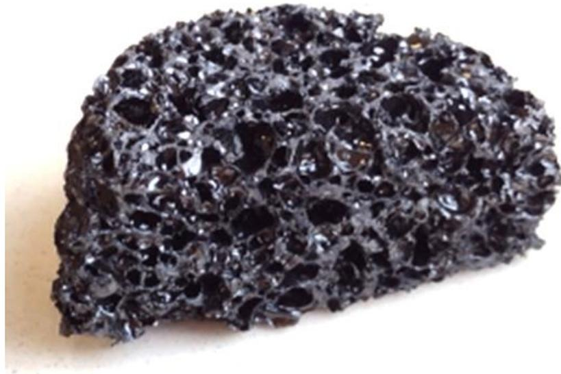
**Figure 3.** Coke recyclate used for the test specimens.
