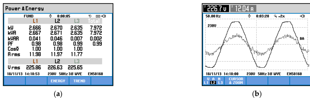
Figure 42. Case 5—ZSS and three-wire ShAPF operating with unbalanced loads: (a) source power; (b) voltage and current waveforms in phase S.
