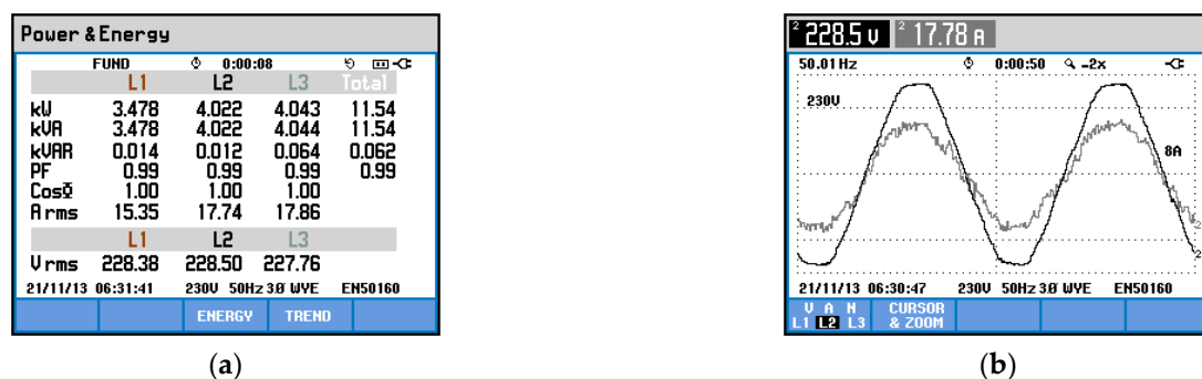
Figure 35. Case 3—four-wire ShAPF operating with balanced voltages and balanced loads: (a) source power; (b) voltage and current waveforms in phase S.
