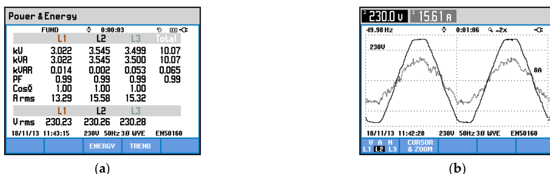
Figure 46. Case 6—four-wire ShAPF operating with unbalanced loads: (a) source power; (b) voltage and current waveforms in phase S.
