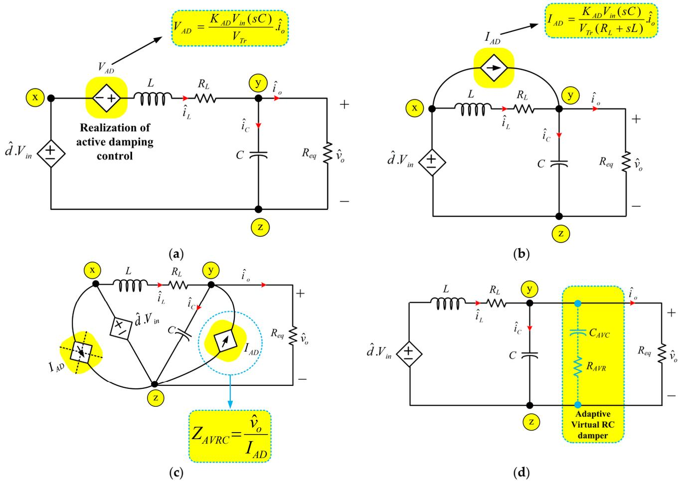
Figure 12. (a) Small-signal averaged model; (b) analytical interpretation of (a); (c) analytical represented in Figure 12b; (d) physical idea of AVRC damping [87].
