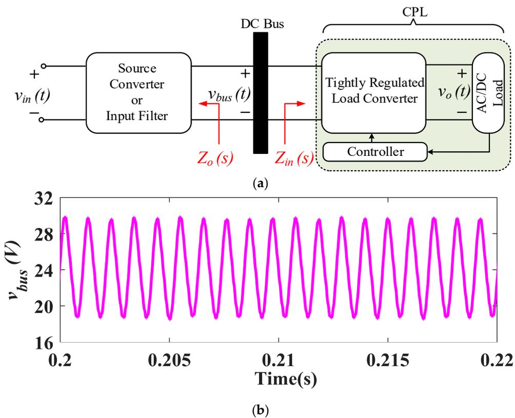
Figure 3. (a) A generic cascaded system feeding CPL. (b) Observed oscillation in DC bus voltage caused by CPL.
