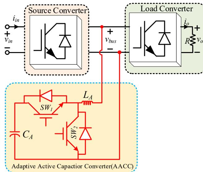
**Figure 16.** Intermediate-level active damping by adding an adaptive active capacitor converter (AACC) [103].
