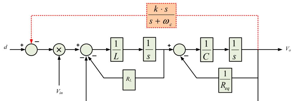
Figure 9. Block diagram representation of the buck converter with CPL [86].
