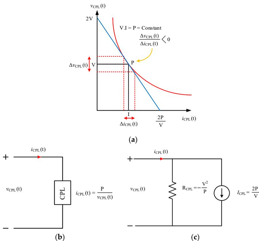
Figure 2. (a) Constant power load V-I Characteristics. (b) Large signal CPL model. (c) Small signal CPL model.
