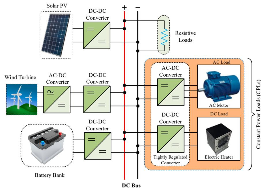
**Figure 1.** Architecture of DC Microgrid.
