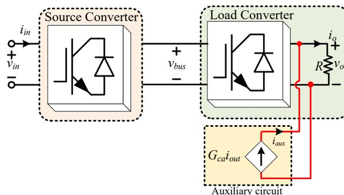
**Figure 17.** Using auxiliary circuit active damping [104].
