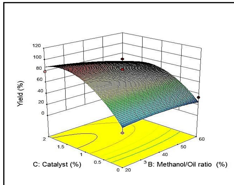
Figure 5. Biodiesel yield (%) vs. CC (%) and methanol/oil ratio (%).
