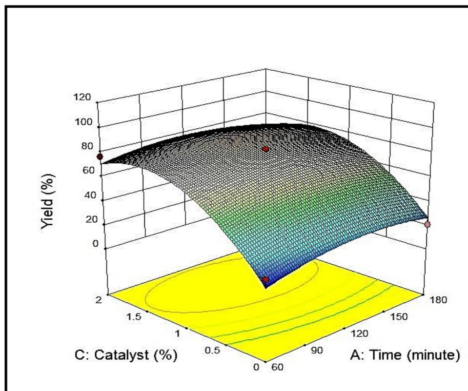
**Figure 6.** Biodiesel yield (%) vs. CC (%) and reaction time (minutes).
