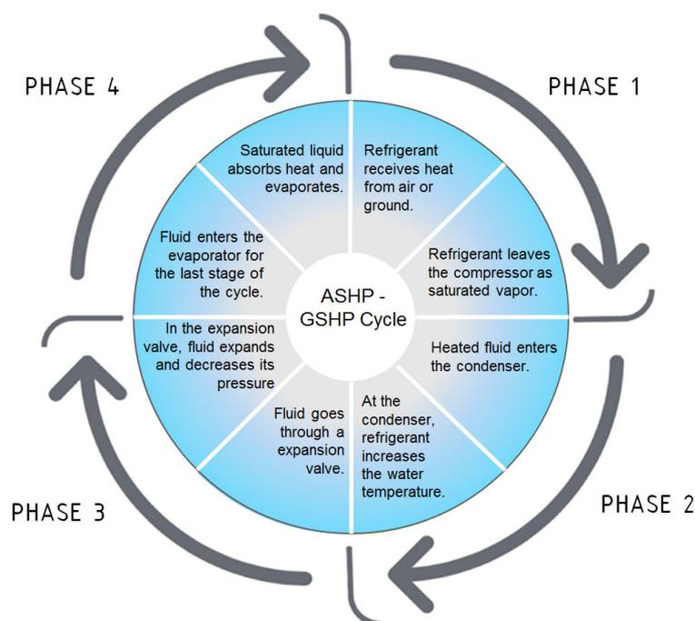
**Figure 2.** Schematic view of the ASHP and GSHP systems.
