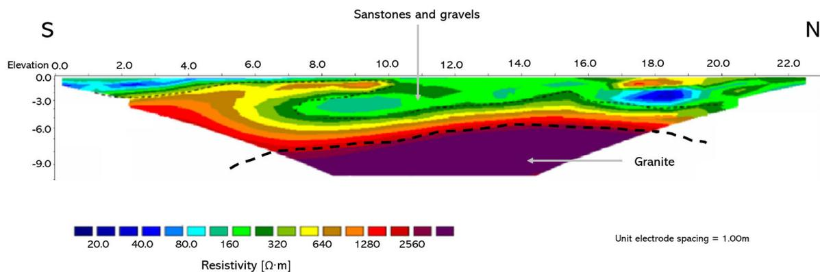
Figure 5. 2D electrical tomography profile for study Case 1, Ávila.
