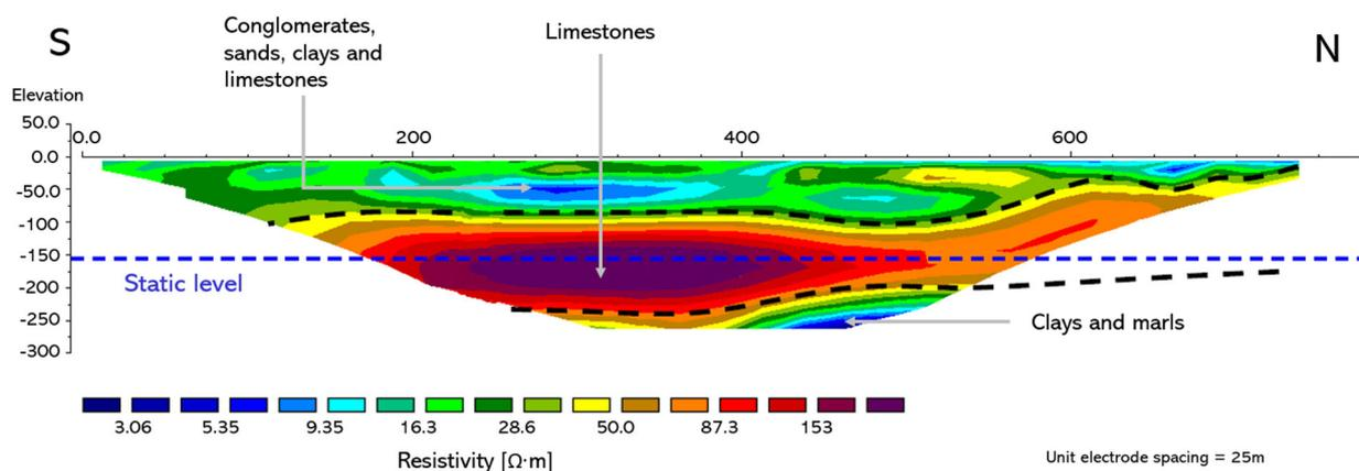
**Figure 6.** 2D electrical tomography profile for study Case 2, Alicante.
