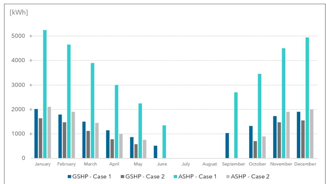
**Figure 7.** Monthly consumption of the different heat pumps alternatives in each Case.
