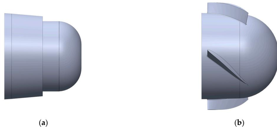
**Figure 8.** The original boss cap vs. the new boss cap with optimized fins. (a) Original boss cap. (b) New boss cap, with optimized PBCFs.
