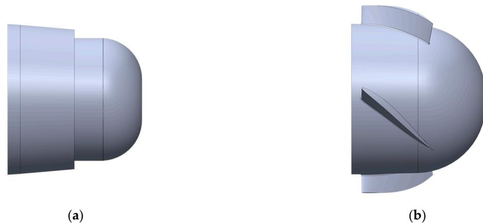
**Figure 8.** The original boss cap vs. the new boss cap with optimized fins. (a) Original boss cap. (b) New boss cap, with optimized PBCFs.
