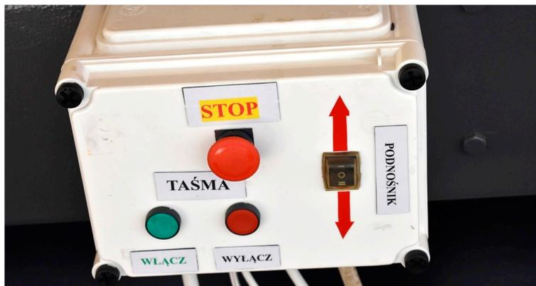
Figure 7. Local control of the belt feeder.
