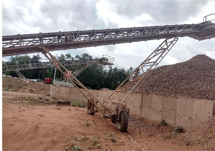
Figure 10. Belt feeder with VMSs (V-type mobile supports).
