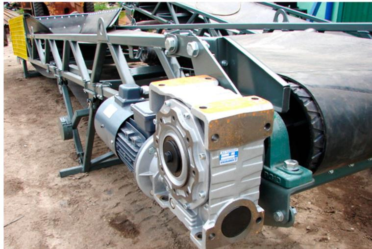
**Figure 2.** Belt feeder's drive (gear motor).
