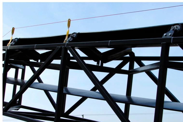
**Figure 4.** Belt feeder's route with idlers, trestles, and a safety line.
