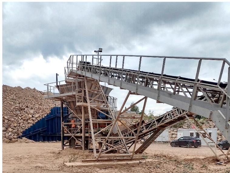
**Figure 9.** Belt feeder with VSSs (V-type stationary supports).
