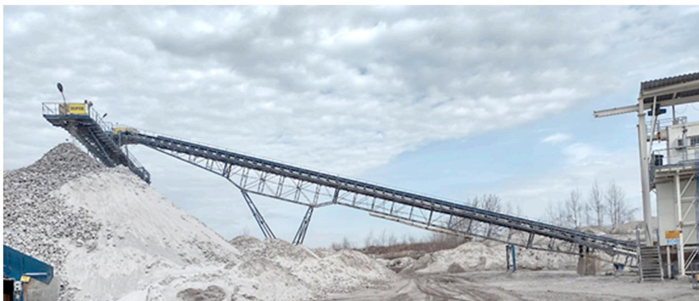
**Figure 1.** Belt feeder in the technological line of the processing plant of an aggregate mine.
