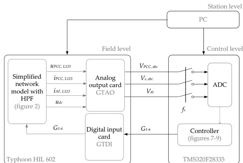
**Figure 17.** Scheme of hardware connections between control hardware and Typhoon HIL.
