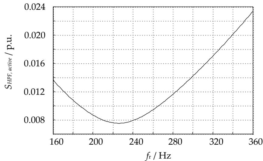
**Figure 3.** The required power of the active part of the hybrid filter as a function of the tuning frequency of the passive part [20]—case parameters (in p.u.):  $U_{supply,1} = 1$ ;  $I_{Load,1} = 1$ ;  $I_{Load,5} = 0.2$ ;  $I_{Load,7} = 0.14$ ;  $f_t = 200$  Hz.
