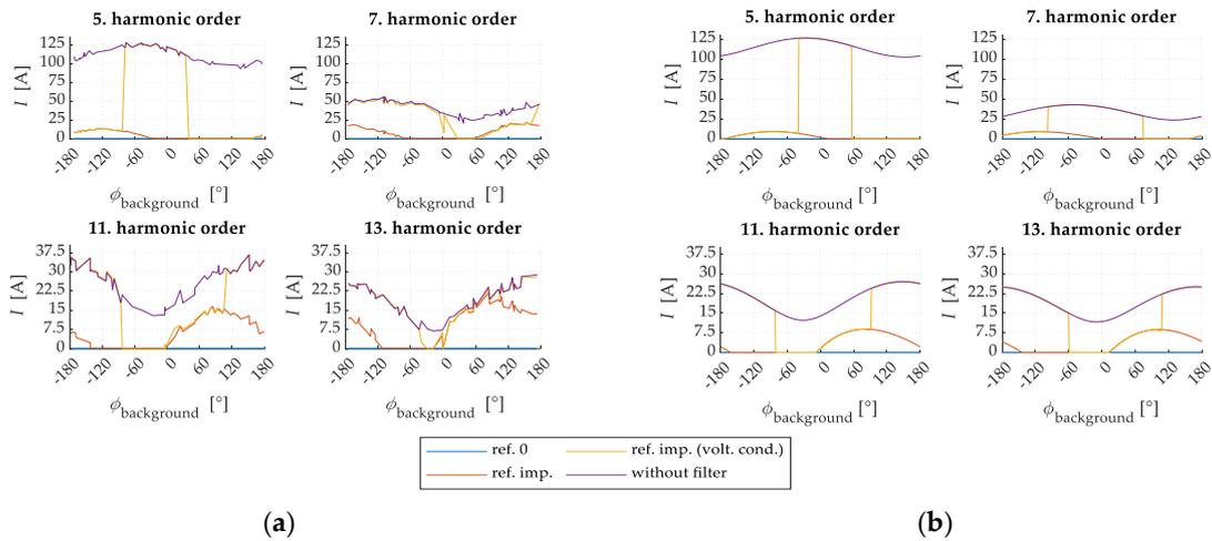
Figure 12. Measured system current (reference) at PCC: PSCAD results (a) vs. ideal harmonic sources analysis (b).
