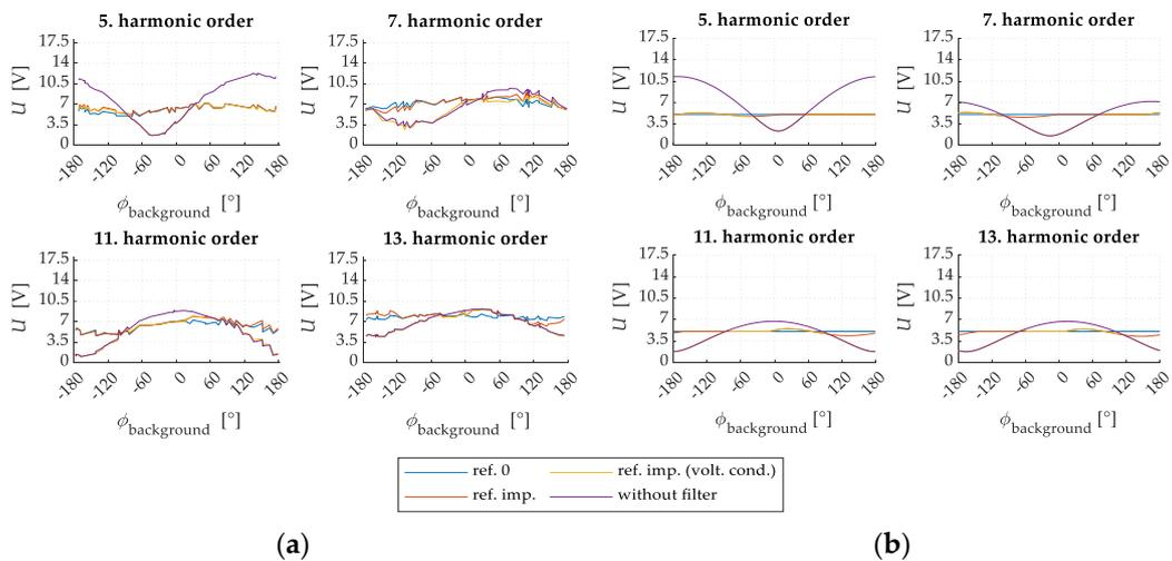
Figure 14. Measured harmonic voltage distortion at PCC: PSCAD results (a) compared to the ideal harmonic source analysis (b).
