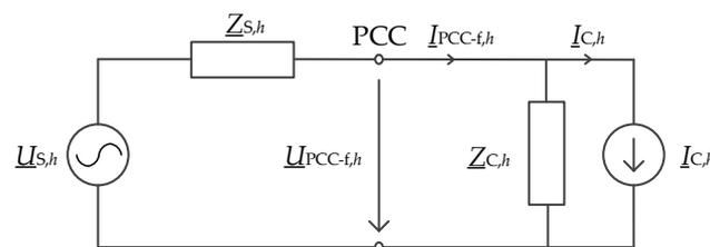
**Figure 5.** Equivalent network of the single-line model used for defining reference harmonic impedances, utilizing fictive voltages and currents.
