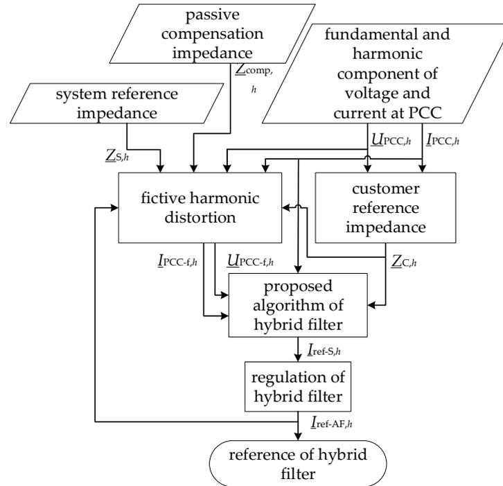
Figure 7. Flowchart for reference current calculation method.
