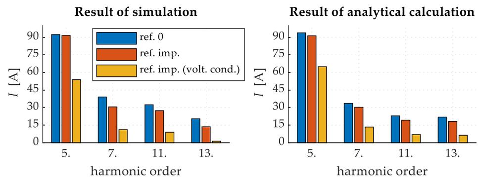
Figure 15. Comparison of the hybrid filter's average current.
