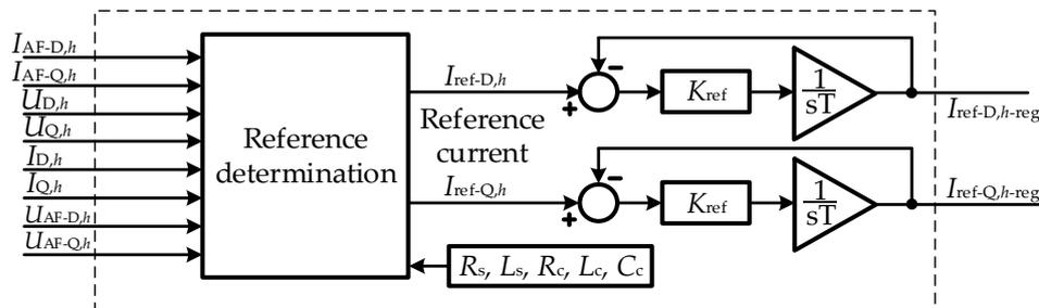
Figure 9. Block Diagram of the Reference Control Loop [34].
