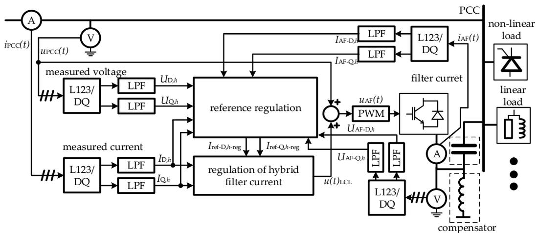
Figure 8. Control block diagram of the HPF.
