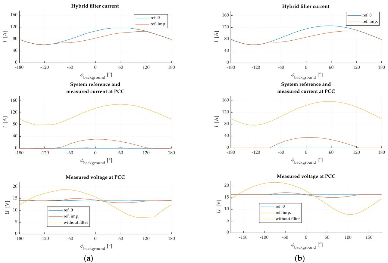
**Figure 18.** Result of CIL analysis with Typhoon HIL simulator (a) and ideal harmonic source (b).
