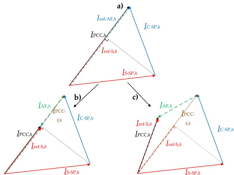
**Figure 6.** Phasor diagram: (a) before the HPF starts with the operation; (b) ideal case; (c) realistic case.
