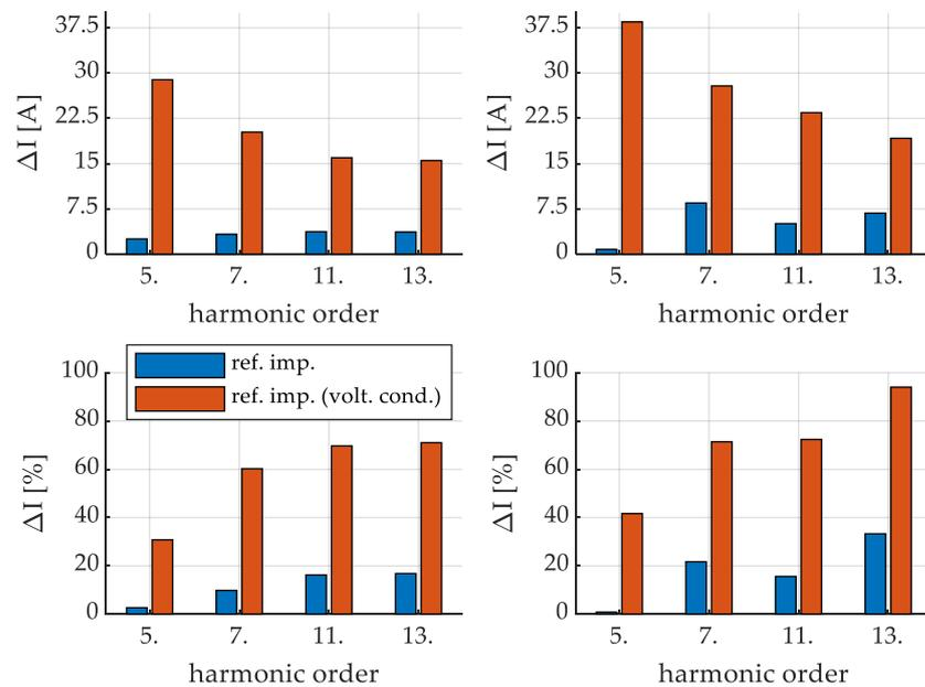
Figure 16. Differences in the average HPF current: simulation results (left) and analytical calculation (right).
