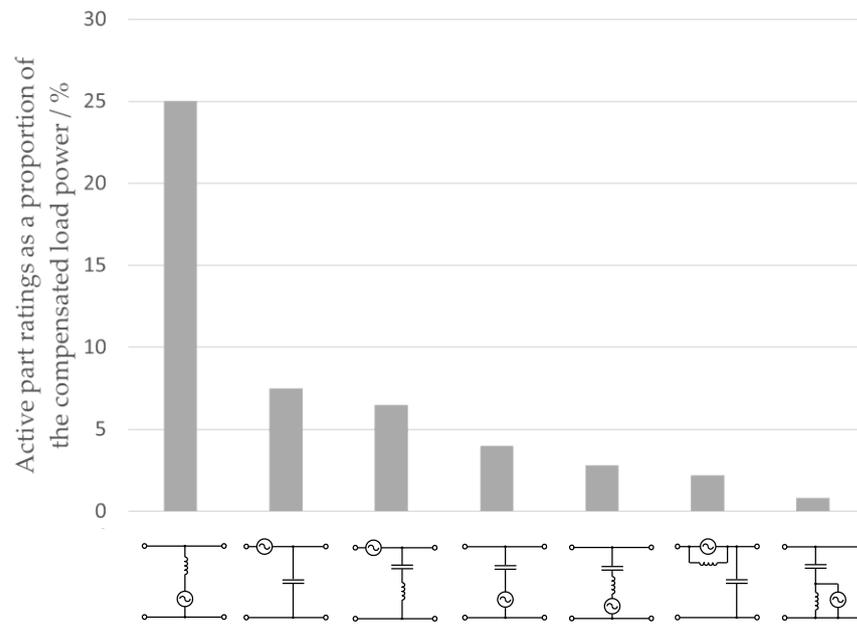
**Figure 4.** Representation of theoretically minimal required ratings of voltage converters for the most commonly used topologies [20]—case parameters (in p.u.):  $U_{supply,1} = 1$ ;  $I_{Load,1} = 1$ ;  $I_{Load,5} = 0.2$ ;  $I_{Load,7} = 0.14$ ;  $f_t = 200$  Hz.
