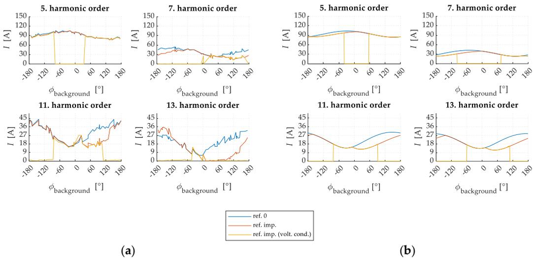
Figure 13. Hybrid filter current: PSCAD simulation (a) and analysis with ideal harmonic sources (b).
