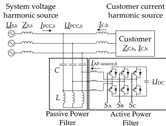
Figure 1. The diagram of the proposed topology of HPF.
