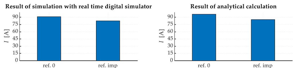
**Figure 19.** Comparison of the average current of the hybrid filter in the simulation.
