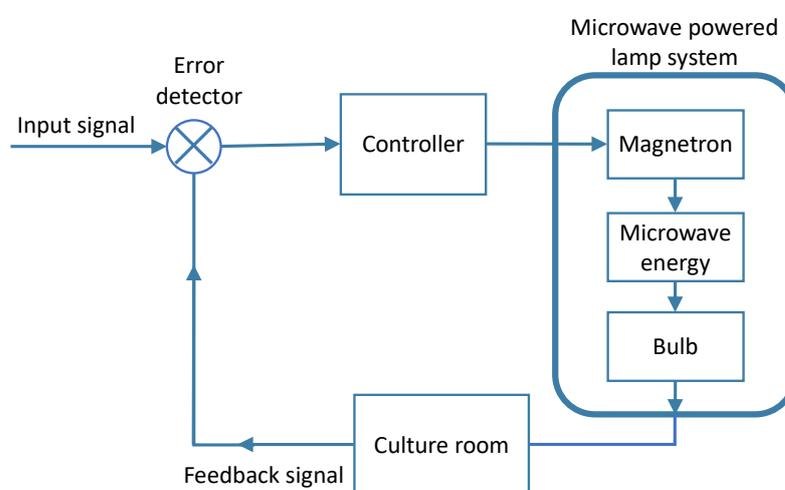
**Figure 5.** Experimental set-up and microwave-lamp schematic.
