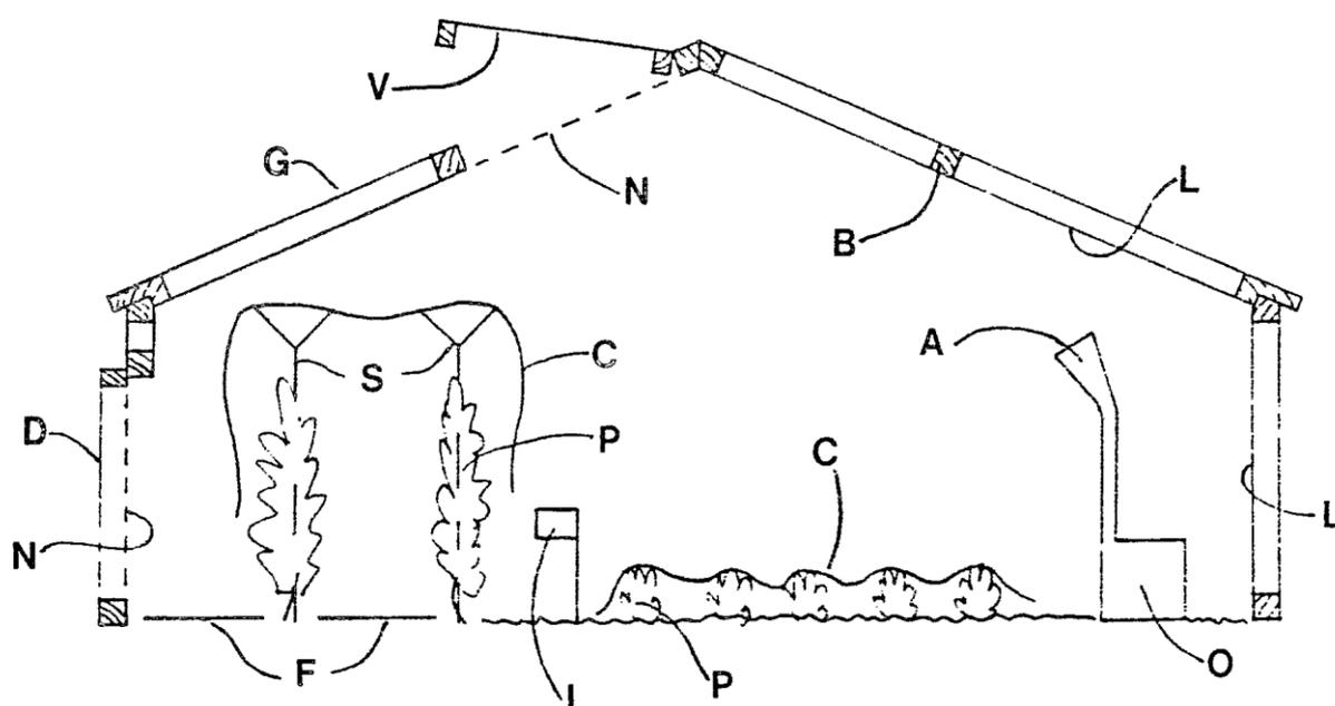
**Figure 3.** General system setup as proposed by Huber’s patent n° GB2120065A. Meaning of letters: “D” door, “O” magnetron oscillator, “A” horn antenna, “L” reflecting liner, “G” glazing, “B” glazing bars, “V” ventilators, “N” metal mesh, “F” metal foil, “P” plants to be heated, “C” film of thin, clear, polythene sheet, “S” plant supports, “I” infra-red detector.
