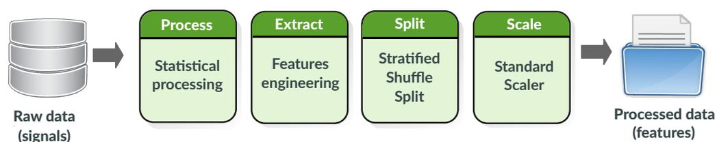
**Figure 1.** Data processing pipeline transforming the raw time-domain PMU signals into standardized training and test feature sets.
