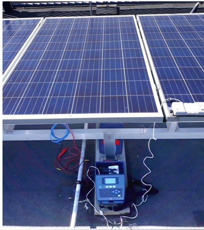
**Figure 4.** Stand for measuring I–V characteristics (photo by J. Teneta).
