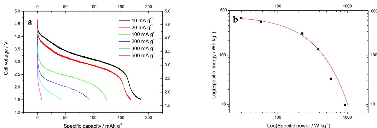
**Figure 7.** Voltage profiles recorded at various specific currents (a) and Ragone plot (b) for the material prepared by the sol-gel procedure. The specific current values are reported in the legend.
