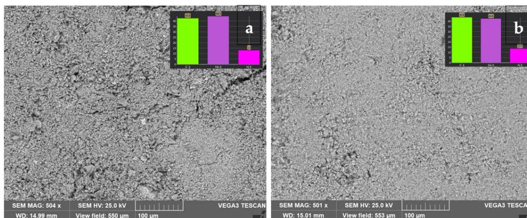
**Figure 3.** Low magnification BSE images (500×) of the material prepared by the solid-state synthesis method (a) and by the sol-gel procedure (b). The insets show the percentage composition of manganese (violet), nickel (pink), and oxygen (green) as evaluated by X-ray microanalysis.
