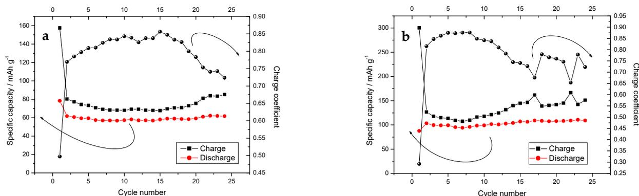
**Figure 6.** Specific capacity and charge coefficient as a function of the cycle number for the material prepared by the solid-state synthesis method (a) and by the sol-gel procedure (b).
