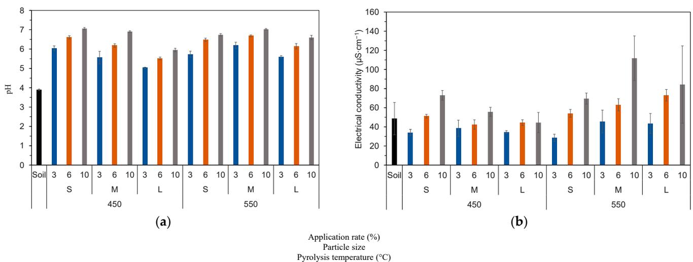
**Figure 3.** Values of (a) pH and (b) electrical conductivity for the treatment mixtures assorted by application rate (3%, 6%, and 10% ( $w/w$ ), which correspond to the blue, orange, and grey columns, respectively), particle size (S  $< 0.5$  mm, M = [0.5, 3.15], and L  $> 3.15$  mm), and pyrolysis temperatures, with the control soil as a reference (black column).
