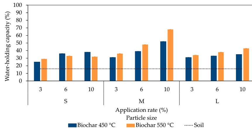
**Figure 2.** Water-holding capacity of biochar incubated in soil compared to the negative control (dotted line).
