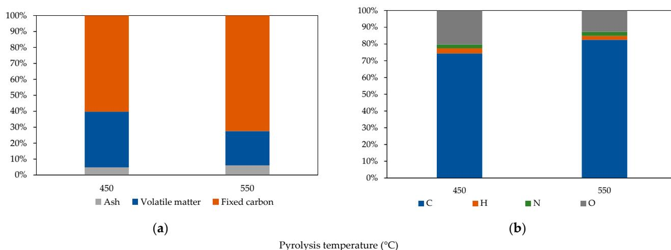
**Figure 1.** Values of the (a) proximate and (b) elemental analysis of biochar produced at 450 °C and 550 °C.
