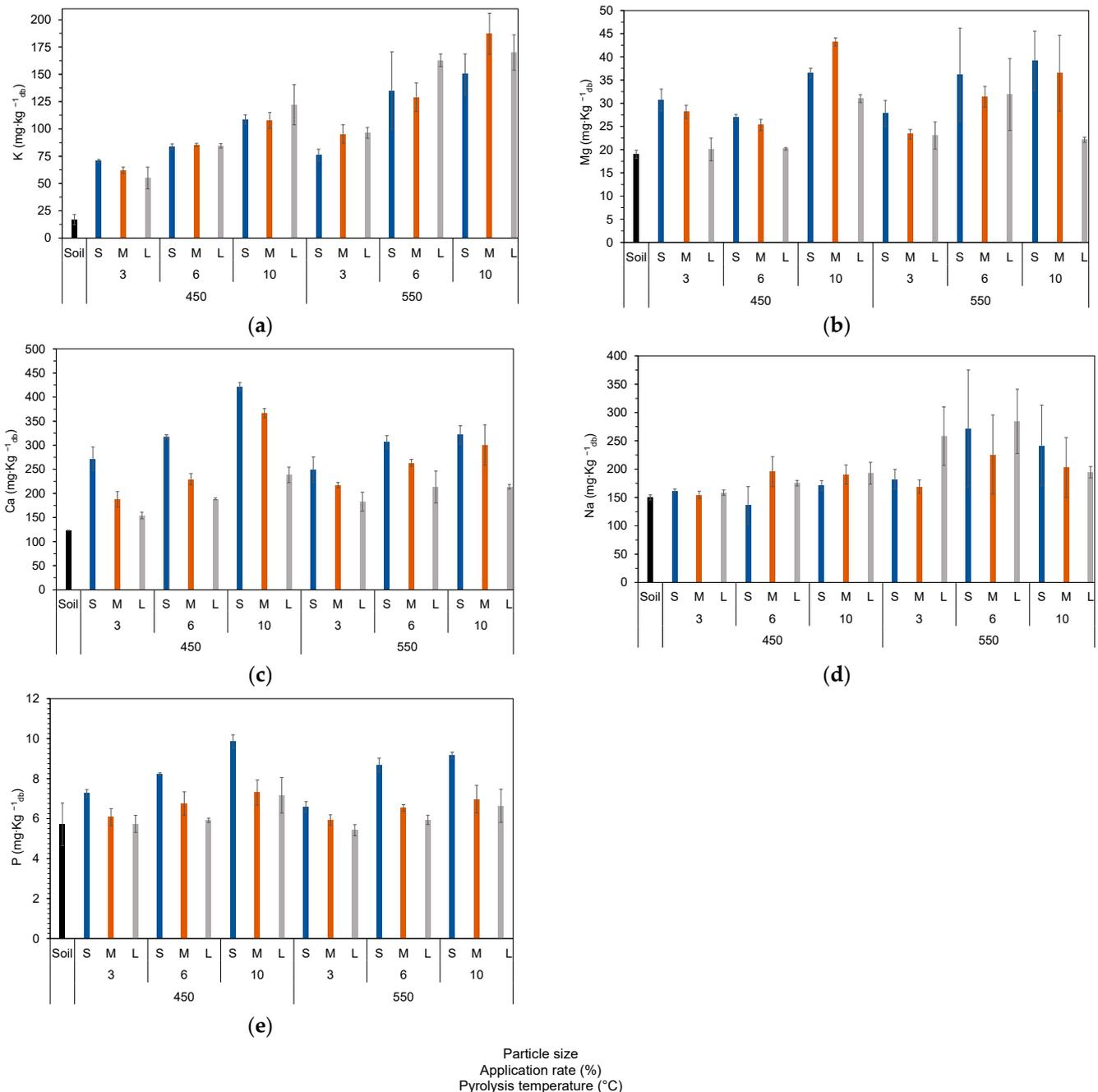
**Figure 4.** Plant nutrient element concentrations in the soil treatments assorted by particle size (S < 0.5 mm, M = [0.5, 3.15], and L > 3.15 mm, corresponding to the blue, orange, and grey columns, respectively); application rate; and pyrolysis temperatures: (a) K, (b) Mg (B), (c) Ca, (d) Na, and (e) P, with the control soil as a reference (black column).
