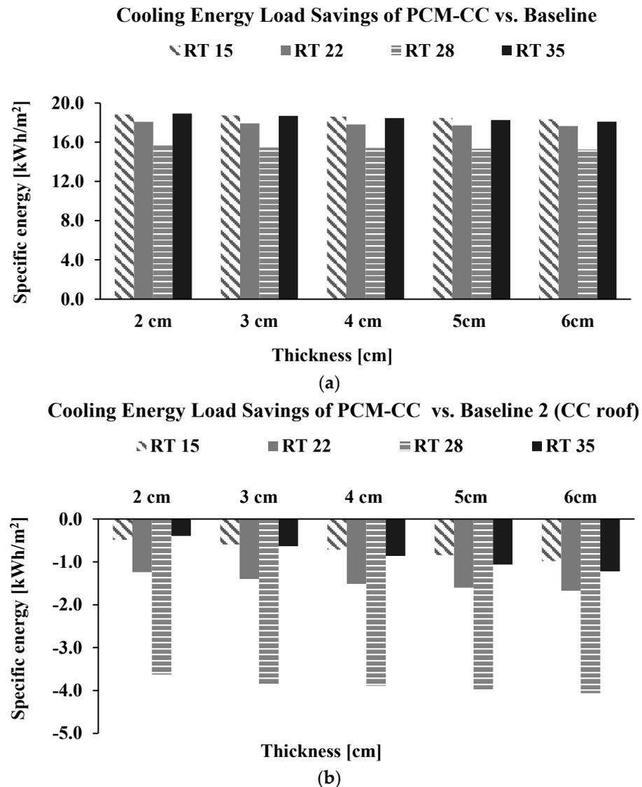
**Figure 4.** Cooling energy load savings of the PCM-CC roof system compared to (a) baseline scenario 1 and (b) baseline scenario 2.
