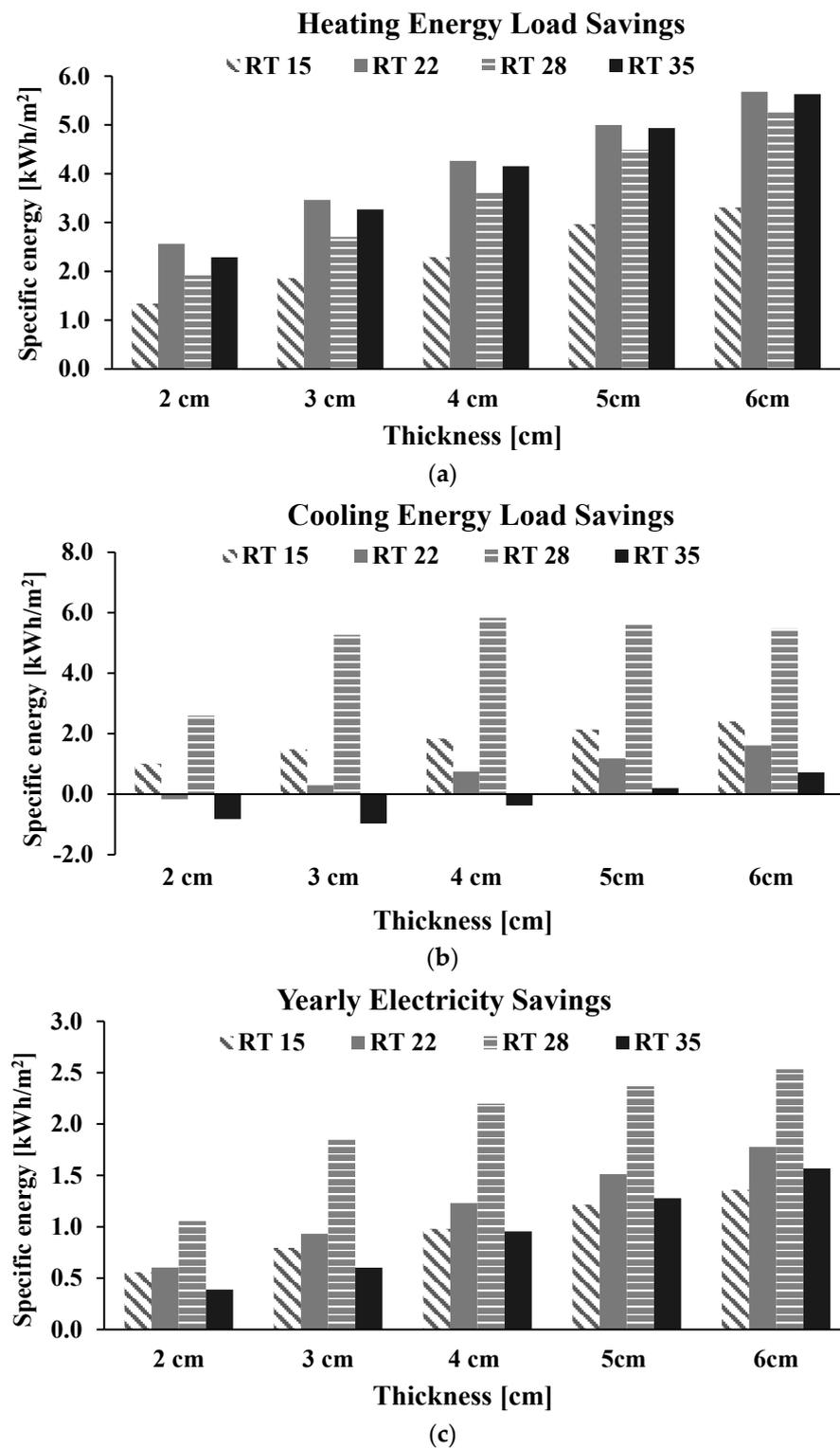
**Figure 2.** Energy savings of the PCM system compared to baseline scenario 1 for the (a) heating energy load, (b) cooling energy load, and (c) yearly electricity demand.
