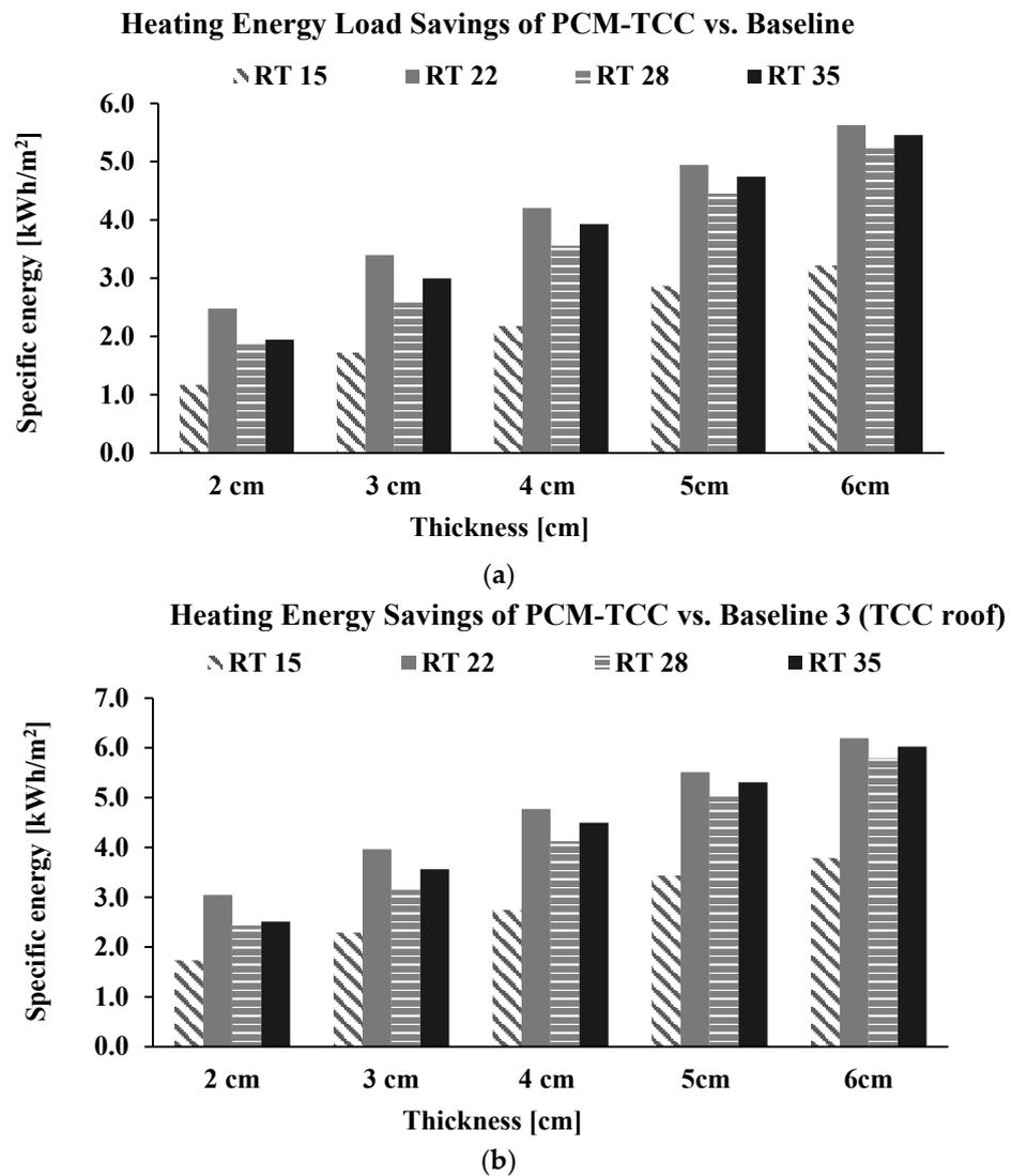
Figure 6. Heating energy load savings of the PCM-TCC roof system compared to (a) baseline scenario 1 and (b) baseline scenario 3.
