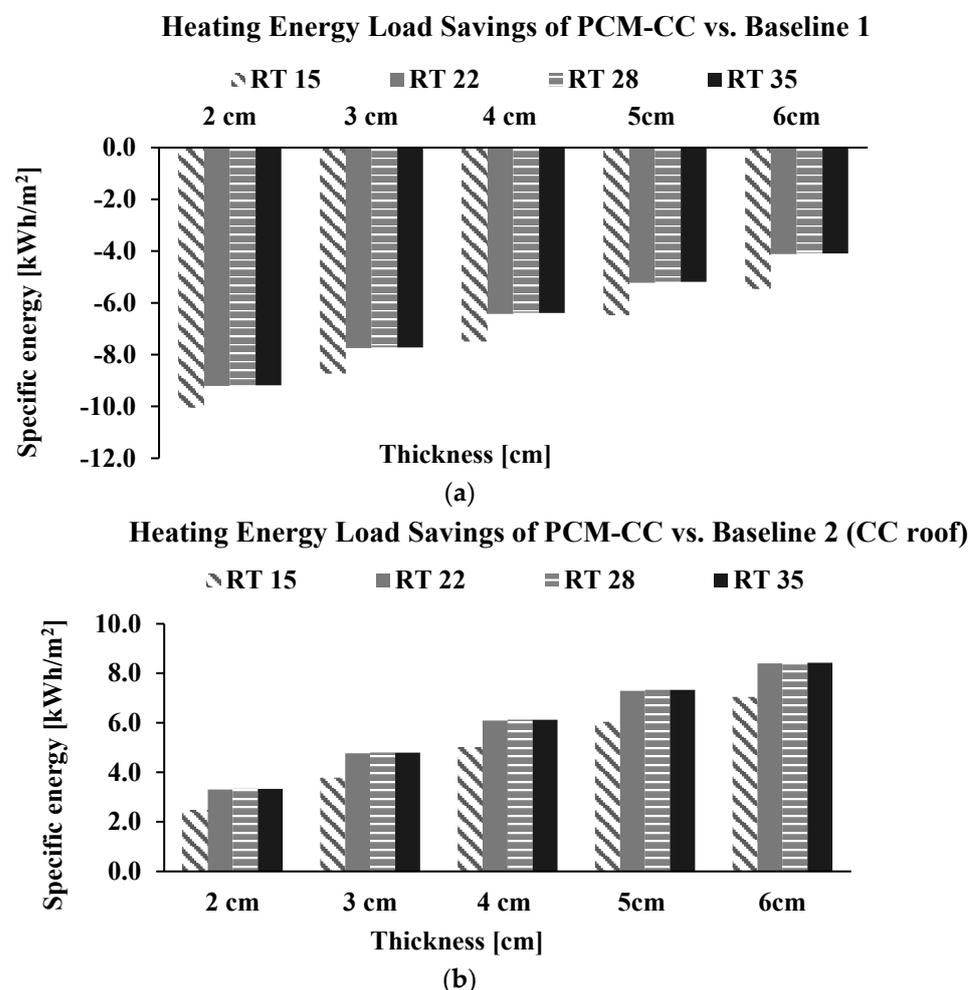
**Figure 3.** Heating energy load savings of the PCM-CC roof system compared to (a) baseline scenario 1 and (b) baseline scenario 2.
