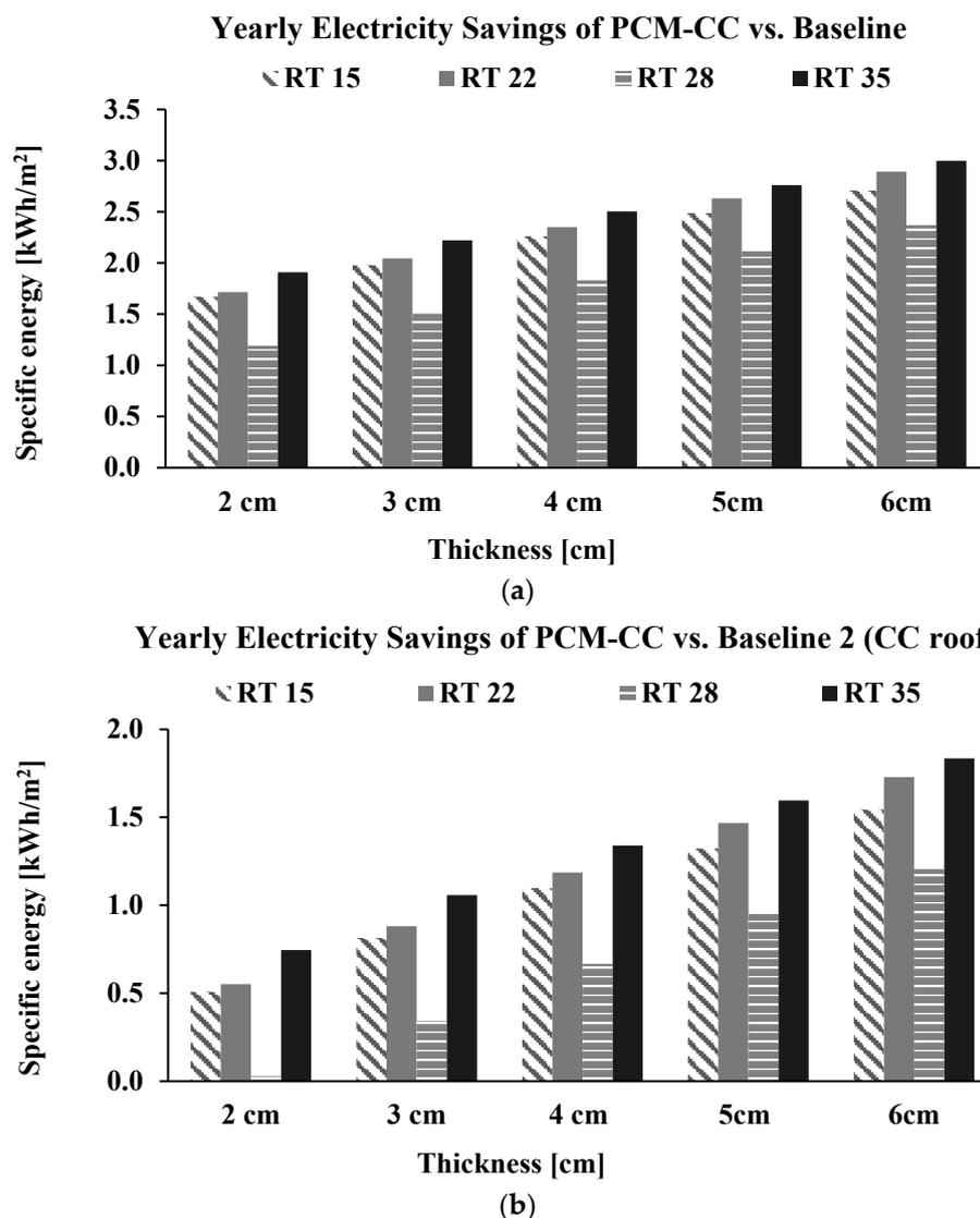
**Figure 5.** Yearly electricity savings of the PCM-CC roof system compared to (a) baseline scenario 1 and (b) baseline scenario 2.
