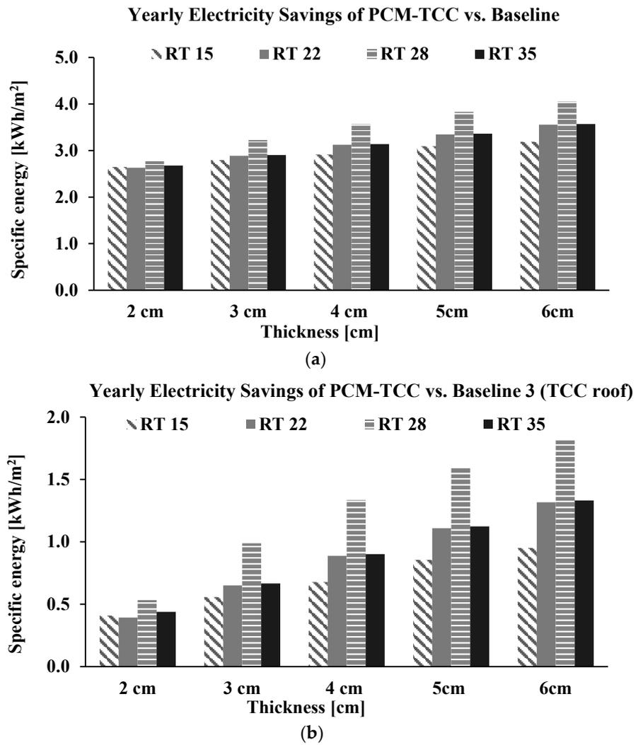
Figure 8. Yearly electricity savings of the PCM-TCC roof system compared to (a) baseline scenario 1 and (b) baseline scenario 3.
