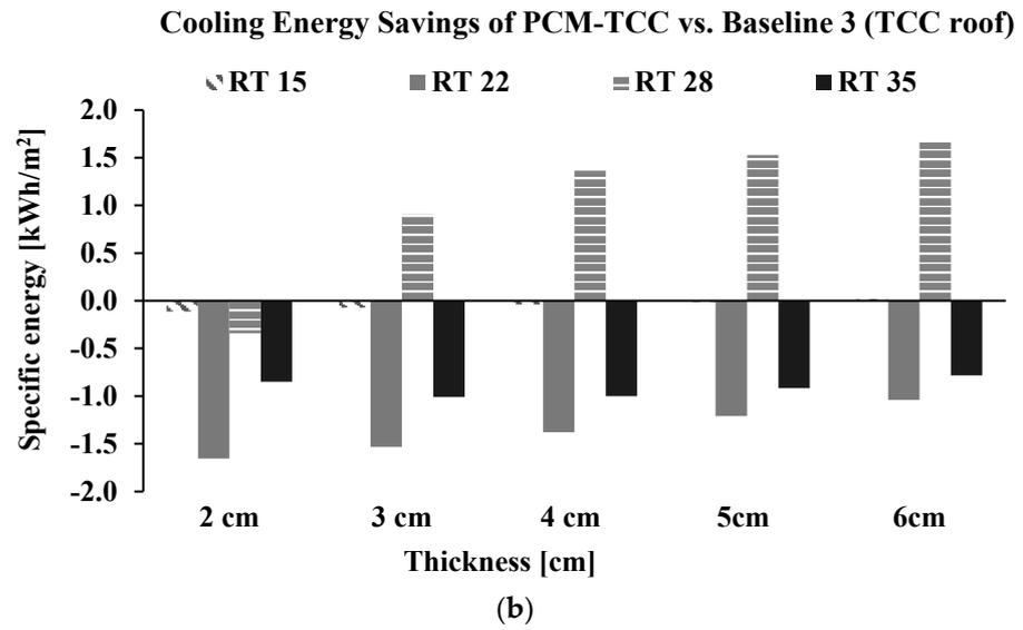
Figure 7. Cooling energy load savings of the PCM-TCC roof system compared to (a) baseline scenario 1 and (b) baseline scenario 3.
