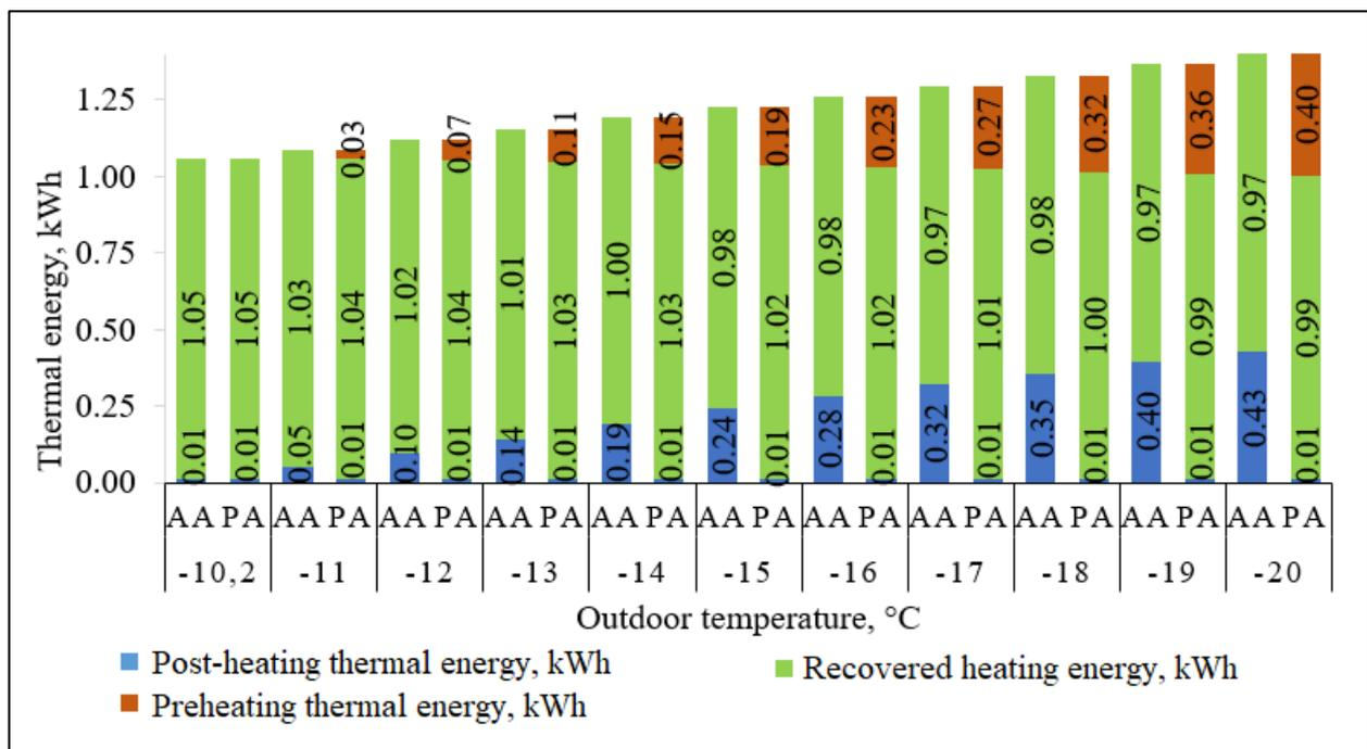
Figure 9. Energy balance of bypass (AA) and preheating (PA) defrosting methods, air volume 105 m<sup>3</sup>/h.
