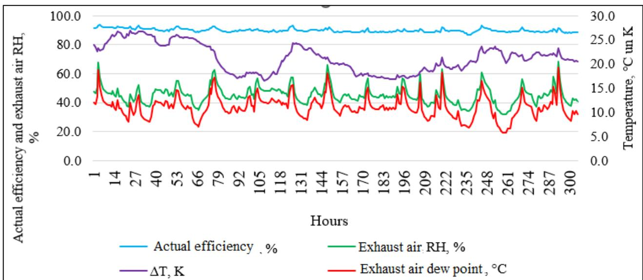
**Figure 6.** Changes in the efficiency of the heat recovery.
