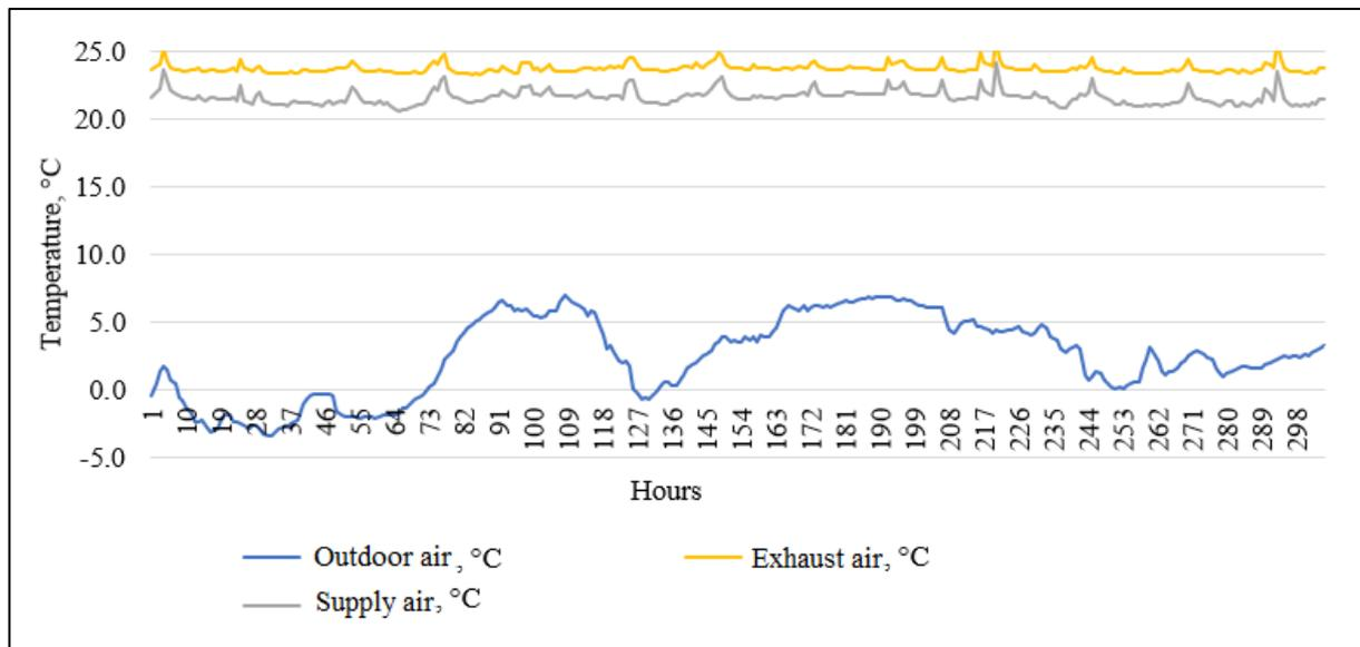
Figure 3. Outdoor, exhaust, and supply air temperature measurements.
