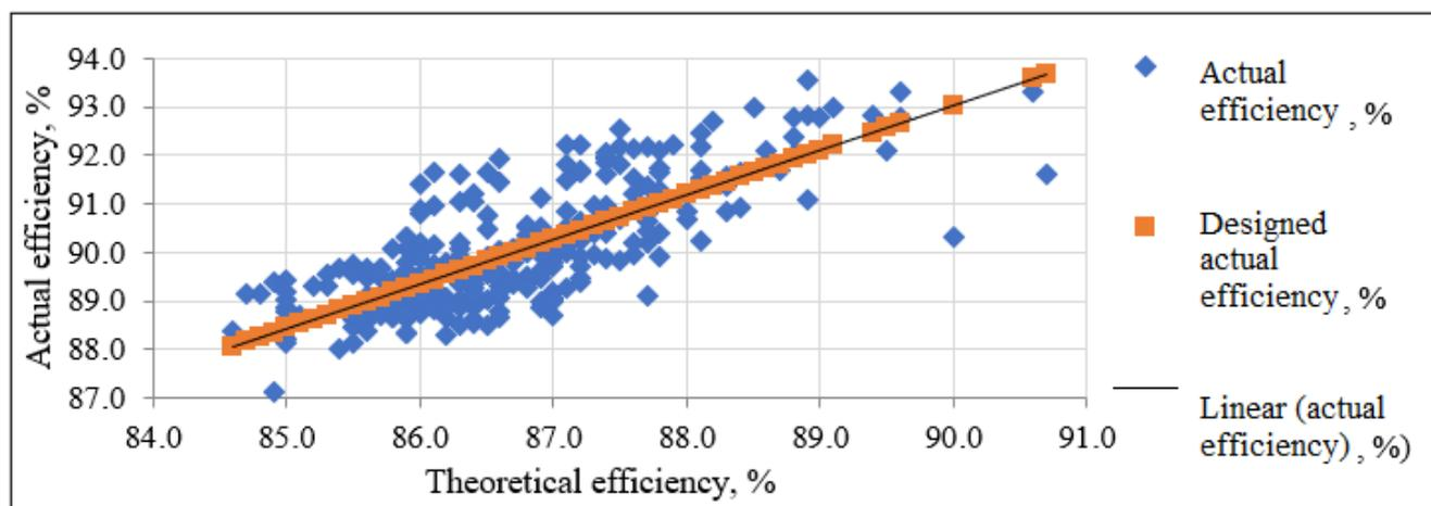
Figure 7. Regression model of the actual and theoretical heat recovery efficiency.
