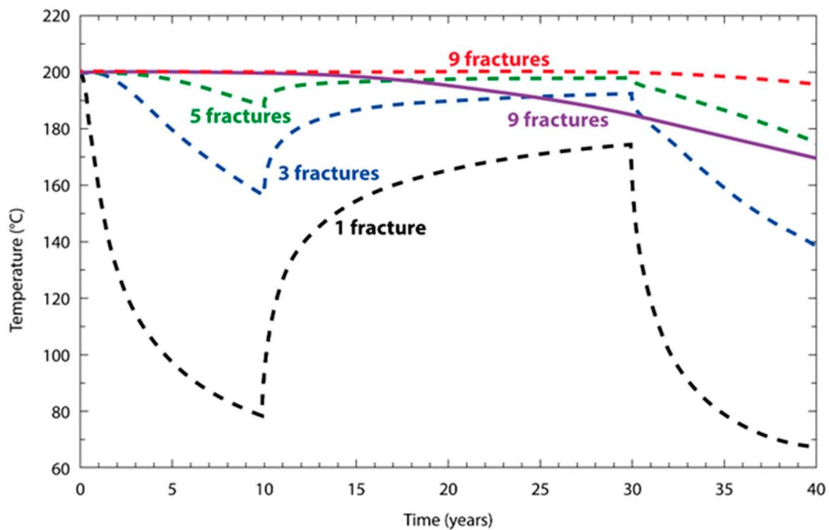
**Figure 6.** Production fluid temperature results from a multi-fractured PEGS reservoir with different fracture densities; dashed line: periodic extraction; solid line: continuous extraction. From [55], modified.
