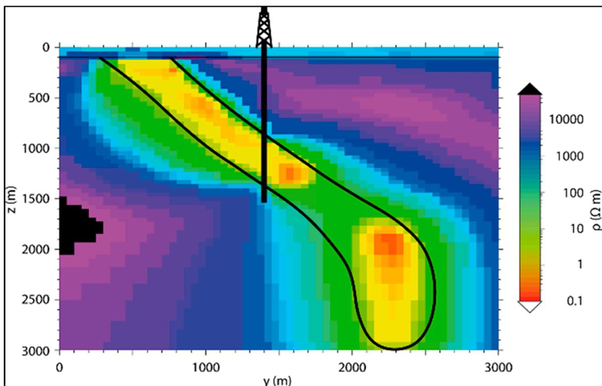
**Figure 5.** The numerical 2D inversion result of magnetotelluric data reveals a low-resistivity body at 2000–3000 m depth. From [42], modified.
