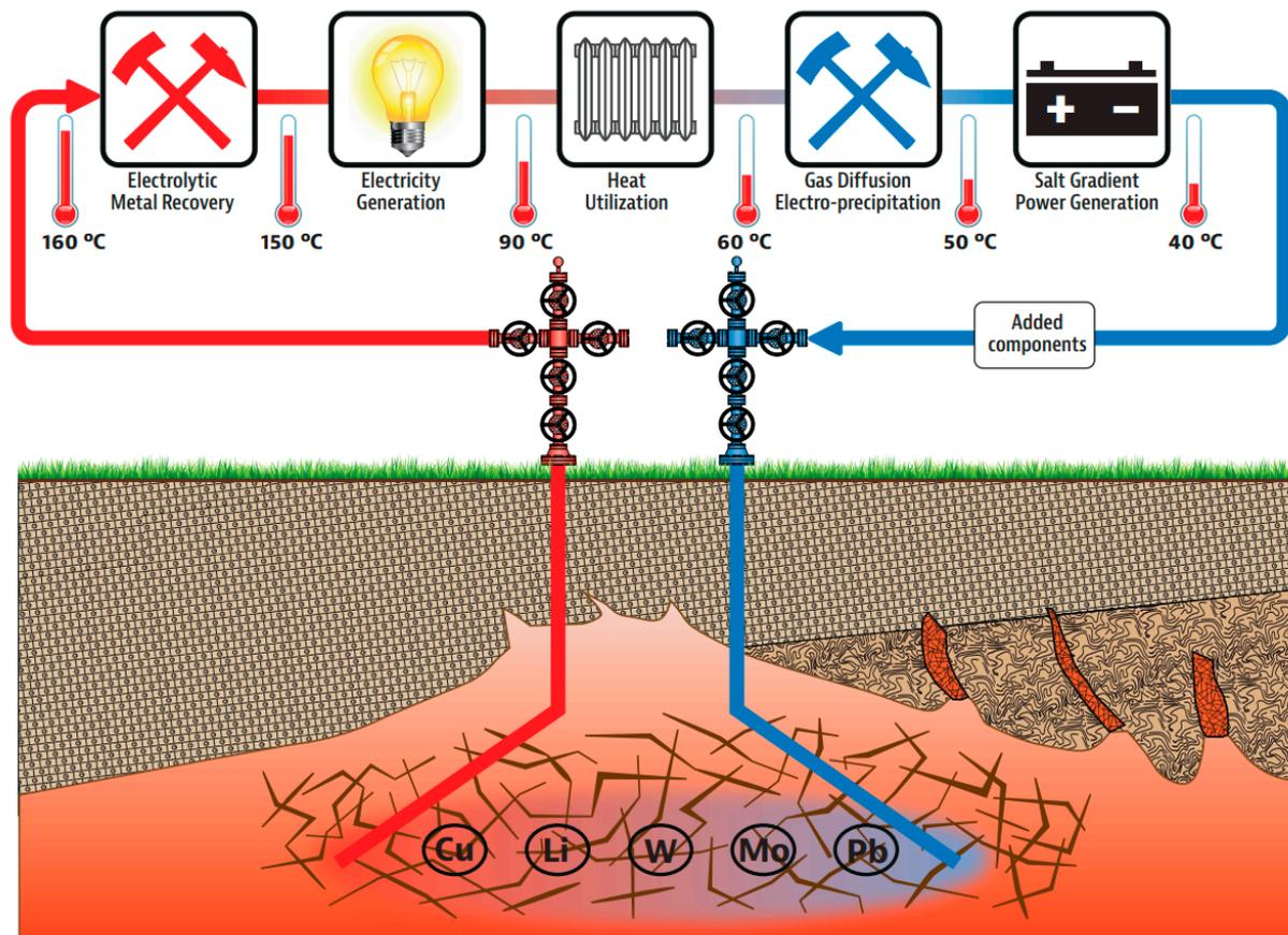
**Figure 4.** Schematic diagram of the overall CHPM system showing the surface technological components. From [41], modified.
