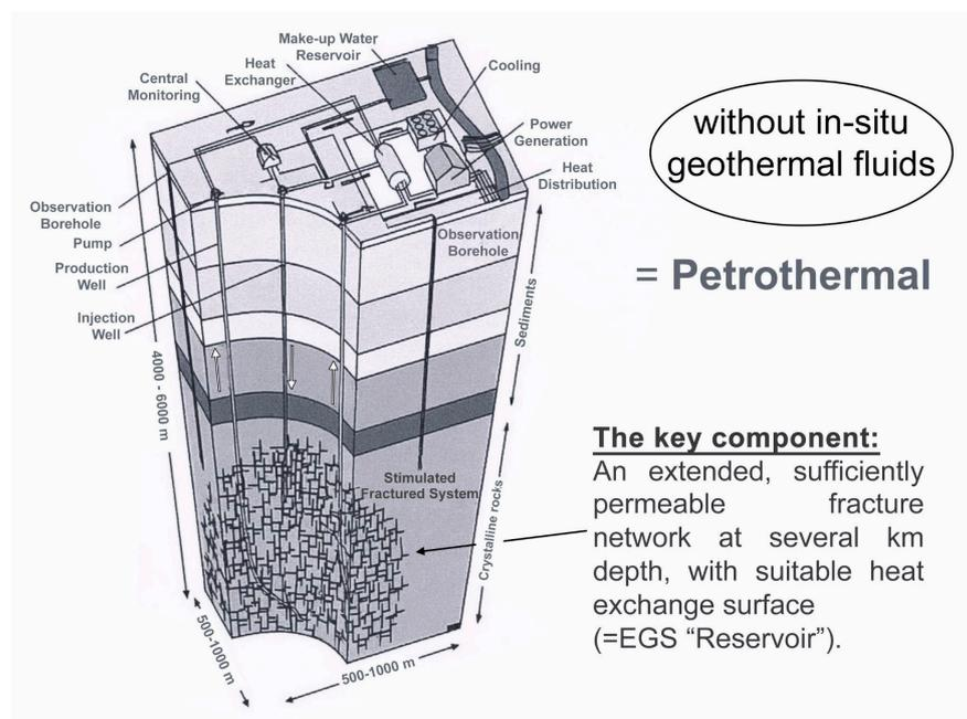
**Figure 10.** Schematics of a PEGS installation for power generation and district heating. From [75], modified.
