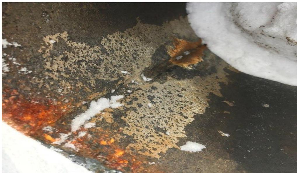
**Figure 1.** Oil pipeline section with groove corrosion damage.
