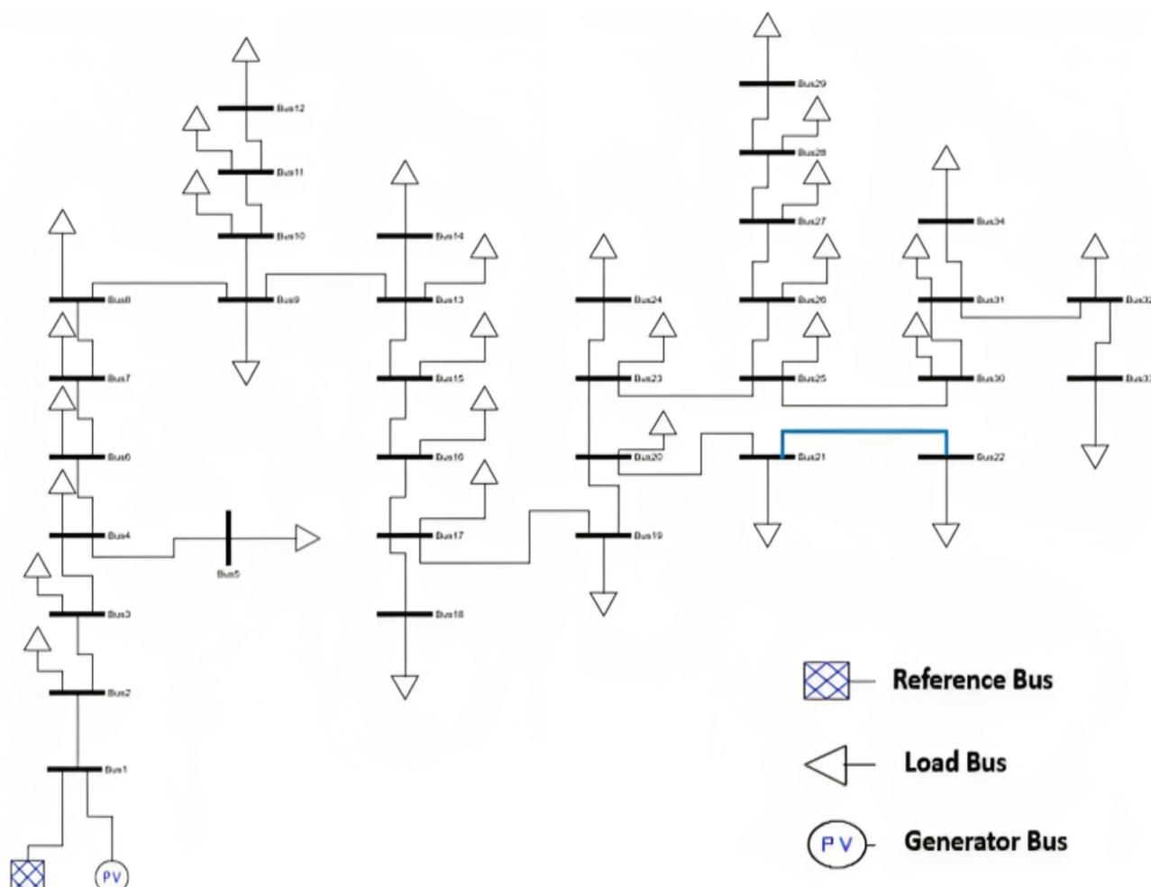
Figure 10. IEEE 34-Node Network design on PSAT Toolbox.
