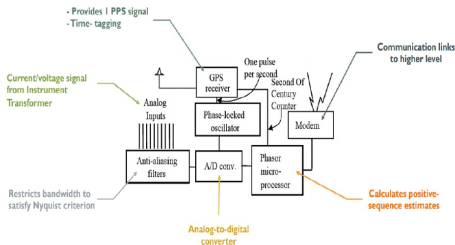
**Figure 1.** Functional block diagram of PMU.
