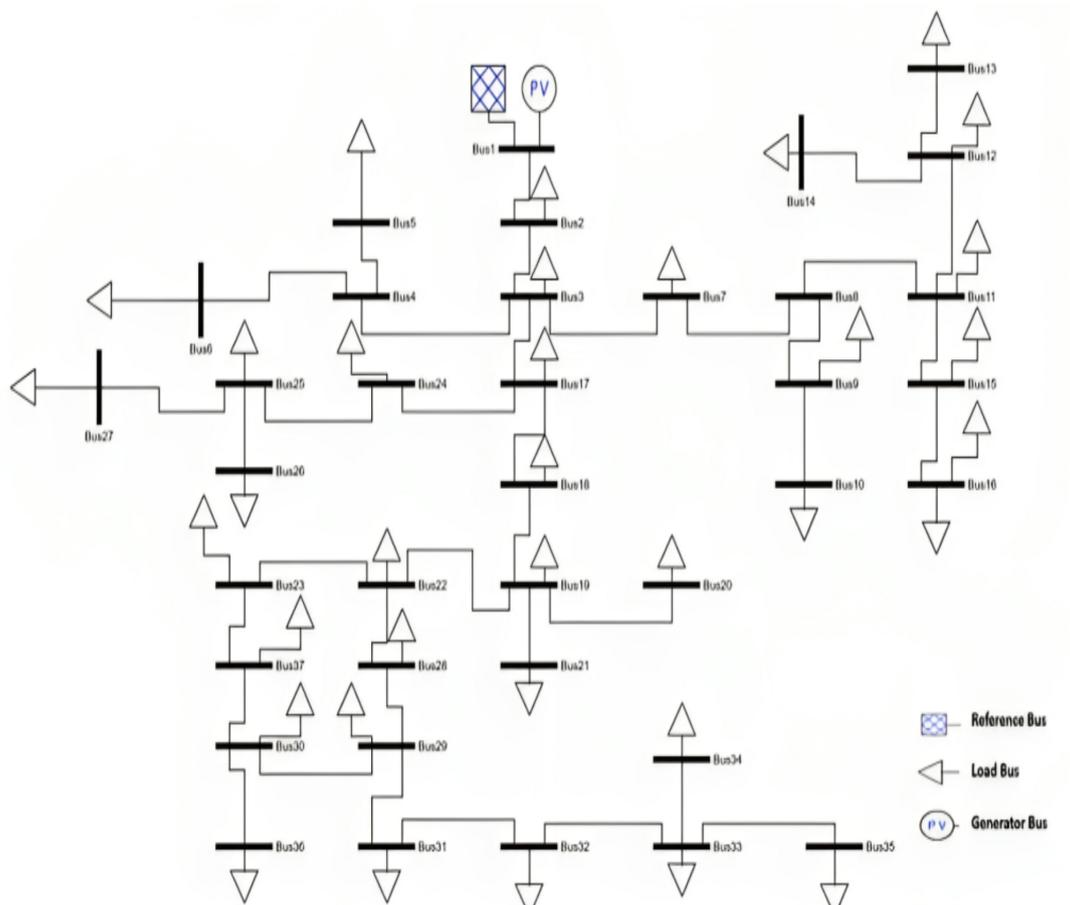
Figure 12. IEEE 37-Node Network design on PSAT Toolbox.
