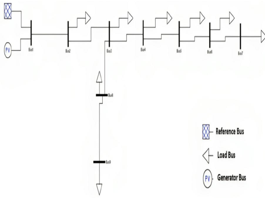
**Figure 6.** IEEE 9-Node Network design on PSAT Toolbox.
