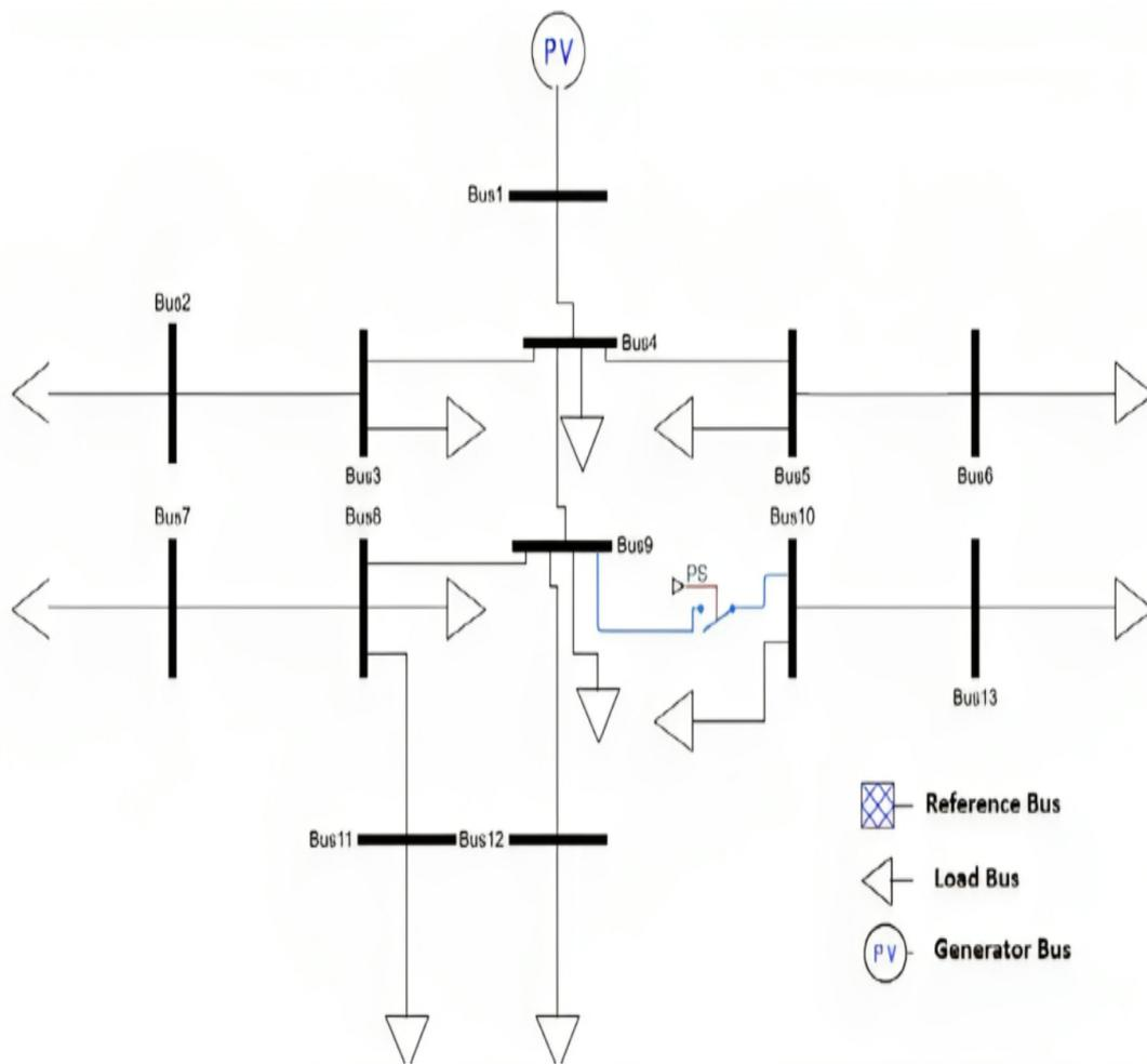
Figure 8. IEEE 13-Node Network design on PSAT Toolbox.
