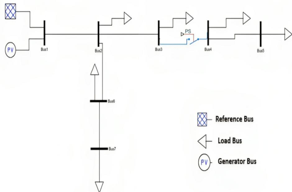
**Figure 4.** IEEE 7-Node Network design on PSAT Toolbox.
