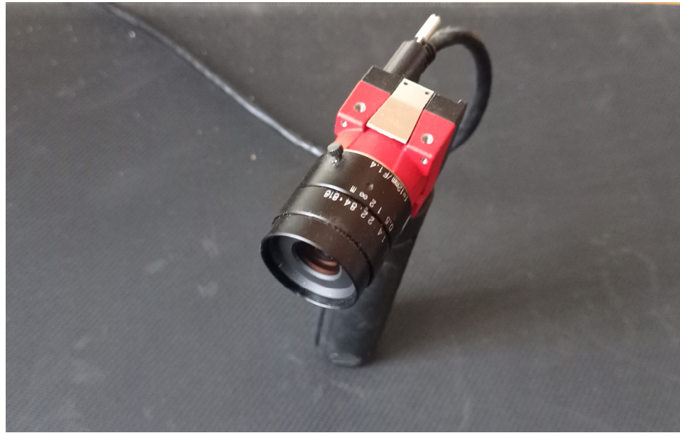
Figure 1. Alvium 1800 U-050 industrial camera.
