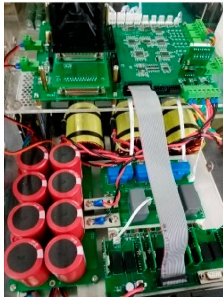
**Figure 11.** The single-phase H-bridge experimental prototype.
