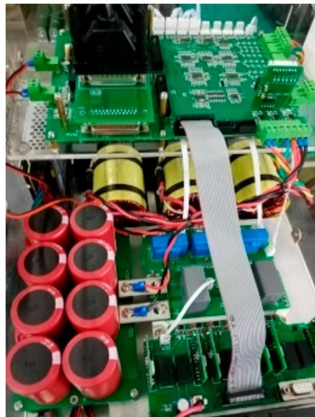
**Figure 11.** The single-phase H-bridge experimental prototype.
