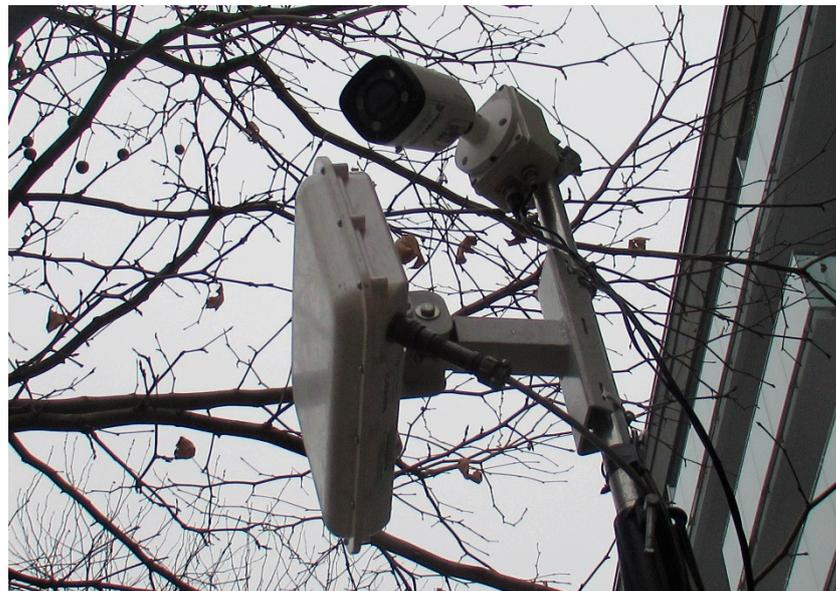
**Figure 2.** Perpendicular radar and CCTV IP camera (own study).
