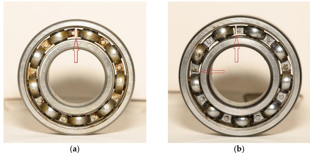
**Figure 3.** Faulty bearings (6206) with cage defects: (a) one gap and (b) two gaps.
