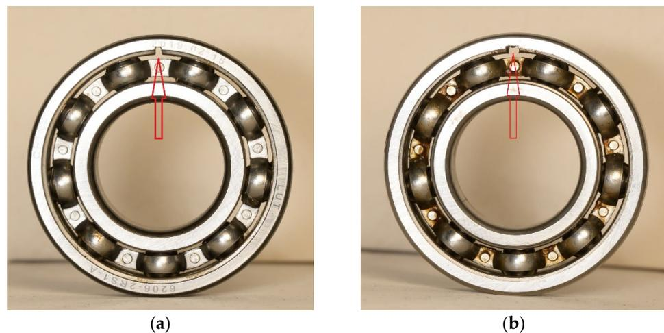
**Figure 2.** Faulty bearings (6202) with outer race defects: (a) 1 mm wide groove and (b) 3 mm wide groove.
