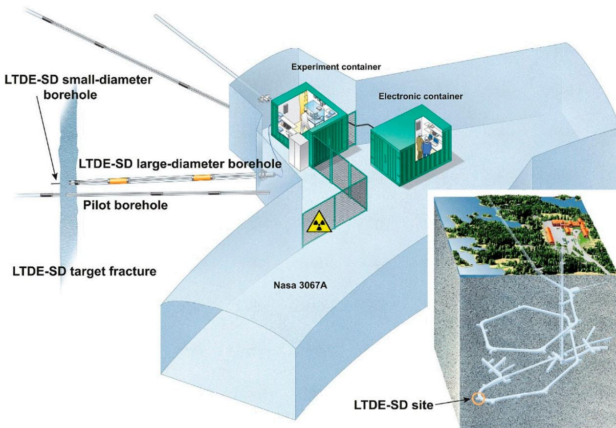
**Figure 6.** Illustration of the LTDE-SD experimental site at the ÄHRL, Sweden (from [23]).
