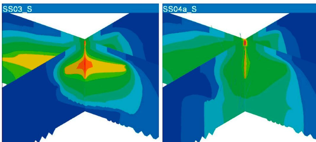
**Figure 4.** Contoured normalized drawdown for the Posiva/VTT small zone models for case SS03 (no monitoring boreholes) and case SS04a (including monitoring boreholes). Both are uncalibrated models (from [20]). The pumped borehole is located at the intersection of the two slices utilized for visualization purposes.
