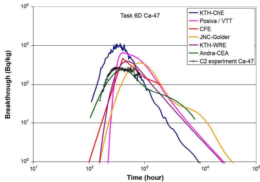
**Figure 3.** Inter-comparison of calculated breakthrough curves for Ca-47 in Task 6D together with the TRUE Block Scale C2 tracer test results [19].
