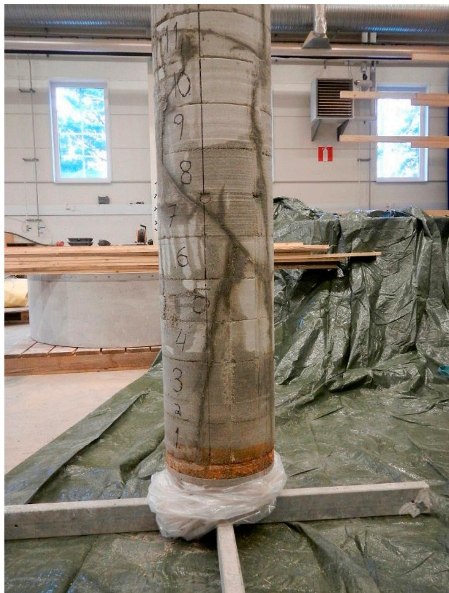
**Figure 9.** Bentograph showing traces of the flowing fractures on the surface of the retrieved buffer material from a deposition hole.
