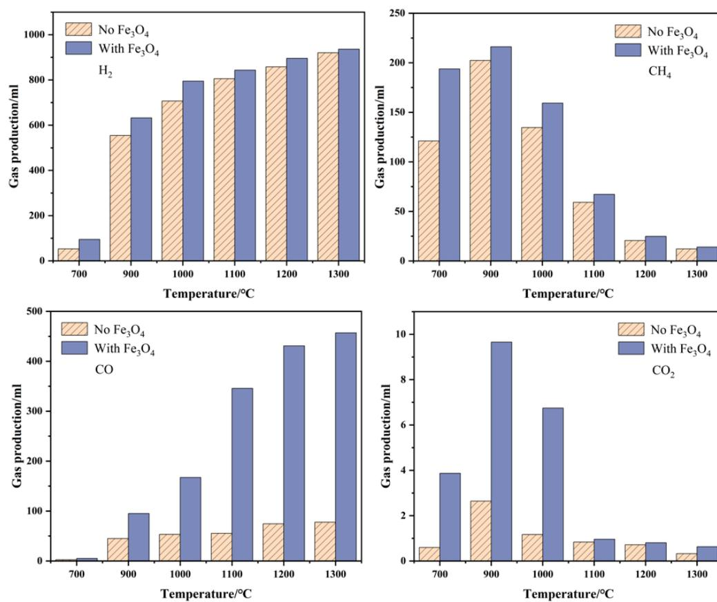
Figure 8. Gas production of WEO at different pyrolysis temperatures.
