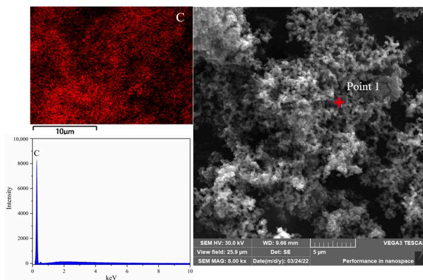
**Figure 10.** SEM-EDS analysis of cracking carbon.
