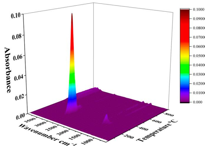
Figure 5. Three-dimensional FTIR spectra of pyrolysis gas products from WEO.
