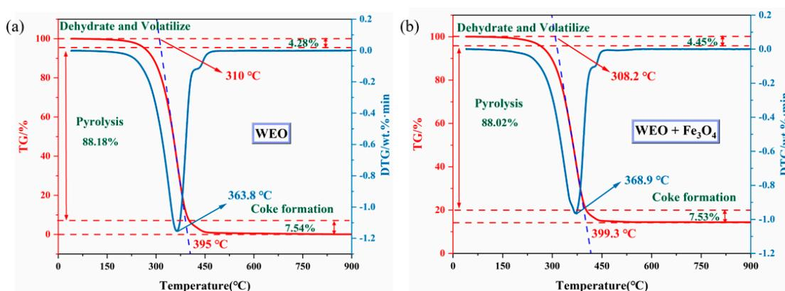
**Figure 3.** TG–DTG curve of (a) WEO and (b) WEO with  $\text{Fe}_3\text{O}_4$  at a heating rate of  $10\text{ }^\circ\text{C}/\text{min}$ .
