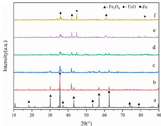
**Figure 11.** XRD patterns of Fe<sub>3</sub>O<sub>4</sub> samples, (a) 700 °C; (b) 900 °C; (c) 1000 °C; (d) 1100 °C; (e) 1200 °C; (f) 1300 °C.
