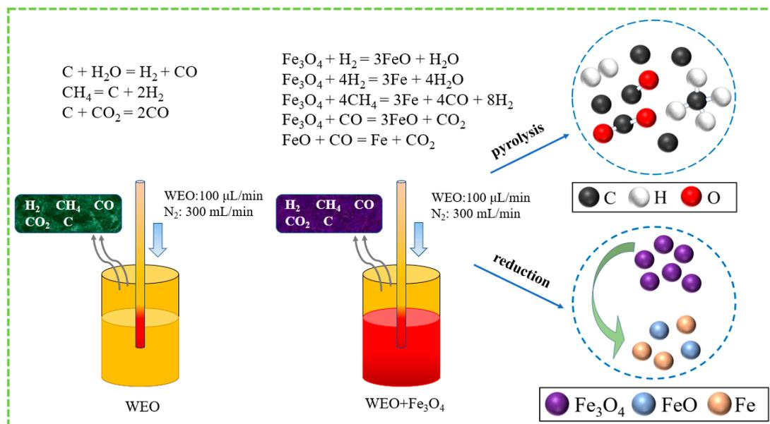
Figure 6. Reaction mechanism of WEO cracking.
