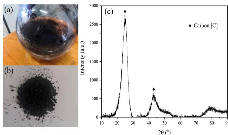
**Figure 9.** Carbon deposition during cracking process, (a) flask for cooling; (b) collected carbon from the flask (a); (c) XRD pattern of generated carbon.
