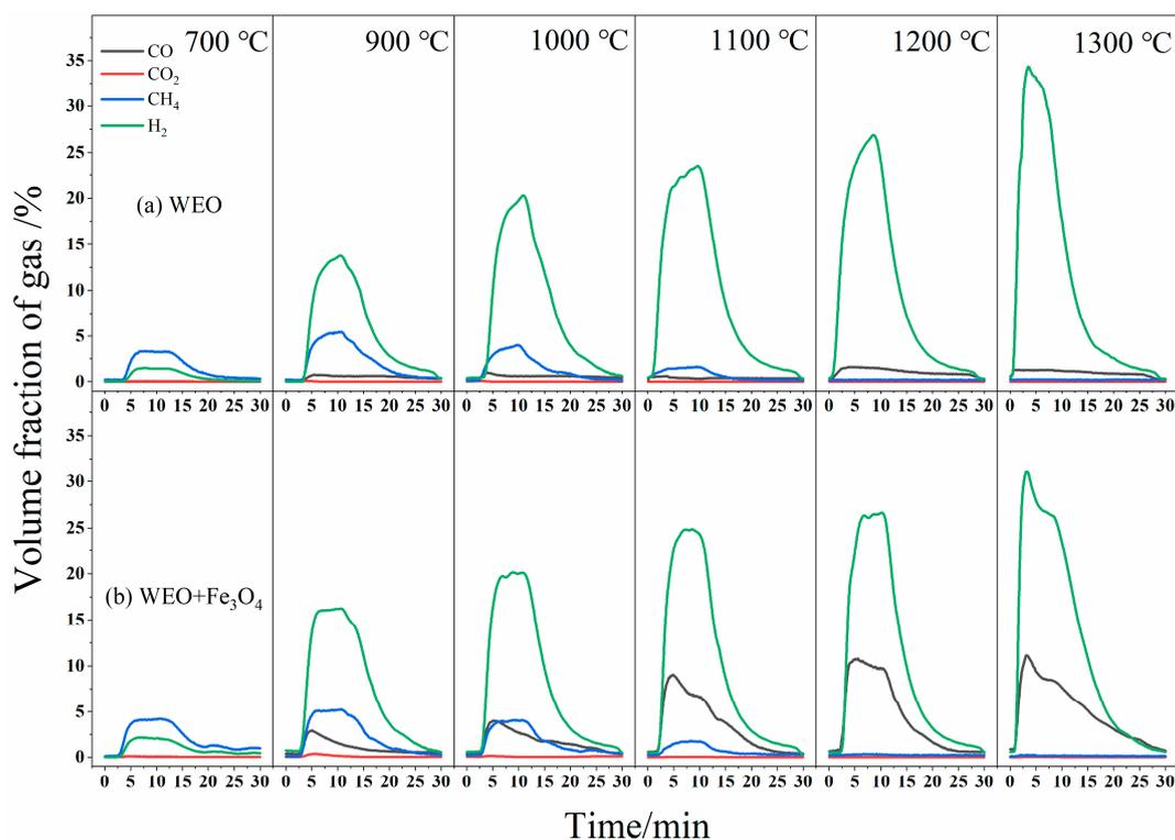
**Figure 7.** The volume fraction of produced gas as a function of time, (a) WEO cracking directly; (b) WEO cracking with 1.5 g  $\text{Fe}_3\text{O}_4$ .
