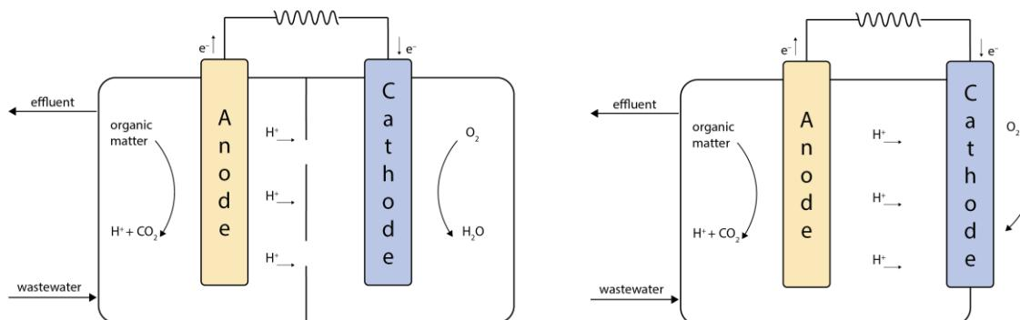
**Figure 2.** Two types of MFC—one- and two-chamber.
