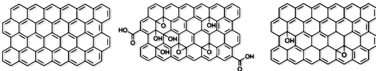
**Figure 1.** Graphene (G), graphene oxygen (GO), and reduced graphene oxygen (rGO).
