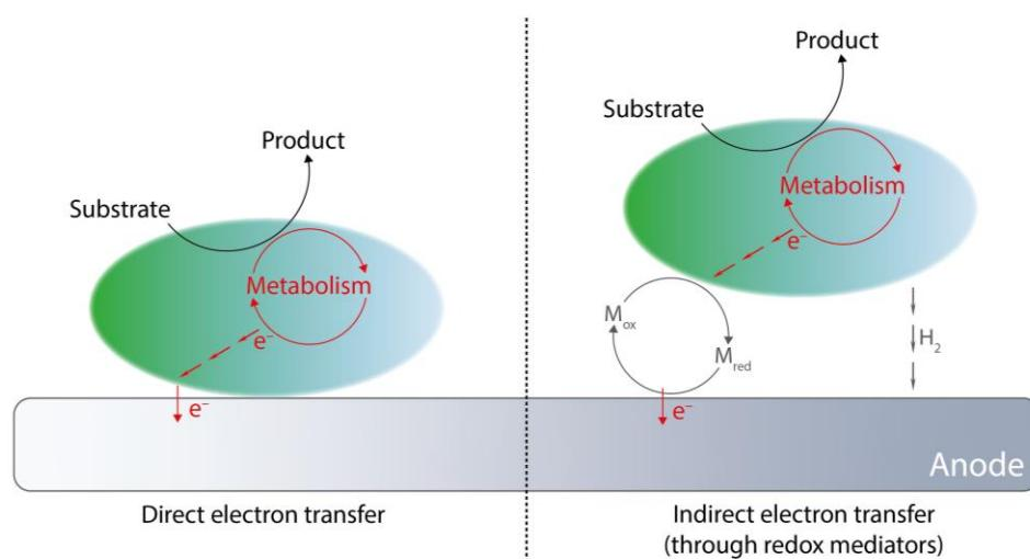
**Figure 3.** Mechanisms of electron transfer between micro-organisms and anode in MFCs.
