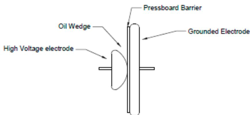
Figure 2. The model electrode system for the oil wedge considered in this study.
