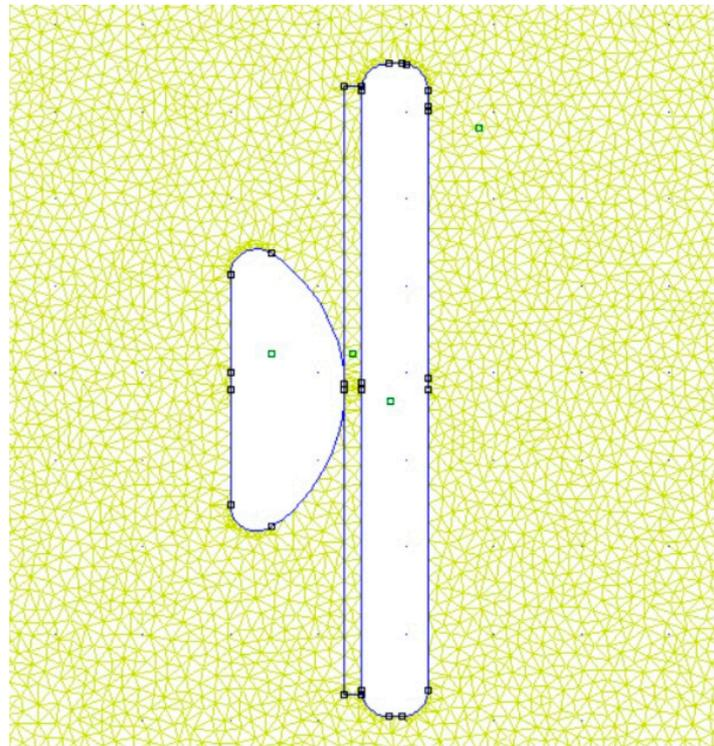
**Figure 6.** The model electrode system of the oil-wedge type constructed in FEMM software with applied calculating mesh.
