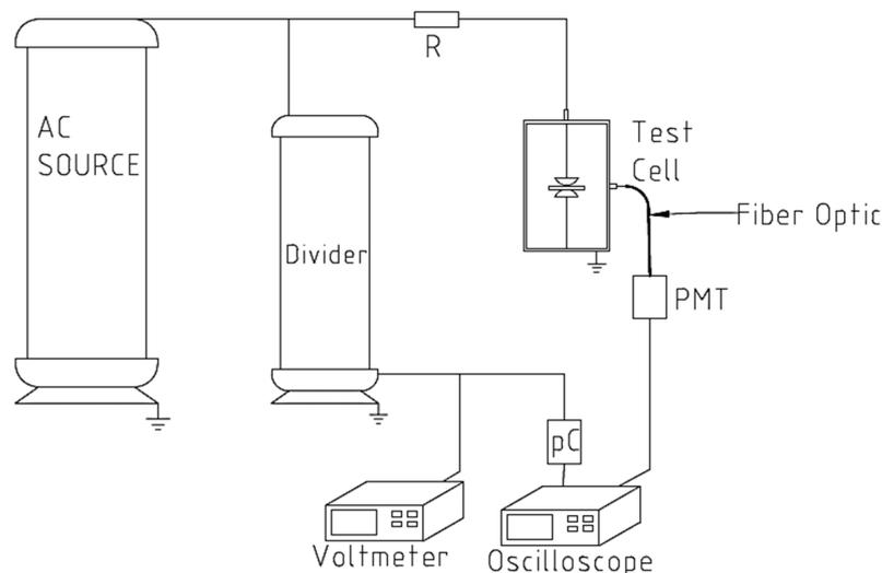
**Figure 3.** Experimental setup used during the measurements: R—limiting resistor, pC—quadrupole, PMT—photomultiplier.
