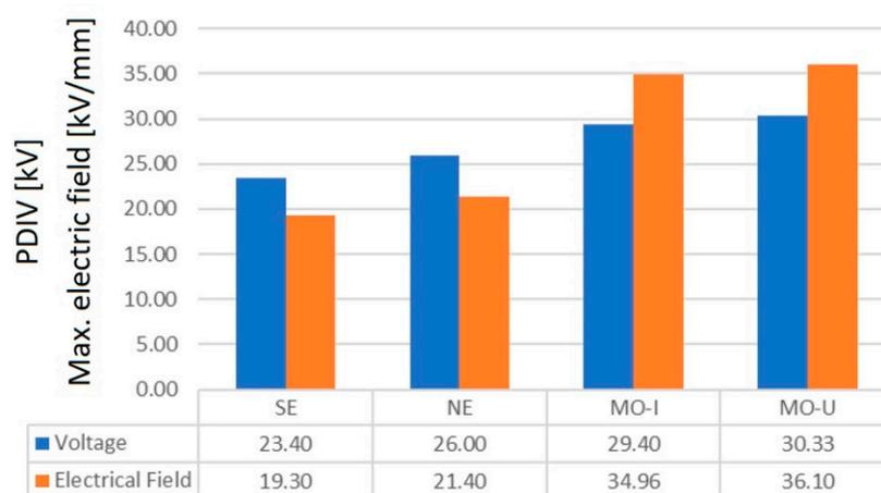
**Figure 8.** PDIV and maximum electric field in the oil wedge for the tested electrode model.
