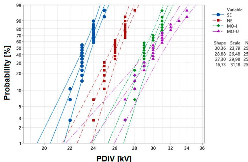
**Figure 5.** Weibull distribution plots of partial-discharge inception voltage (PDIV) for the distinctive liquids considered: SE—synthetic ester, NE—natural ester, MO-I—inhibited mineral oil, MO-U—uninhibited mineral oil. Shape—shape parameter of Weibull distribution function, Scale—scale parameter of Weibull distribution function, N—number of random variables.
