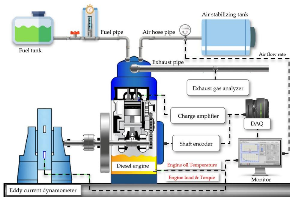
Figure 2. Schematic illustration of the experimental setup [49].
