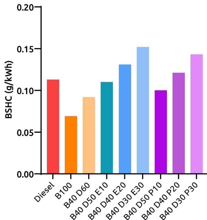
Figure 8. Brake specific hydrocarbon emissions for tested fuels at full engine load.
