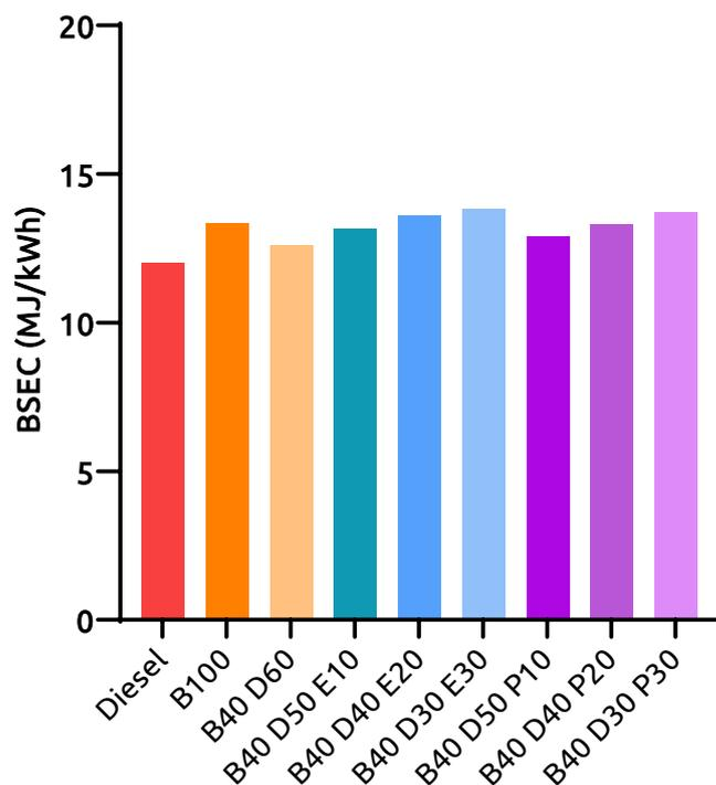
Figure 4. Brake specific energy consumption for tested fuels at full engine load.
