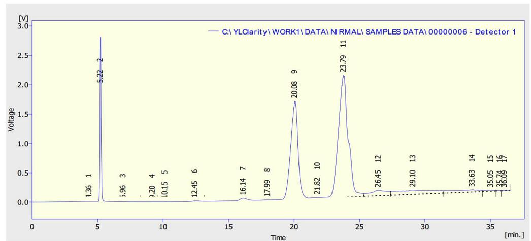
**Figure 1.** Results from GC-FID instrument with palm biodiesel sample. Dotted line shows overall trend.
