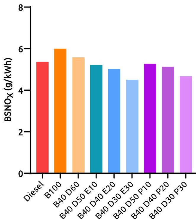
**Figure 9.** Brake Specific oxides of nitrogen emissions for tested fuels at full engine load.
