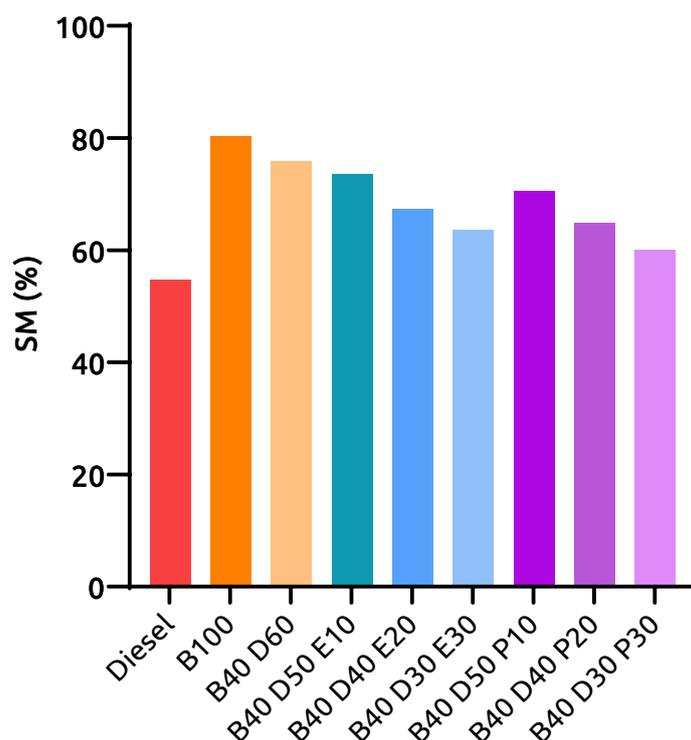
Figure 10. Smoke opacity for tested fuels at full engine load.
