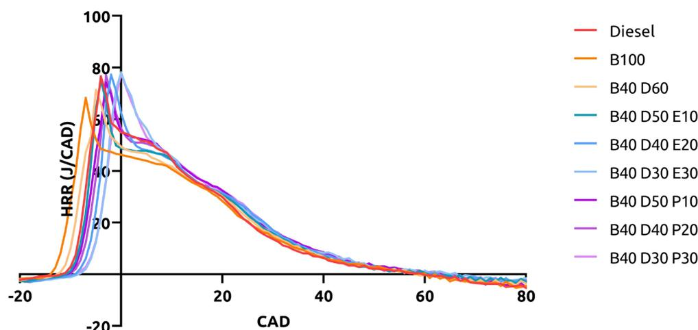
Figure 6. Heat release rate for tested fuels at full engine load.
