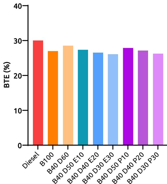
Figure 3. Brake thermal efficiency for tested fuels at full engine load.
