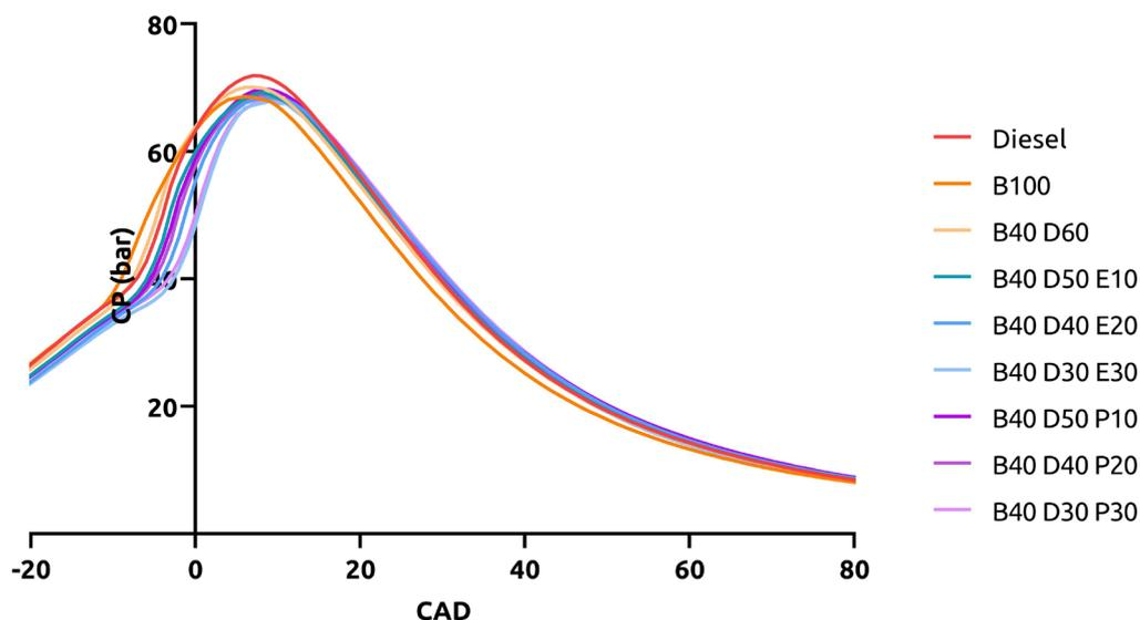
Figure 5. In-cylinder pressure for tested fuels at full engine load.
