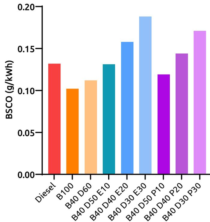
Figure 7. Brake specific carbon monoxide emissions for tested fuels at full engine load.
