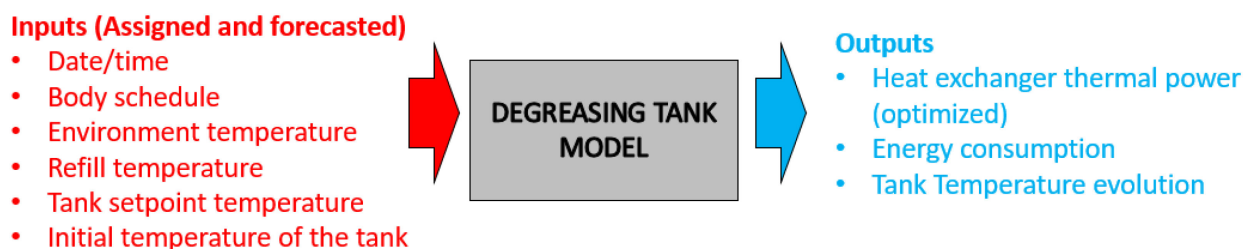
Figure 8. Complete input–output list for the usage of the degreasing tank model in simulation mode.
