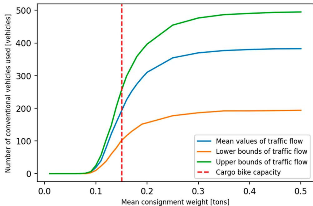
**Figure 5.** The number of conventional vehicles that deliver loads directly to clients for the study area of San Sebastian.
