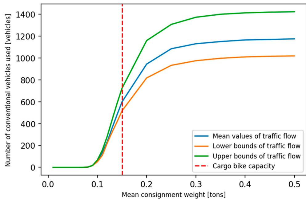
**Figure 4.** The number of conventional vehicles that deliver loads directly to clients for the study area of Krakow.
