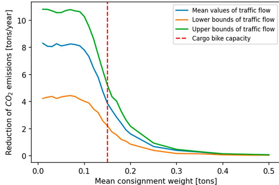
**Figure 7.** Dependence of CO<sub>2</sub> reduction on the consignment weight in San Sebastian.
