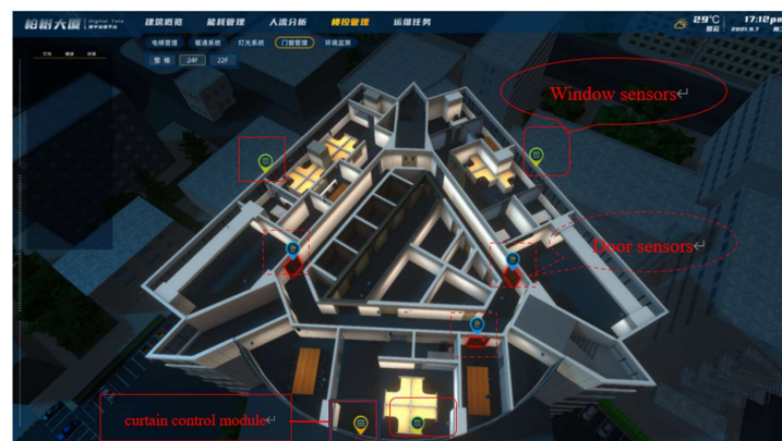
Figure 8. Door, window, and curtain intelligent management interface for the 24th floor.
