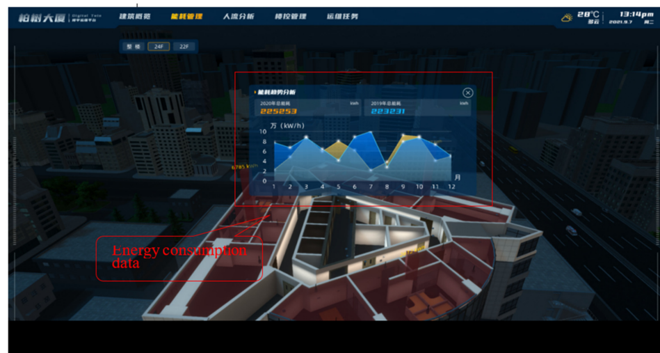
Figure 11. Building energy consumption monitoring and management interface.
