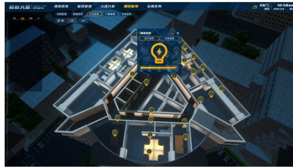
Figure 9. The lighting monitoring and intelligent management interface for the 24 floor.
