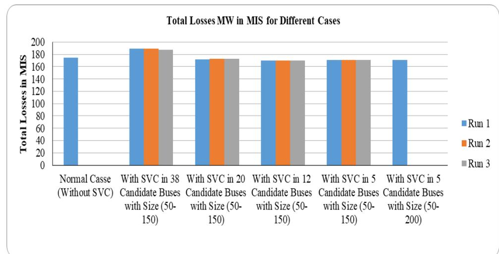
Figure 4. Total MW losses in MIS for different cases with and without SVC.
