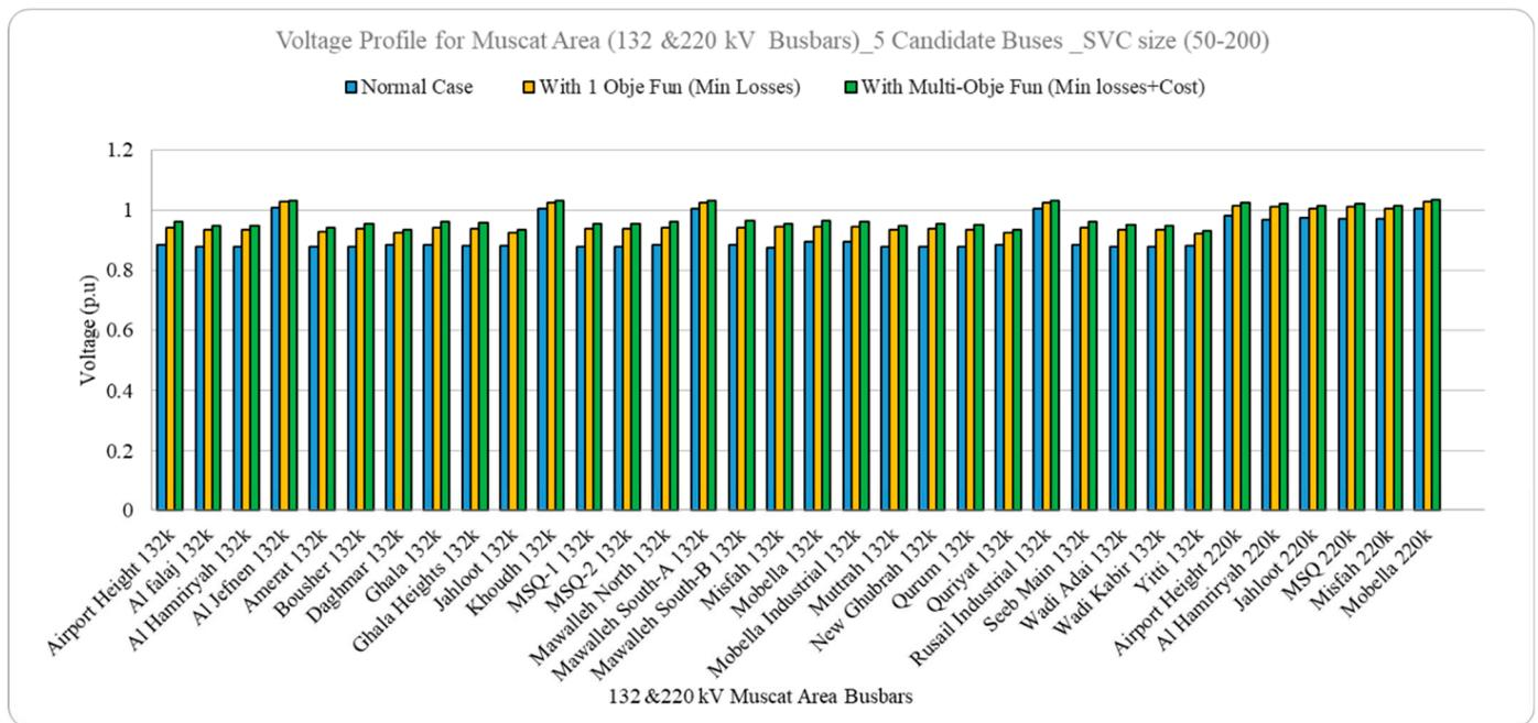
**Figure 6.** Voltage profile for 132 kV and 220 kV stations with optimal SVC sizes for five candidate buses with different objective.
