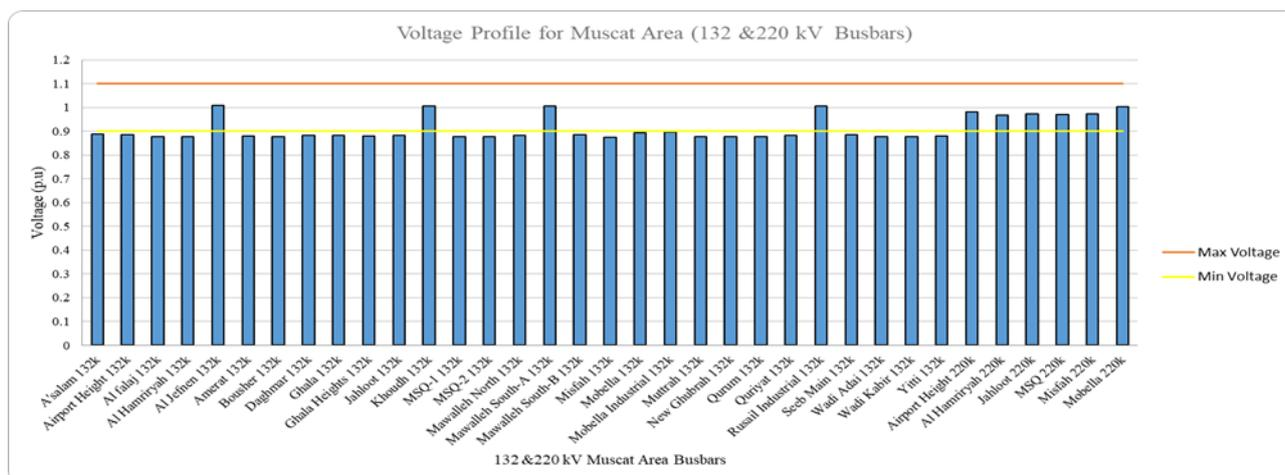
**Figure 1.** Voltage profile for 132 kV and 220 kV in the Muscat area using a MATLAB Model.
