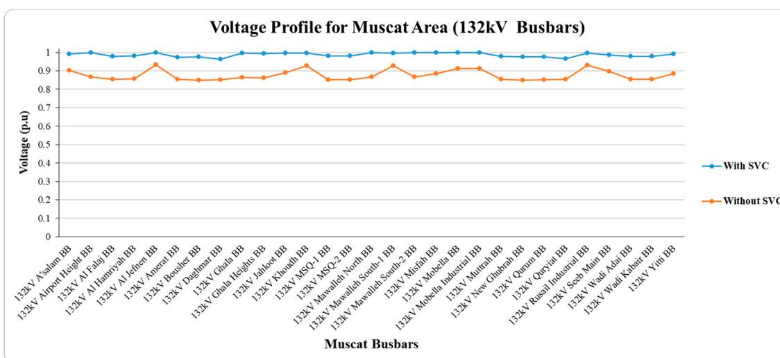
**Figure 7.** Voltage profile for 132 kV stations with and without SVC using DigSILENT software.
