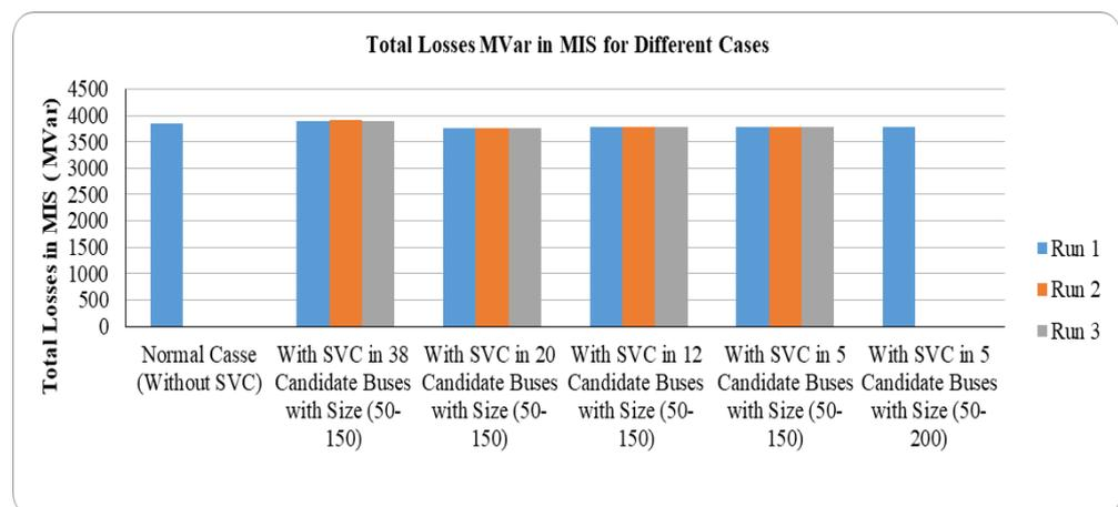
Figure 5. Total MVar losses in MIS for different cases with and without SVC.
