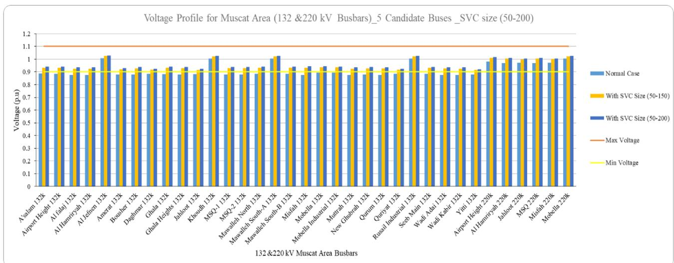
**Figure 3.** Voltage profile for 132 kV and 220 kV stations with optimal SVC sizes for five candidate buses for trace of size [50–200].
