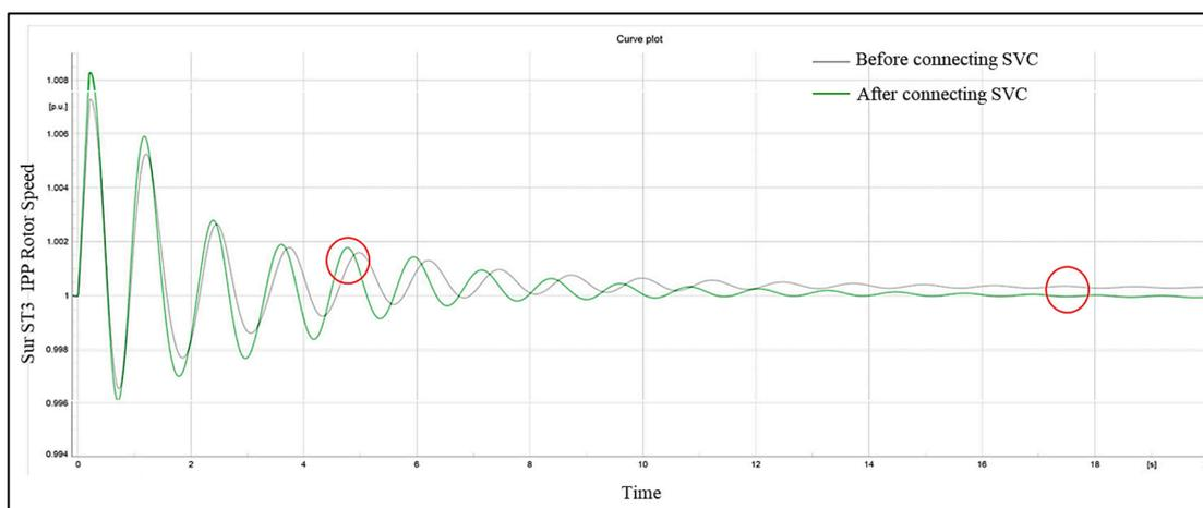
Figure 8. Rotor angle for Sur ST3 after fault cleared.
