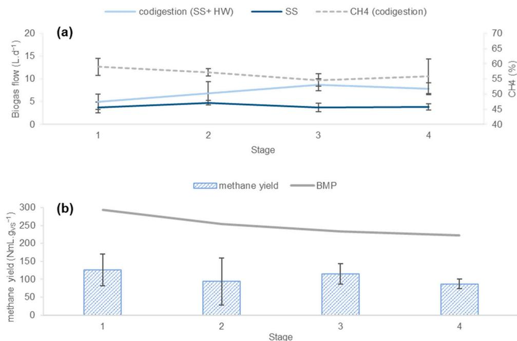
**Figure 7.** Productivity of the phase 2 process including (a) the average biogas quantity and quality of D2 and average biogas quantity of D1; (b) average methane yield of D2 and BMP.
