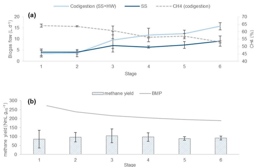
**Figure 5.** Productivity of the process in phase 1 including (a) average biogas quantity and quality of D2 (SS + HW) as well as average biogas quantity of D1 (SS only); (b) average methane yield of D2 and BMP.
