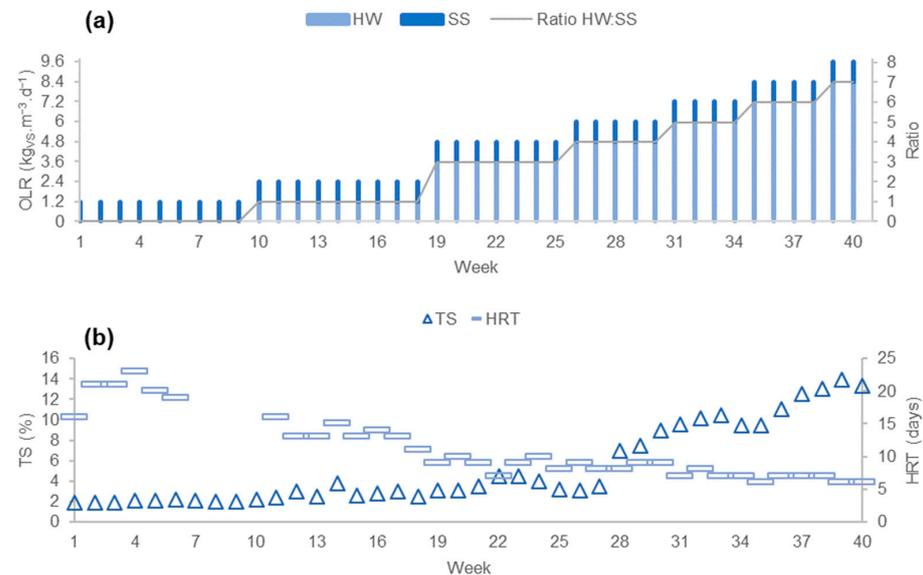
**Figure 2.** Operational scheme of phase 1 in D2: (a) OLR and ratio changes; (b) changes in TS and HRT.
