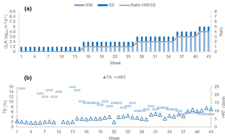
**Figure 3.** Operational scheme of phase 2 in D2 including (a) OLR and ratio changes; (b) changes in TS and HRT.
