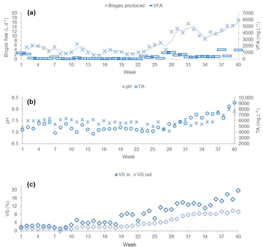
**Figure 4.** Operational parameters of phase 1 in D2 including (a) volumetric biogas production and VFA; (b) TA and pH; (c) VS in and VS out.
