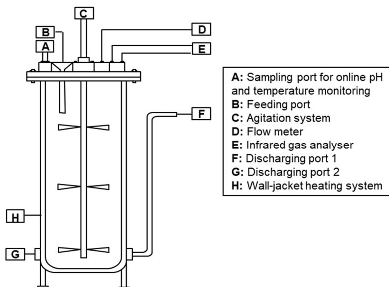
**Figure 1.** Experimental setup of the continuous stirred-tank reactor (CSTR-10S, Bioprocess Control, Lund, Sweden).
