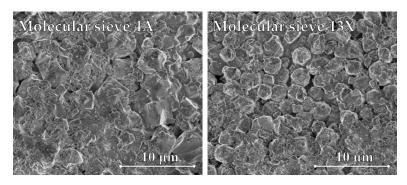
Figure 4. Scanning electron microscope images of molecular sieves 4A and 13X.
