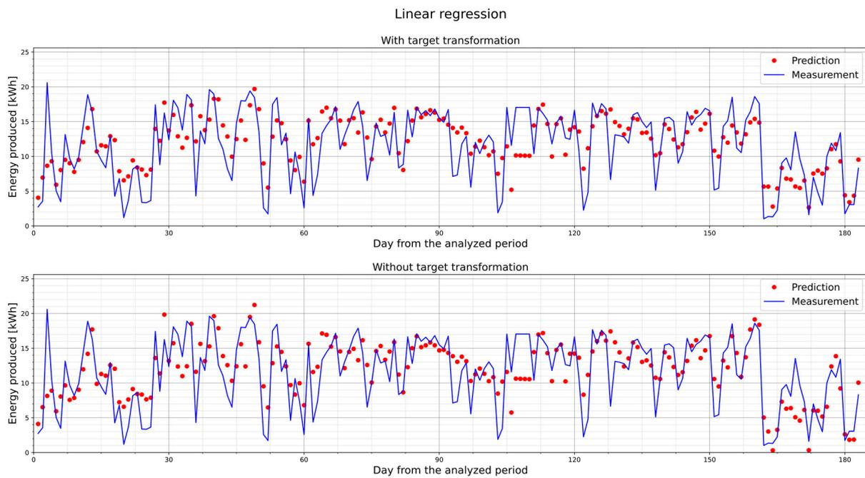
**Figure 9.** The energy produced in each day of the analyzed period and forecasts for the PV1 power plant using the linear regression model for  $m = 2$  and predictions with and without target transformation (MinMaxScaler).
