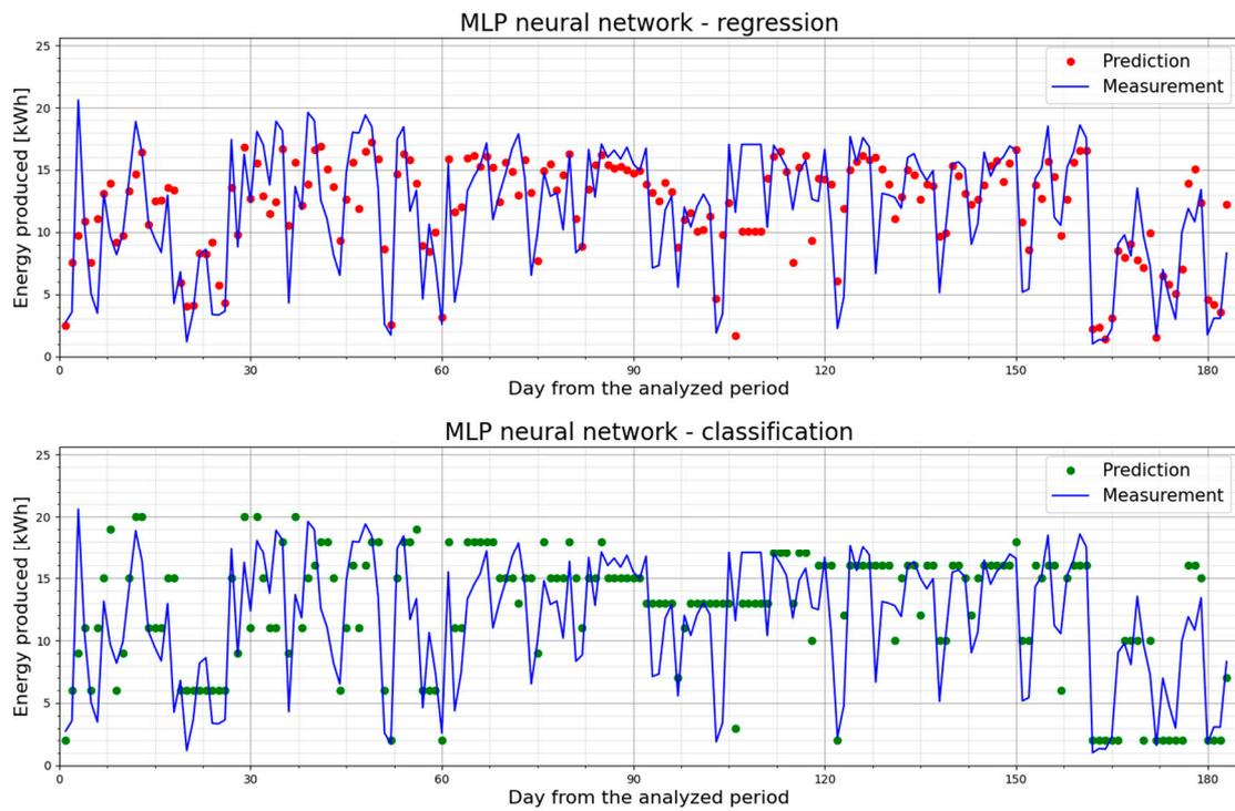
**Figure 4.** The produced energy in each day of the analyzed period and forecasts for the PV1 power plant using the MLPRegressor model and MLPClassifier model (a discretization width of 1 kWh).
