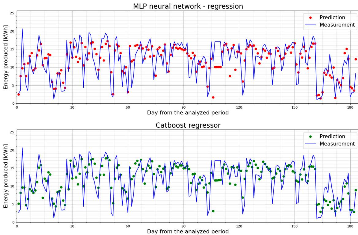
**Figure 5.** The produced energy in each day of the analyzed period and forecasts for the PV1 power plant using the MLPRegressor and CatBoostRegressor models.
