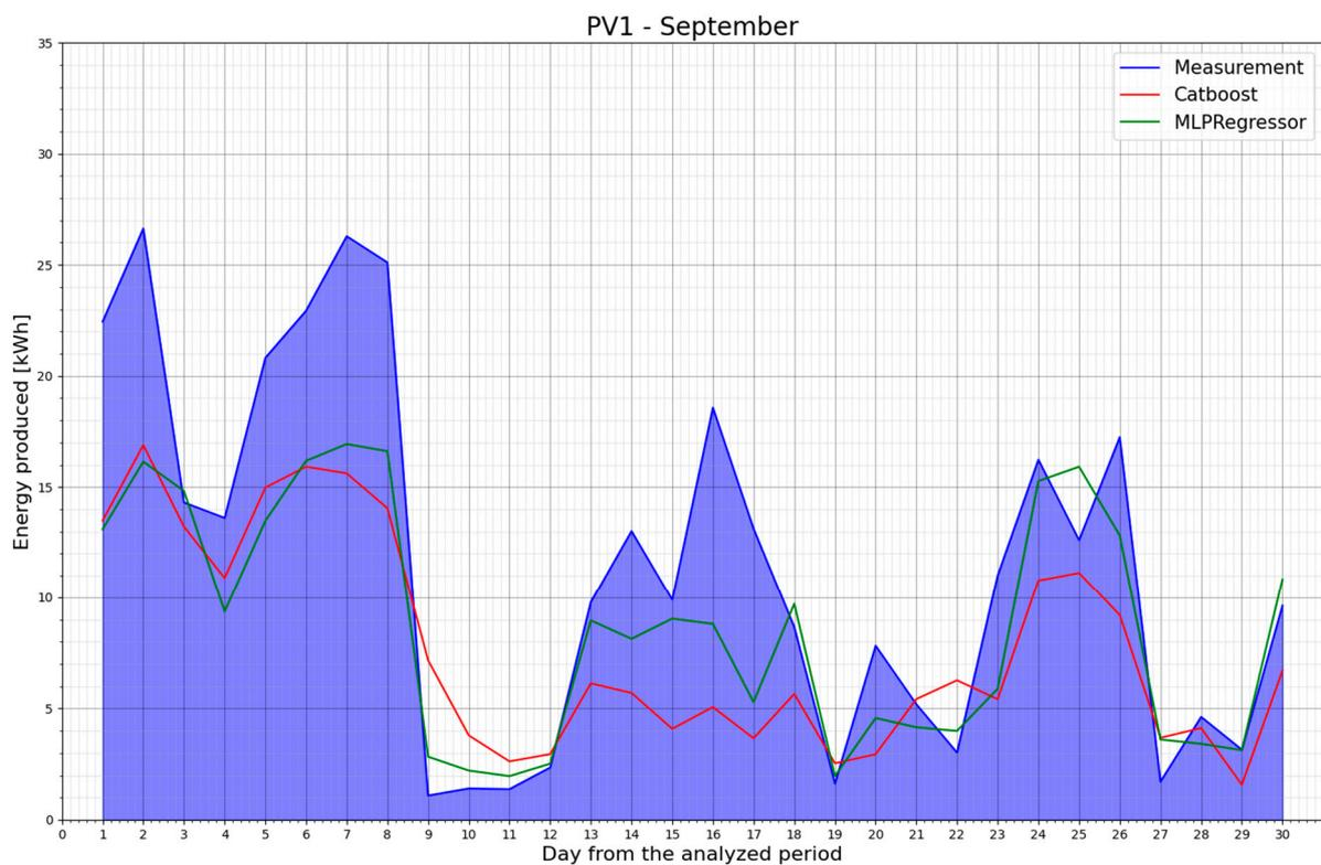
**Figure 10.** The energy produced in September 2022 and forecasts for the PV1 power plant using MLPRegressor and CatBoostRegressor models.
