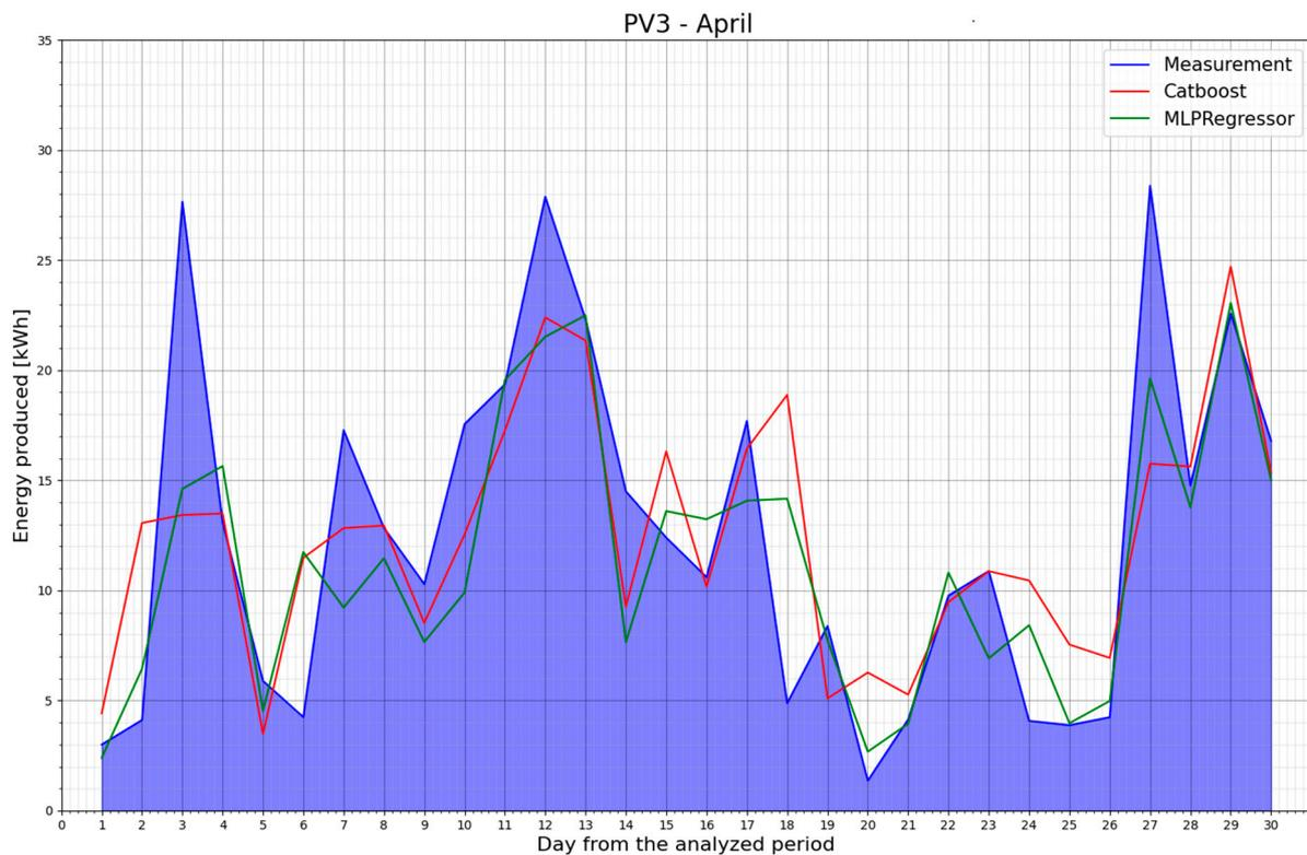
**Figure 11.** The energy produced in April 2022 and forecasts for the PV3 power plant using MLPRegressor and CatBoostRegressor models.
