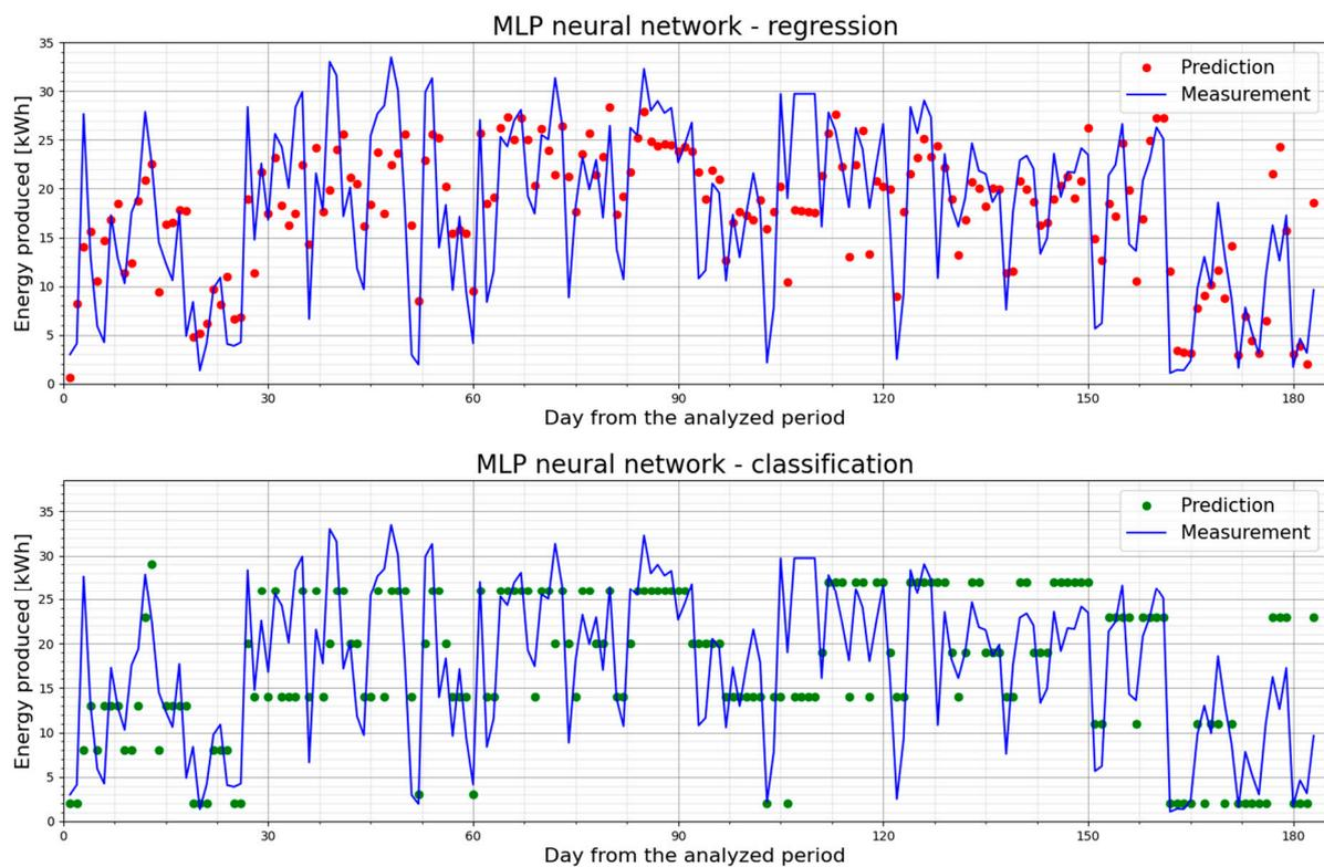
**Figure 6.** The energy produced in each day of the analyzed period and forecasts for the PV3 power plant using the MLPRegressor model and MLPClassifier model (with a discretization width of 1 kWh).
