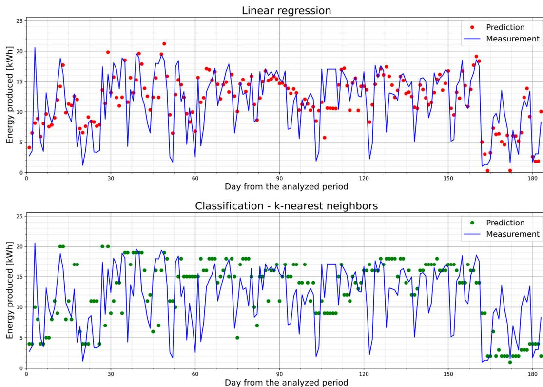
**Figure 3.** The energy produced in each day of the analyzed period and forecasts for the PV1 power plant using the linear regression model for  $m = 2$  and the KNN model for  $k = 12$  and  $weights = 'uniform'$ ; the width of discretization is 1 kWh.
