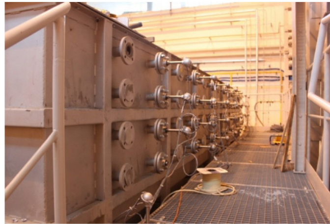
Figure 23. Placement of sensors on the side of the ex situ reactor [71]. Reproduced under CC BY 4.0.
