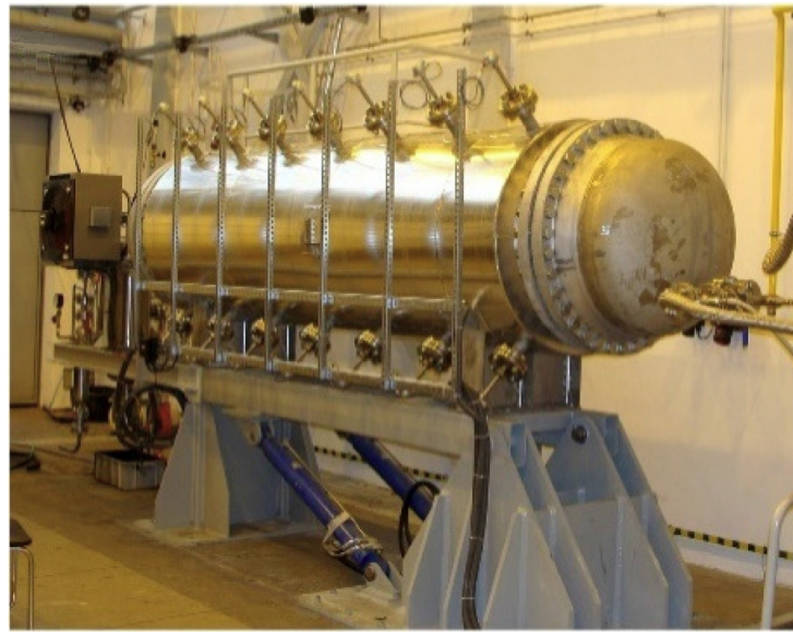
Figure 45. Reactor prepared for gasification [113]. Reproduced under CC BY 4.0.
