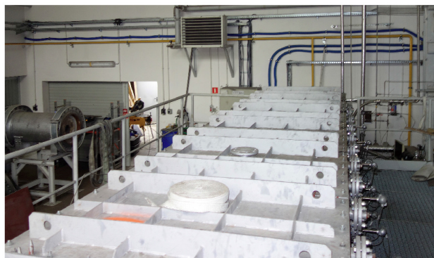
Figure 48. Ex situ reactor prepared for atmospheric pressure coal gasification [88]. Reproduced under CC BY 4.0.
