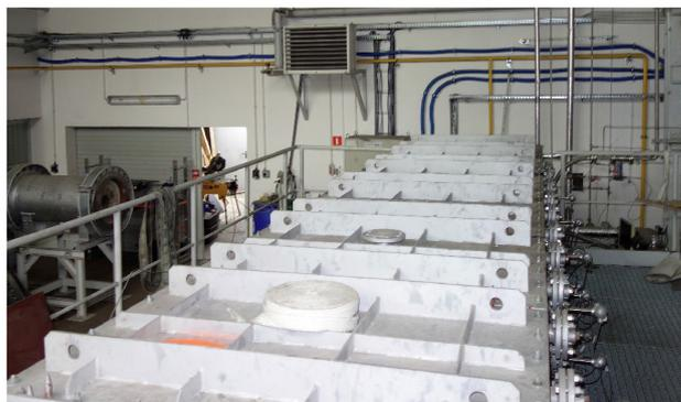
**Figure 48.** Ex situ reactor prepared for atmospheric pressure coal gasification [88]. Reproduced under CC BY 4.0.
