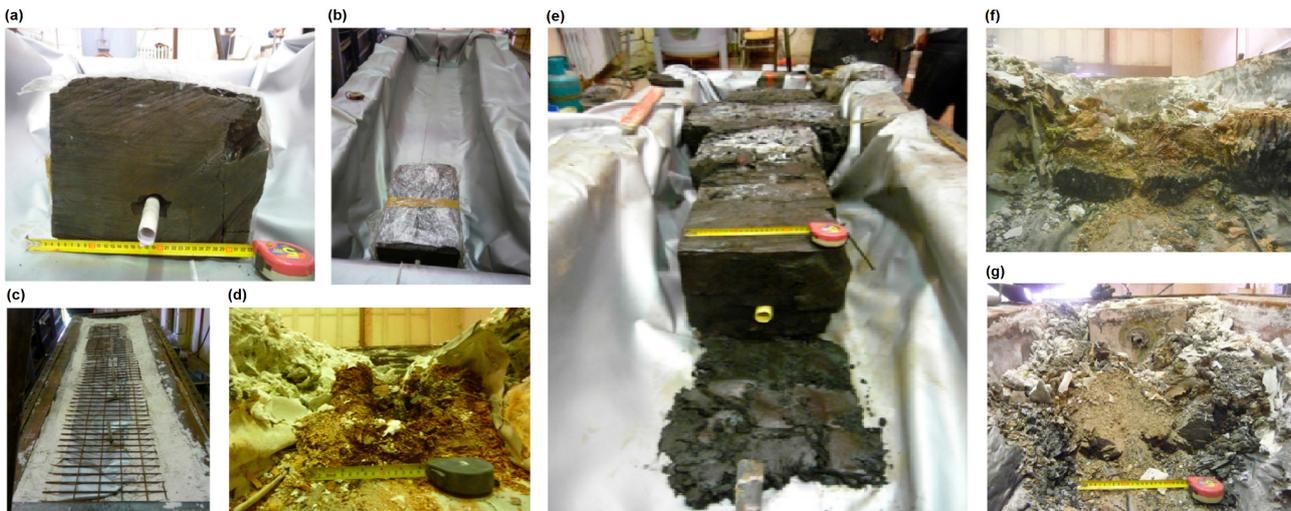
**Figure 36.** Model preparation in ex situ reactor for experiment #1: (a) gasification channel preparation; (b) coal block bedding; (c) metal grid installation; (d) result of gasification. Model preparation for experiment #2: (e) coal block bedding and gasification channel preparation; (f) a layer of coal in the second meter that remained unburned; (g) a layer of coal in the third meter that remained unburned [94]. Reproduced under [CC BY 4.0](#).
