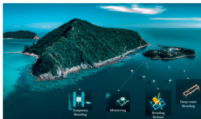
**Figure 1.** Schematic diagram of the Ocean Ranch equipment placement type and layout. According to the arrangement rules, the equipment can form a uniform layout or a linear layout. The equipment type mainly includes the following four types: Temporary Breeding, Monitoring, Breeding Release, and Deep-Water Breeding. All the above equipment can be intelligent equipment or traditional non-intelligent equipment.
