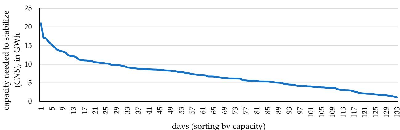
**Figure 8.** Capacity needed to stabilize electricity production (by capacity) sorted by day in Poland, 1 January 2023–14 May 2023. Source: own study.
