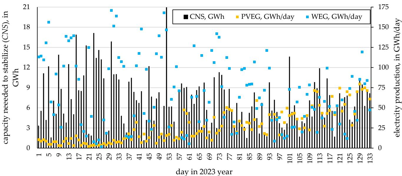
**Figure 7.** Capacity needed to stabilize electricity production in 2023 as well as photovoltaic energy, PVEG, and wind turbine energy, WEG, in Poland, 1 January 2023—14 May 2023. Source: own study.
