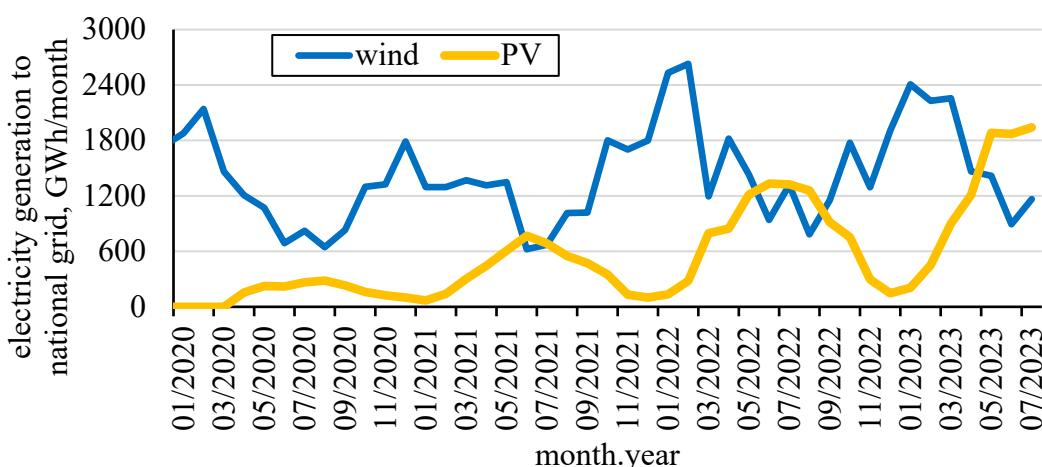
**Figure 1.** Monthly electricity production from wind turbines and photovoltaics in Poland 2020–April 2023. Source: own study based on [22].
