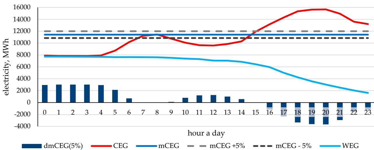
**Figure 5.** Average daily hourly values and hourly values of electricity production from coal (CEG) and wind (WEG) sources (GWh per h); deviations in production values from the average daily value with an acceptable deviation of 5% ( $dmCEG(5\%)$ ). Data for the day with the highest storage capacity requirement, corresponding to the most unfavorable conditions. Poland, 21 February 2023. Source: own study.
