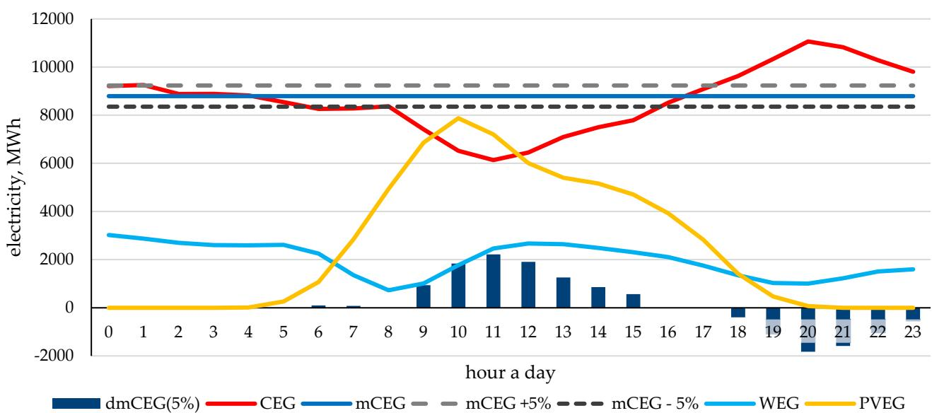
**Figure 6.** Average daily hourly values and hourly values of electricity production from coal (CEG), wind (WEG), and photovoltaic (PVEG) sources (GWh per h); deviations in production values from the average daily value with an acceptable deviation of 5% ( $dmCEG(5\%)$ ). Data for a day with a high value of PV energy production (61 GWh/day). Poland, 13/05/2023. Source: own study.
