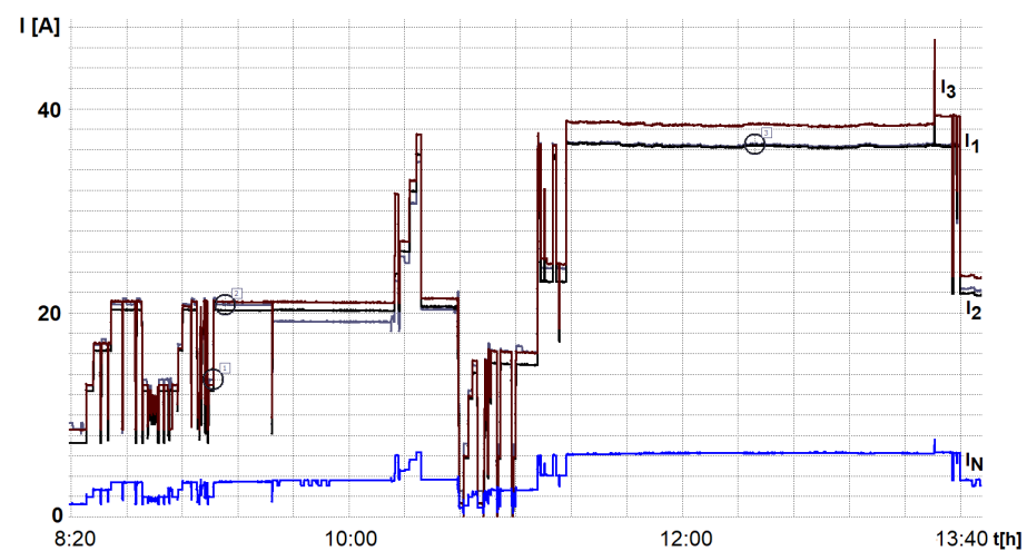
Figure 10. Values of currents in phase conductors and neutral conductor measured in an installation with LED luminaires with control. Source: authors' own study.
