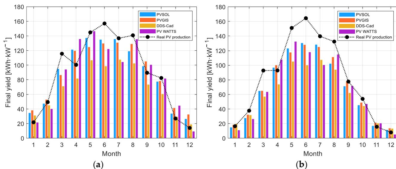
**Figure 5.** The measured and simulated values of monthly final yield of (a) PV3 system; and (b) PV4 system.
