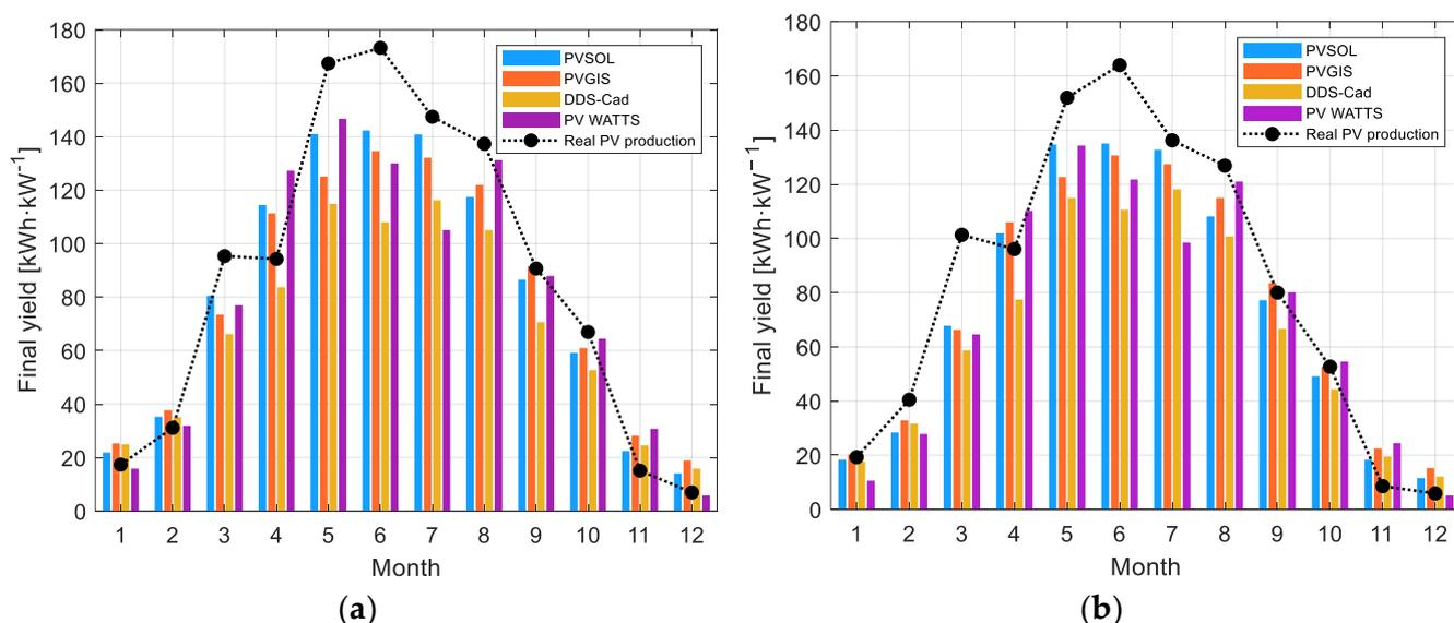
**Figure 4.** The measured and simulated values of the monthly final yield of the (a) PV1 system; and (b) PV2 system.
