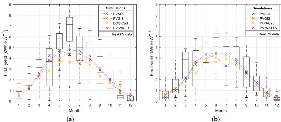
**Figure 6.** The measured and average simulated values of daily final yields of (a) PV1 system; and (b) PV2 system.
