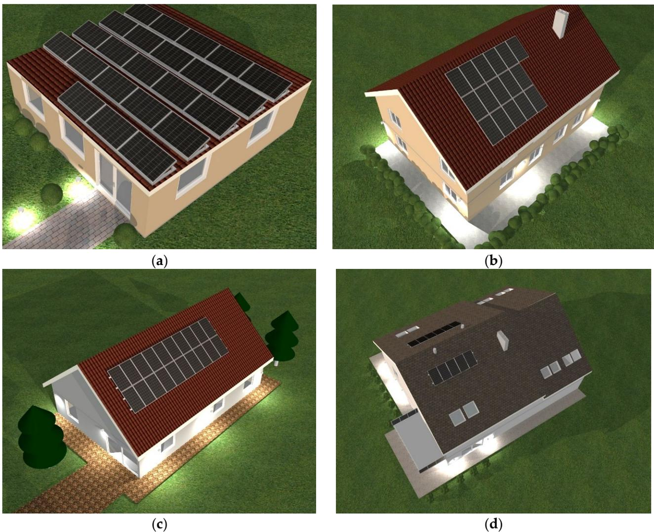
**Figure 2.** Visualization made with the use of DDS-Cad software of (a) PV1 system; (b) PV2 system; (c) PV3 system; and (d) PV4 system.
