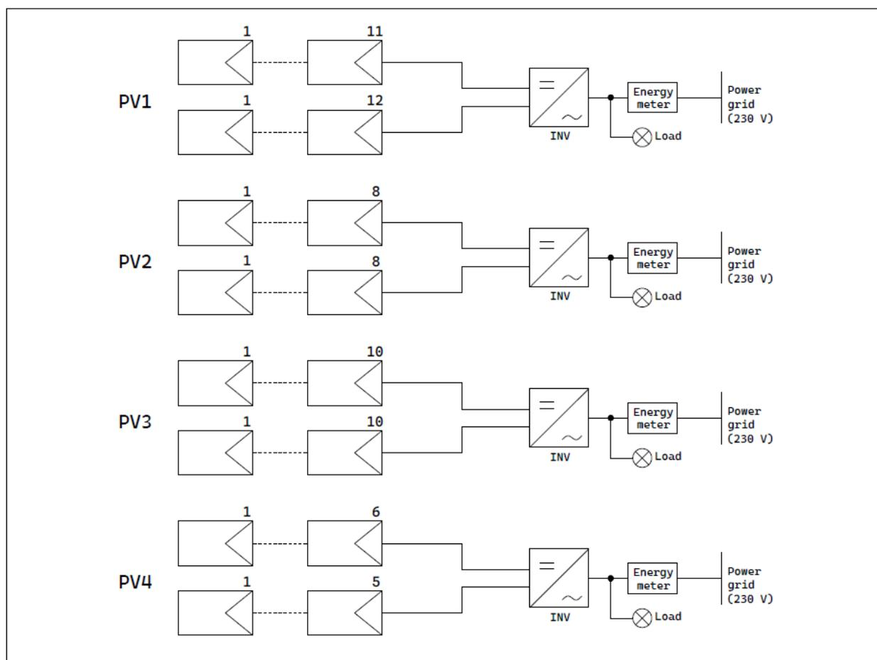
**Figure A1.** Schematic diagram of analyzed PV1–PV4 systems.
