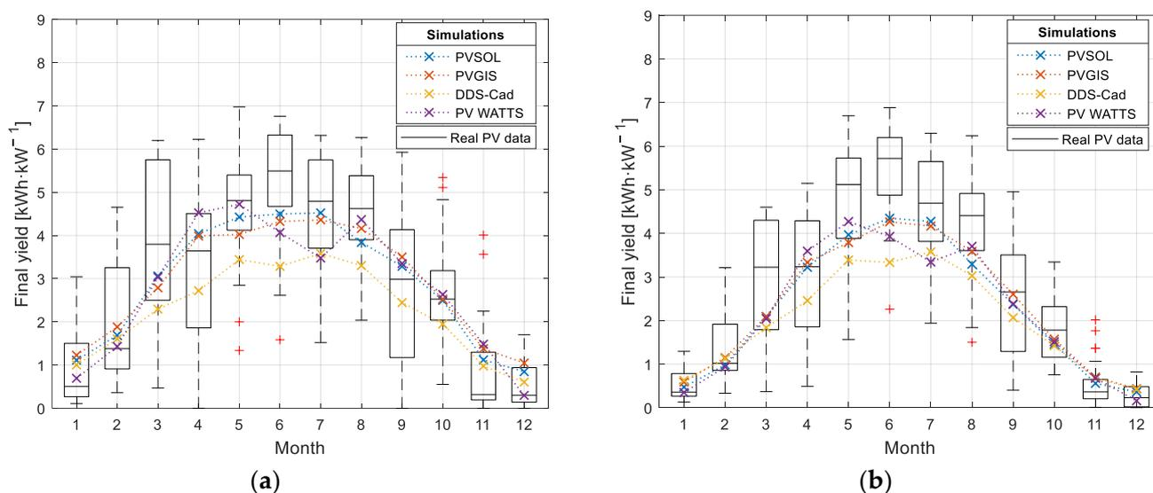
**Figure 7.** The measured and average simulated values of daily final yields of (a) PV3 system; and (b) PV4 system.
