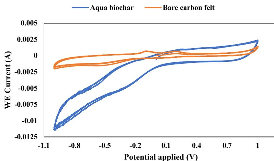
**Figure 5.** CV plots of aquacultural biochar catalyst coated carbon felt and bare carbon felt electrode without any catalyst.
