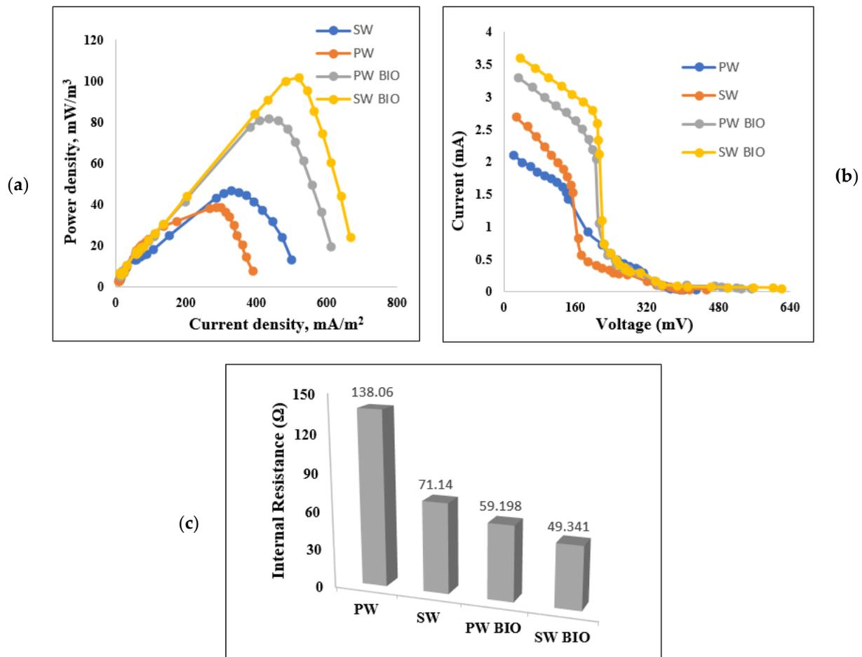
**Figure 10.** Polarization plots: (a) Power density vs. current density curve, (b) voltage vs. current curve, and (c) internal resistance value ranges.
