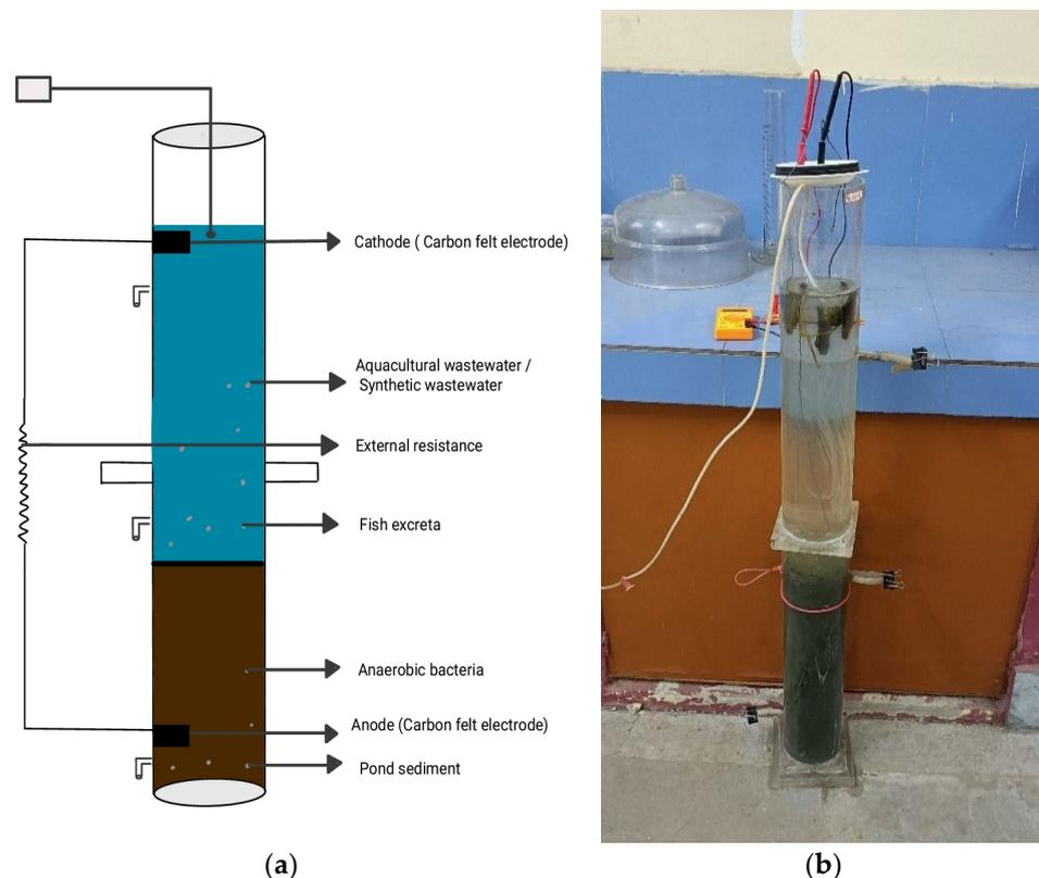
**Figure 3.** (a) Theoretical explanation of SMFC; (b) Experimental SMFC reactor.
