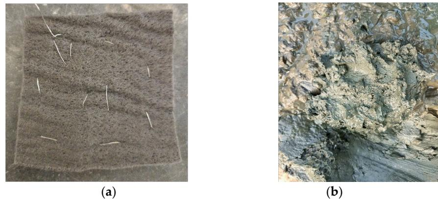
**Figure 2.** (a) Carbon felt electrode; (b) Pond sediment.
