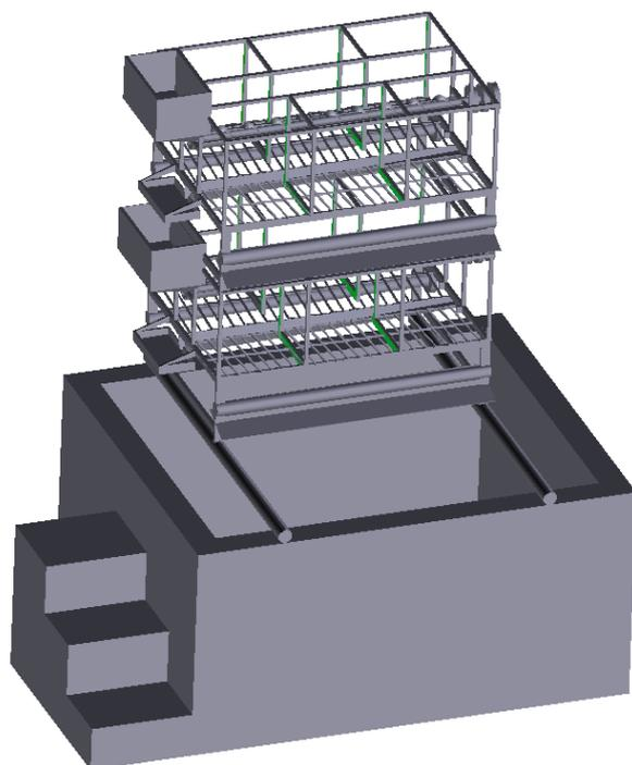
**Figure 11.** Design drawing of SMFC-assisted wastewater treatment for an integrated poultry–fish culture system.
