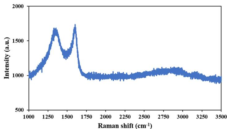
Figure 8. Raman spectroscopy plot for activated aquacultural biochar catalyst.
