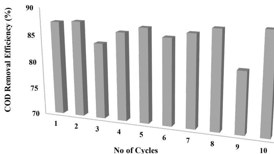
**Figure 9.** Stable COD removal efficiency range of wastewater to effluent over the 10 experimental cycles.
