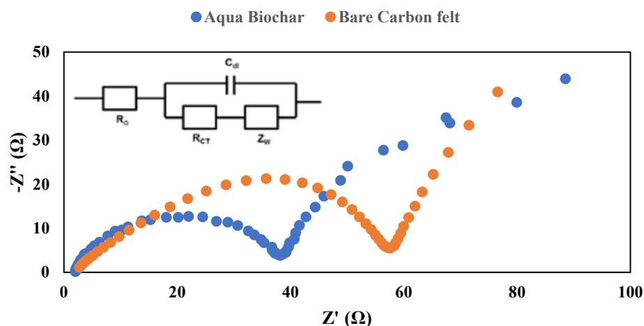
**Figure 6.** EIS plots of aquacultural biochar catalyst coated carbon felt and bare carbon felt along with its Randles circuit with Warburg element.
