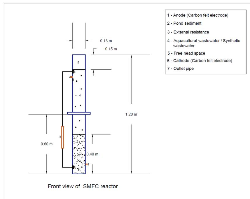
**Figure 1.** CAD design of SMFC reactor.
