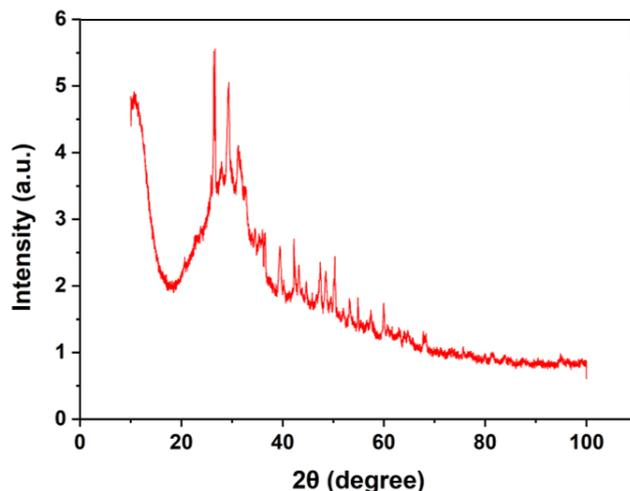
Figure 7. XRD plot for activated aquacultural biochar catalyst.
