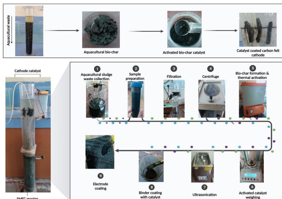
**Figure 4.** Process flowchart of preparation of cathode catalyst from aquacultural wastes for performance improvement of SMFC reactor.
