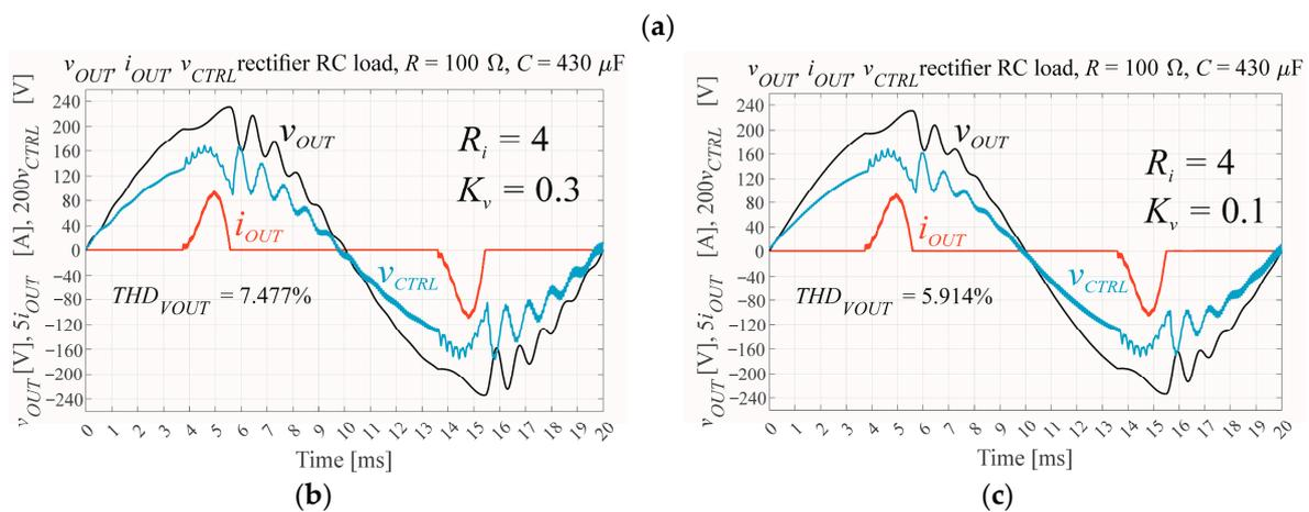
**Figure 10.** (a) The inverter model with  $2T_s$  delays in the measuring traces with the PBC controller without the prediction; (b) the output voltage waveform for the boundary PBC gains; and (c) the output voltage waveform for the decreased PBC gains adjusted to obtain the minimum distortions for  $f_s = 12,800$  Hz.
