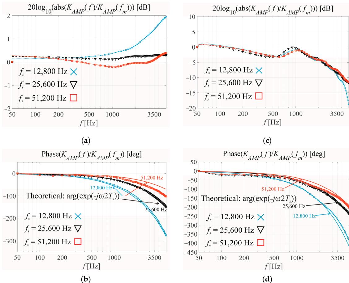
**Figure 6.** Two exemplary Bode plots: (a,c) magnitude, and (b,d) phase of two experimental inverters, (a,b) the first and (c,d) the second one.
