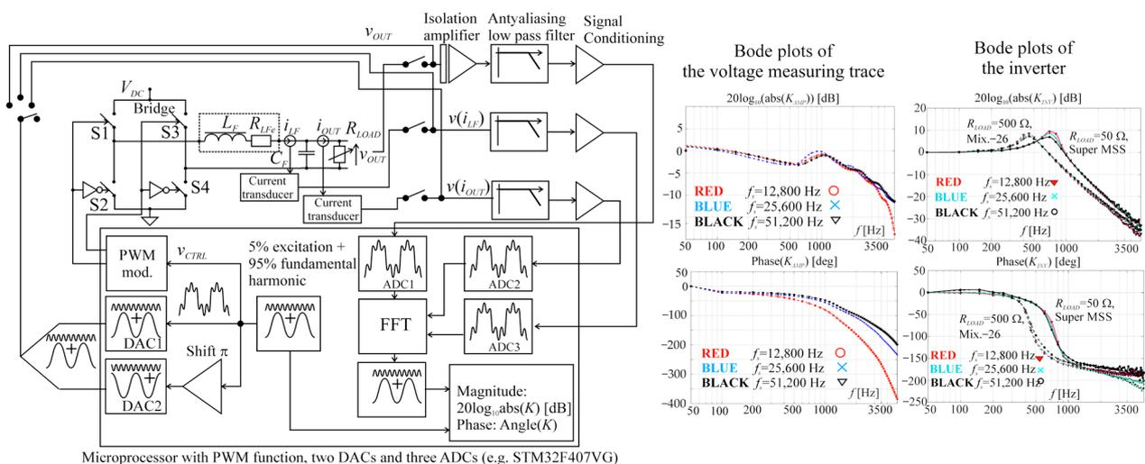
Figure 4. Measurement of the Bode plots of the inverter and the measuring voltage trace.
