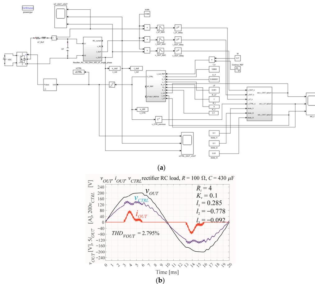
**Figure 11.** (a) The inverter model with  $2T_s$  delays in the measuring traces and PBC with the Luenberger observer; and (b) the output voltage waveform for the PBC and observer gains adjusted to obtain the minimum distortions for  $f_s = 12,800$  Hz.
