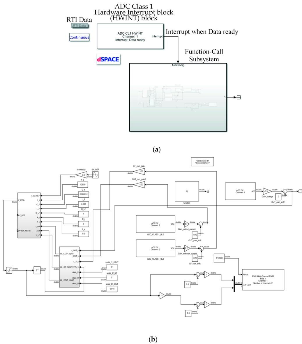
**Figure 13.** The schema of the control using SIMULINK and dSpace, (a) the block diagram of control with the function-call subsystem; (b) the inside of the function-call subsystem.
