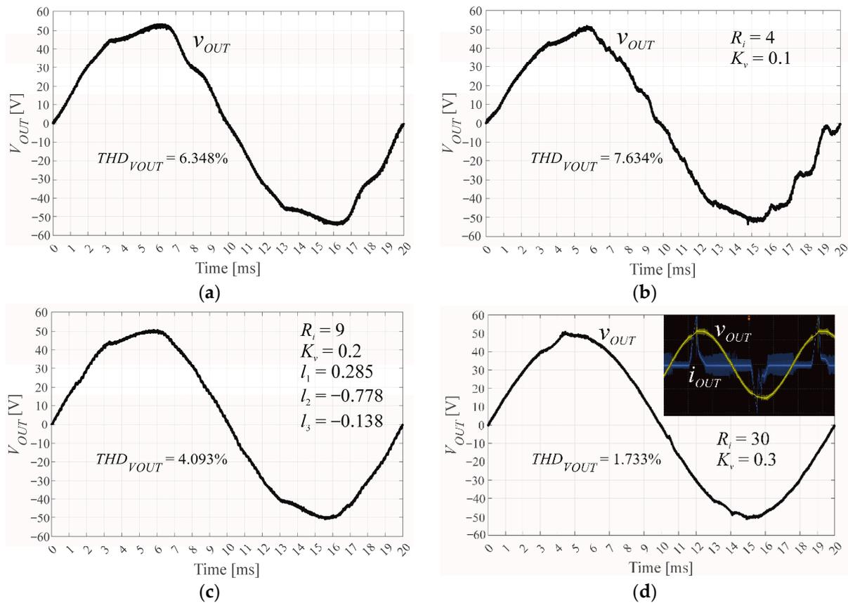
**Figure 14.** The output voltage waveforms: (a)  $f_s = 12,800$  Hz, no feedback; (b)  $f_s = 12,800$  Hz, PBC, no prediction; (c)  $f_s = 12,800$  Hz, PBC with Luenberger observer; (d)  $f_s = 51,200$  Hz, PBC, no prediction.
