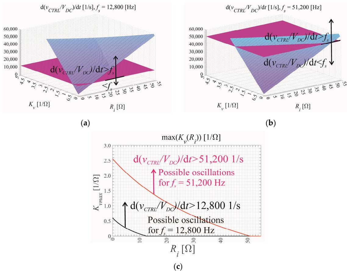
**Figure 7.** The limits of the voltage and current gains for two switching frequencies  $f_s = 12,800$  (a) and  $f_s = 51,200$  Hz (b) for  $L_F = 1$  mH,  $R_{LFe} = 1$  Ω,  $C_F = 51$  μF and gain border lines for two switching frequencies (c).
