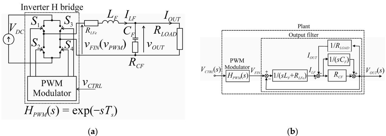
Figure 1. The continuous model: (a) inverter model and (b) block diagram.
