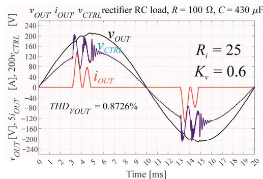
**Figure 12.** The output voltage waveform for the PBC (without the prediction) gains adjusted to obtain the minimum distortions for  $f_s = 51,200$  Hz.
