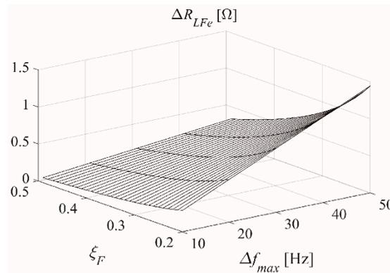
**Figure 5.** The error  $\Delta R_{LFe}$  of measurement of the serial equivalent resistance  $R_{LFe}$  as a function of damping coefficient  $\xi_F$  and frequency resolution  $\Delta f_{max}$  (for  $L_F = 1$  mH,  $C_F = 51$   $\mu$ F).
