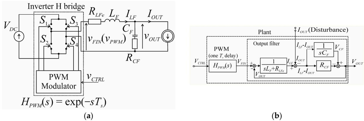
**Figure 2.** The simple continuous model with  $I_{OUT}$  as a disturbance: (a) inverter model and (b) block diagram for modelling the load current as an independent disturbance.
