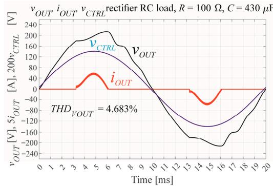
Figure 8. The inverter output voltage, output current waveforms for the open loop and the nonlinear rectifier load  $R = 100 \Omega$  and  $C = 430 \mu F$ .
