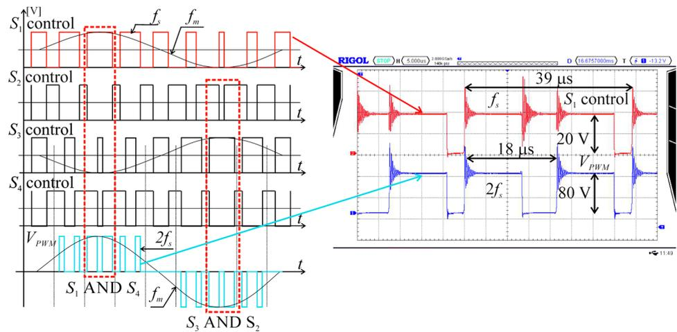
**Figure 3.** The first schema of the double–edge, 3–level PWM.
