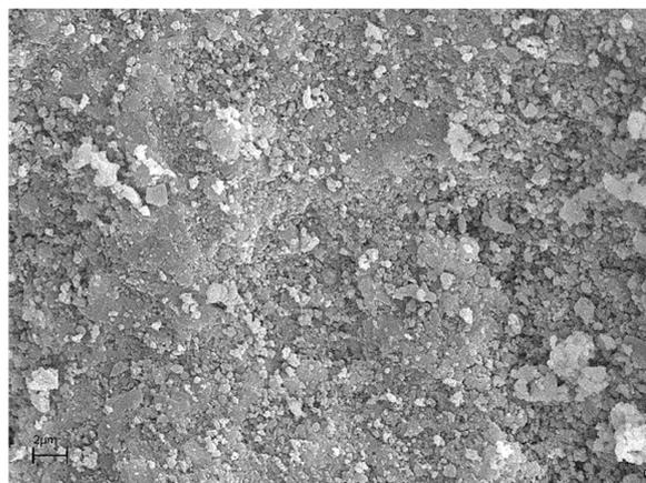
**Figure 8.** SEM photograph of CFBC-S (magn.:  $\times 20,000$ , scale bar: 2  $\mu\text{m}$ ).
