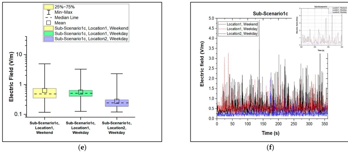
**Figure 2.** Boxplot charts and time variation of electric field for Scenario 1 (voice call) of the electric field measured in each sub-scenario at two locations (Location 1 and Location 2) for weekdays and weekends: (a,b) Sub-Scenario 1a: voice call set up via GSM network; (c,d) Sub-Scenario 1b: voice call set up via UMTS network; and (e,f) Sub-Scenario 1c: voice call set up via 5G/LTE/3G/2G (auto connect) network.
