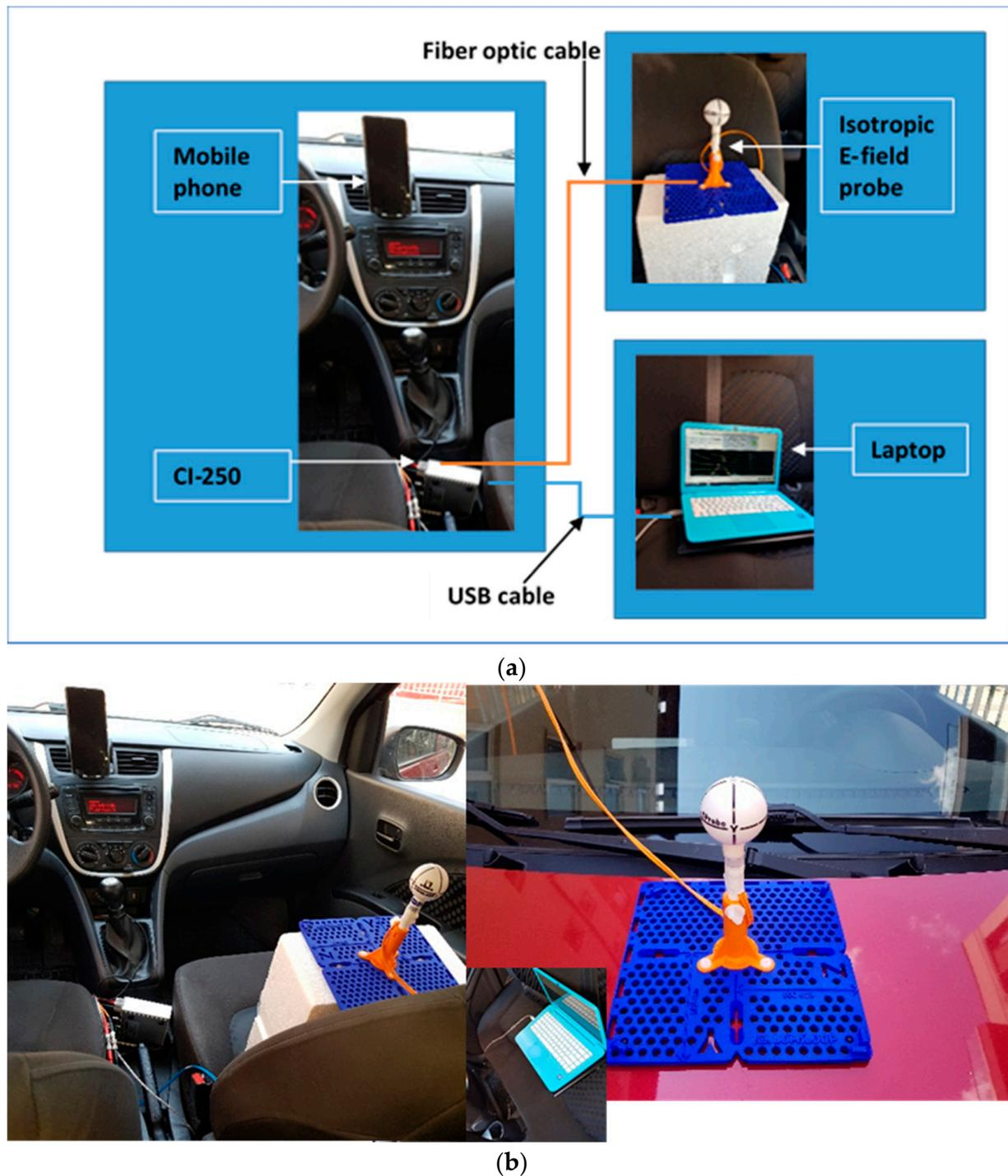
Figure 1. Overview of the experimental setup: (a) block diagram and (b) photos.
