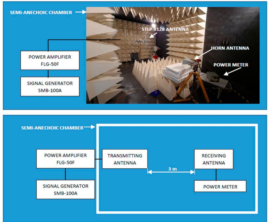
Figure 8. Measurement setup: photo and block diagram.
