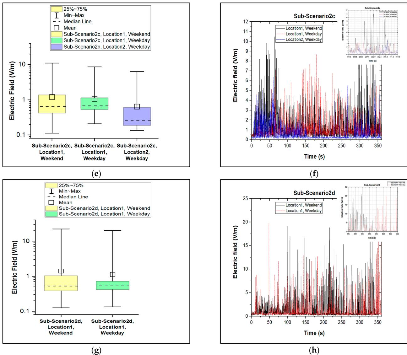
**Figure 3.** Boxplot charts and time variation of electric field for Scenario 2 (video call) of the electric field measured in each sub-scenario at two locations (Location 1 and Location 2) for weekdays and weekends: (a,b) Sub-Scenario 2a: video call set up via GSM network; (c,d) Sub-Scenario 2b: video call set up via UMTS network; (e,f) Sub-Scenario 2c: video call set up via LTE network; and (g,h) Sub-Scenario 2d: video call set up via 5G network.
