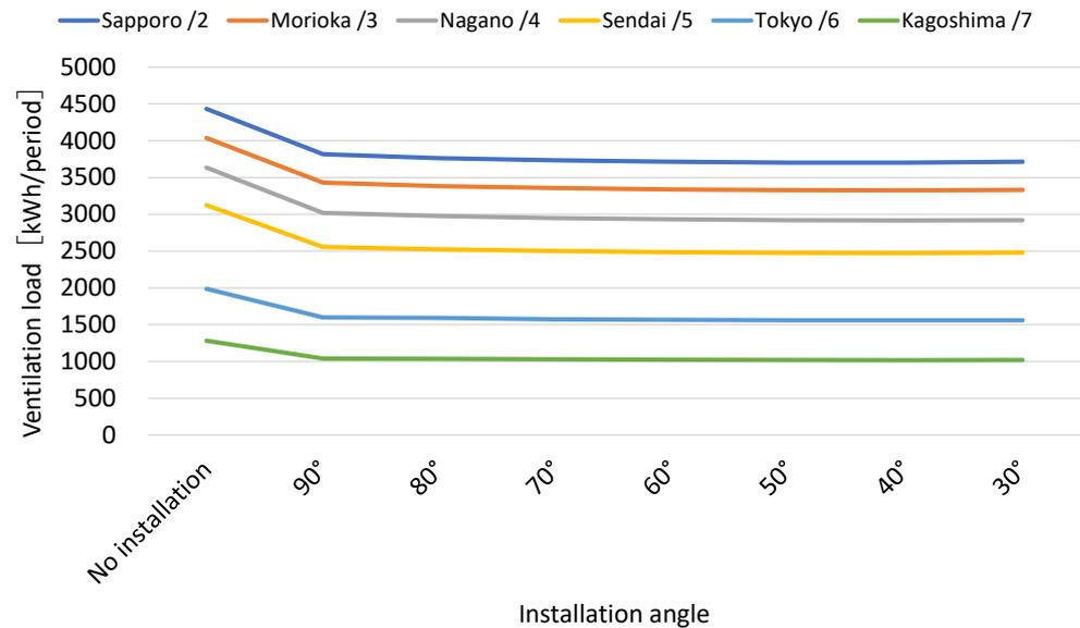
**Figure 6.** Ventilation load during the heating period by the angle of SAH installation by zone.
