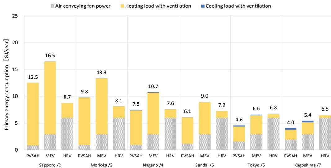
Figure 11. Annual primary energy consumption of a heat pump.
