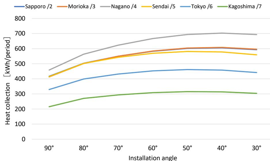
Figure 4. Comparison of heat collection by the angle of SAH installation by zone.
