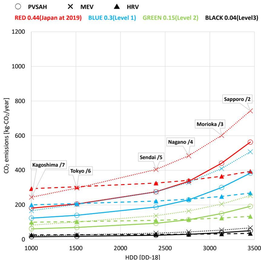
Figure 13. Annual CO<sub>2</sub> emissions of a heat pump.
