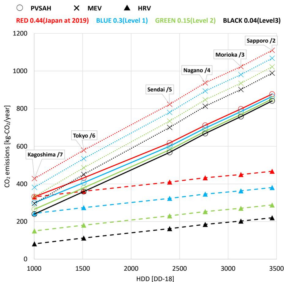
Figure 14. Annual CO<sub>2</sub> emissions of a gas boiler.
