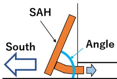
Figure 5. Installation angle of SAH.
