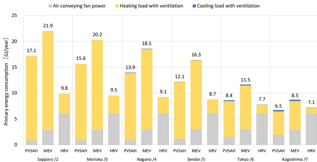
Figure 12. Annual primary energy consumption of a gas boiler.
