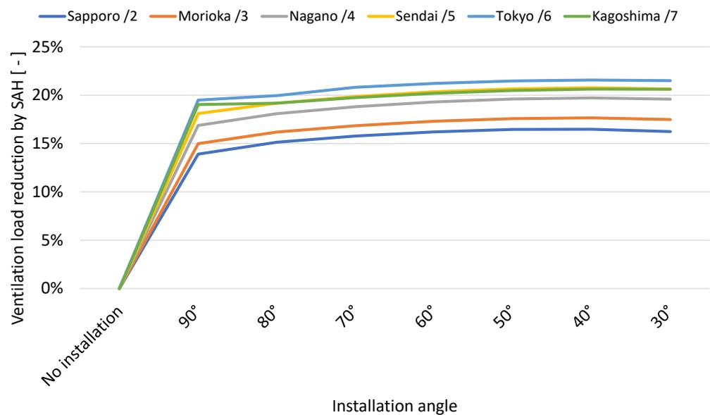
**Figure 7.** Reduction of ventilation load during the heating period by SAH by zone.
