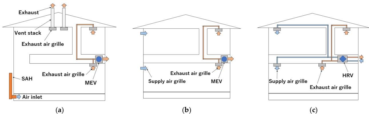
**Figure 3.** Overview of the system diagram. (a) PVSAH, (b) MEV, and (c) HRV.
