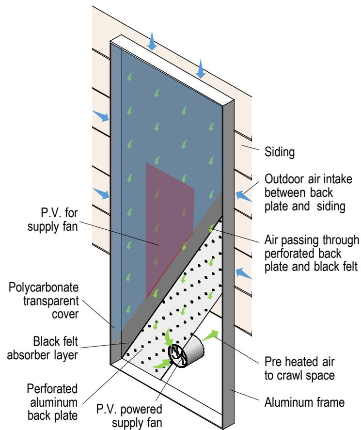
Figure 2. Overview of the solar air heater (SAH) [18].
