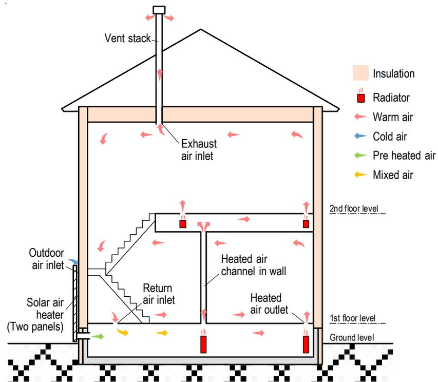
Figure 1. Overview of the passive ventilation system with a solar air heater (PVSAH) [18].
