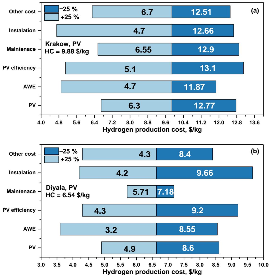
**Figure 12.** Sensitivity analysis of the hydrogen production cost using a 3MW solar photovoltaic power plant for: (a) Krakow and (b) Diyala.
