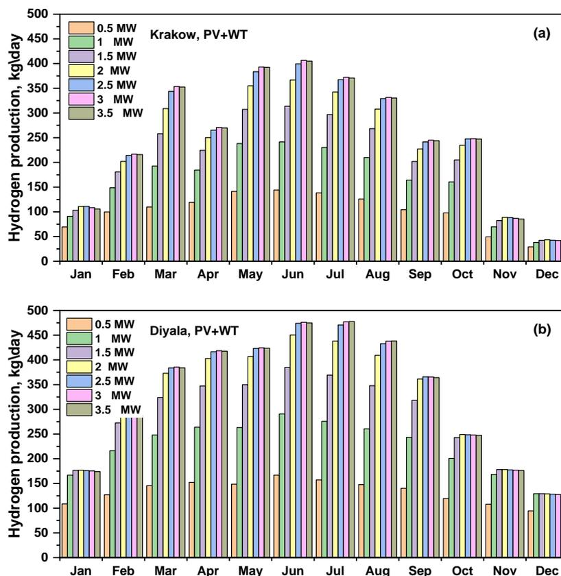
**Figure 11.** Hybrid system annual production of green hydrogen at different AWE capacities for: (a) Krakow and (b) Diyala.
