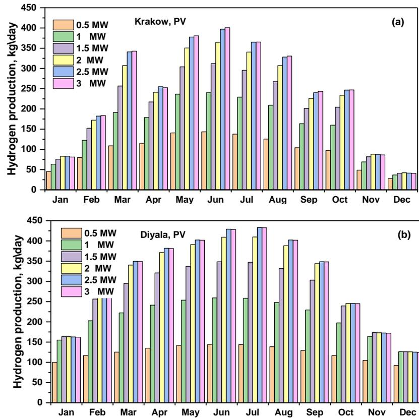
Figure 9. Monthly production of green hydrogen using photovoltaic energy based on a variety of AWE capacities for: (a) Krakow and (b) Diyala.
