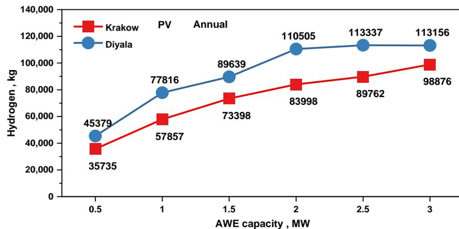
Figure 10. Annual production of green hydrogen based on photovoltaic energy at several AWE capacities for Krakow and Diyala.
