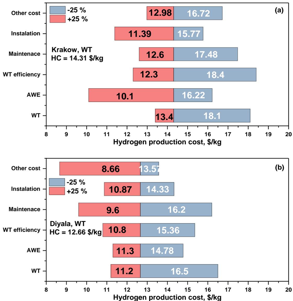
**Figure 13.** Sensitivity analysis of the hydrogen production cost using a 3.0 MW solar WT power plant in: (a) Krakow and (b) Diyala.
