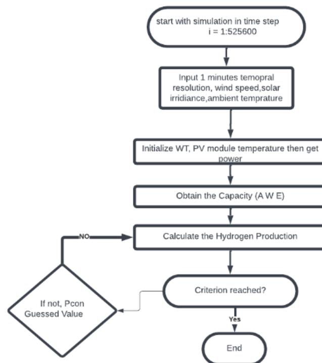
Figure 5. The simulation steps for the proposed system.
