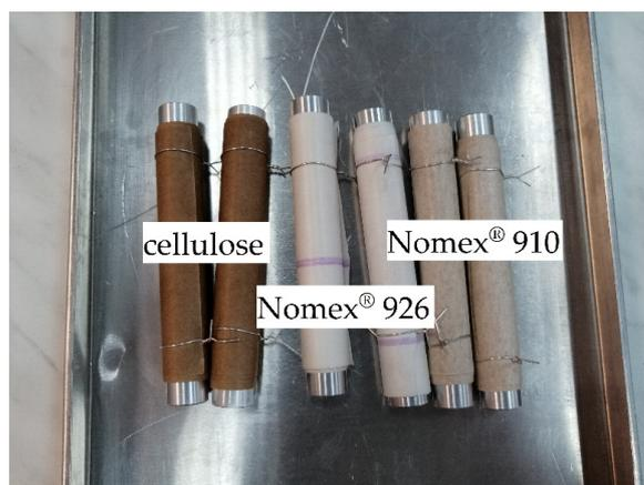
**Figure 3.** Tested insulation materials wound on patrons.
