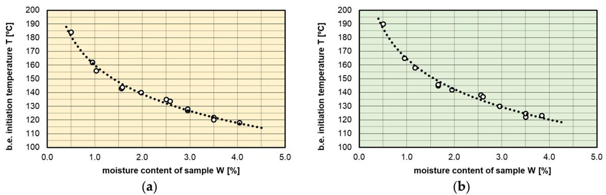
**Figure 8.** Measurement results of the bubble effect initiation temperature for Nomex<sup>®</sup> 926 paper immersed in mineral oil Orlen Trafo EN (a) and synthetic ester Midel 7131 (b).
