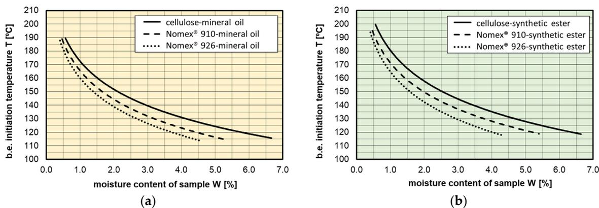
**Figure 10.** Comparison of the bubble effect initiation temperature for cellulose (solid line), Nomex<sup>®</sup> 910 (dashed line) and Nomex<sup>®</sup> 926 (dotted line) immersed in mineral oil Orlen Trafo EN (a) and synthetic ester Midel 7131 (b).
