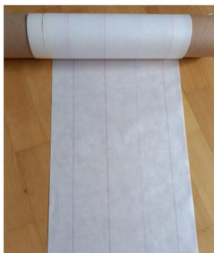
**Figure 1.** A photograph of the Nomex<sup>®</sup> 926 used in the experiment.
