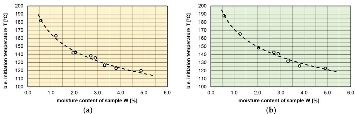
**Figure 7.** Measurement results of the bubble effect initiation temperature for Nomex<sup>®</sup> 910 paper immersed in mineral oil Orlen Trafo EN (a) and synthetic ester Midel 7131 (b).
