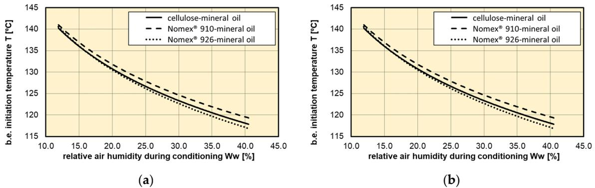
**Figure 11.** Comparison of the bubble effect initiation temperature depending on the relative air humidity in climate chamber during the conditioning of materials at a temperature of 40 °C for cellulose (solid line), Nomex<sup>®</sup> 910 (dashed line) and Nomex<sup>®</sup> 926 (dotted line) immersed in mineral oil Orlen Trafo EN (a) and synthetic ester Midel 7131 (b).
