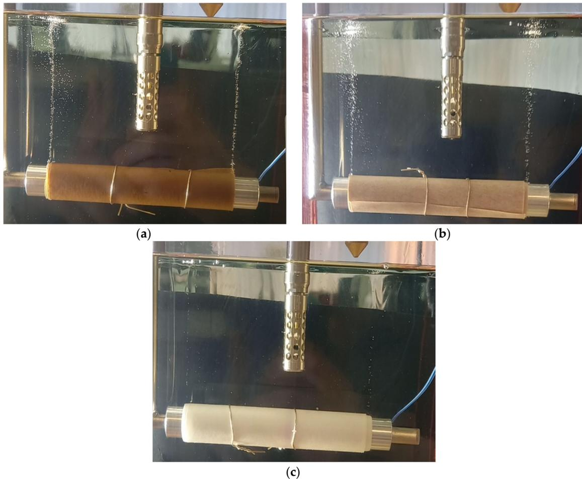
**Figure 12.** Intensity comparison of b.e. recorded for samples conditioned in air of the same relative humidity and at the same temperature. (a) Kraft cellulose paper, (b) Nomex<sup>®</sup> 910 and (c) Nomex<sup>®</sup> 926.
