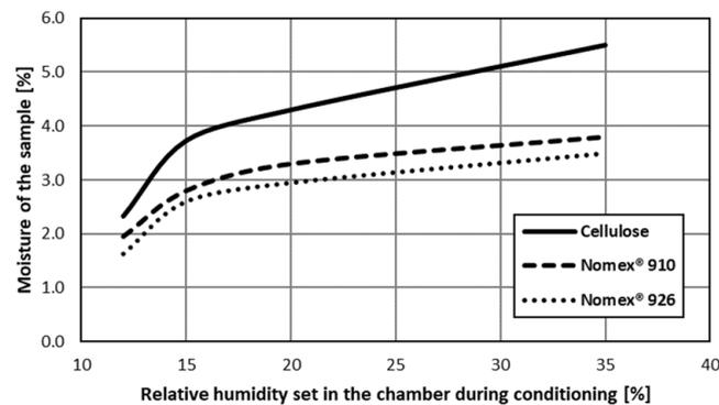
**Figure 4.** Moisture characteristics of the tested materials depending on the relative air humidity in the climatic chamber during conditioning at 40 °C.
