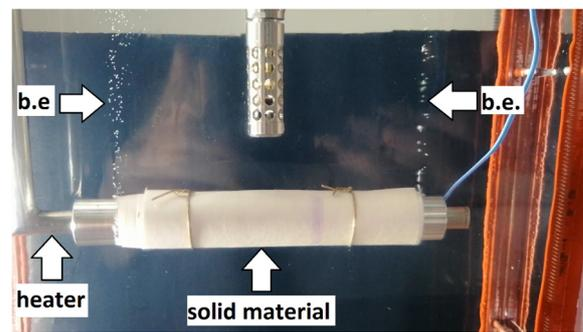
**Figure 5.** The sample of Nomex<sup>®</sup> 926 during the bubble effect test immersed in an insulating liquid.
