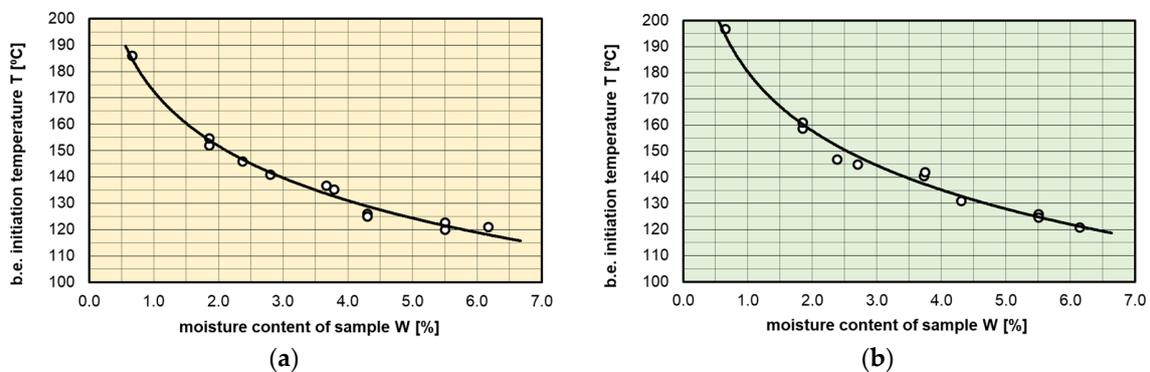
**Figure 6.** Measurement results of the bubble effect initiation temperature for cellulose paper immersed in mineral oil Orlen Trafo EN (a) and synthetic ester Midel 7131 (b).
