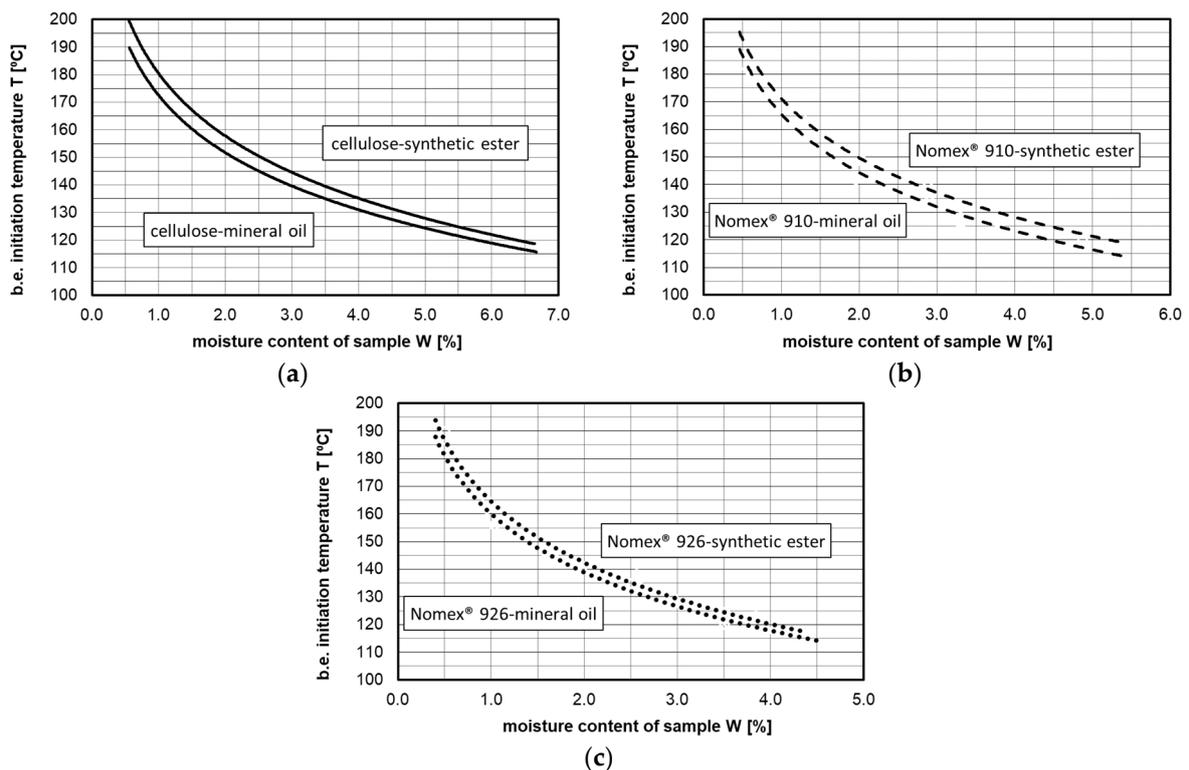
**Figure 9.** The influence of the insulating liquid (mineral oil Orlen Trafo EN, synthetic ester Midel 7131) on the bubble effect initiation temperature for different materials: Cellulose (a), Nomex<sup>®</sup> 910 (b) and Nomex<sup>®</sup> 926 (c).
