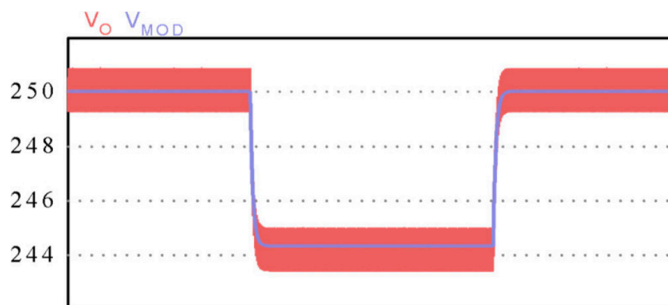
Figure 10. Dynamic responses of rectifier output voltage (red) and small-signal model (blue) for a step of 2% in duty cycle.
