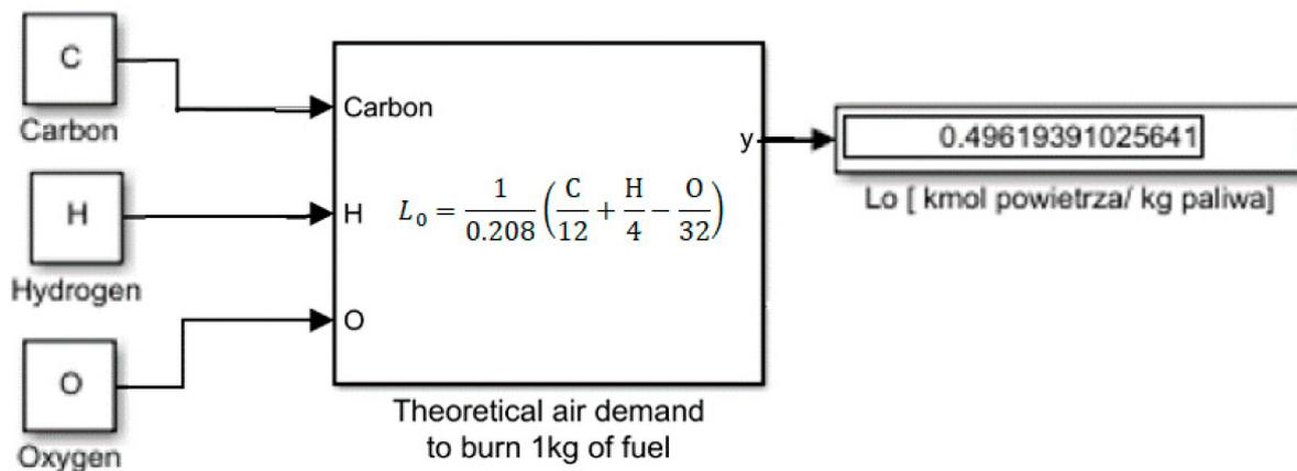
Figure 2. Diagram of the measuring system to determine the theoretical air demand to burn 1 kg of fuel.
