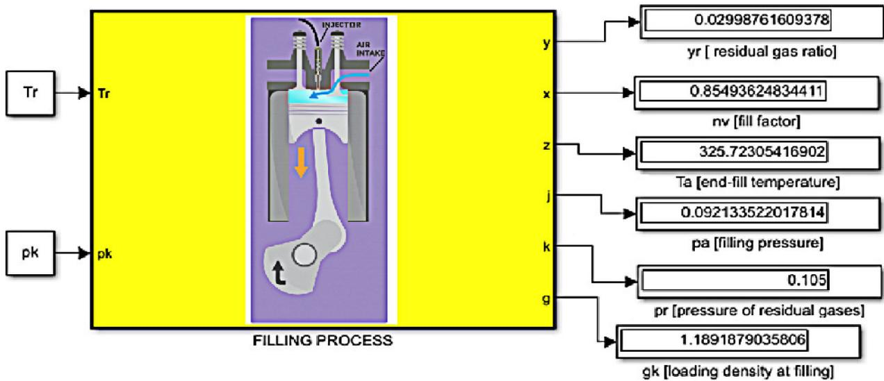
Figure 4. Diagram of the measuring system of the filling process.
