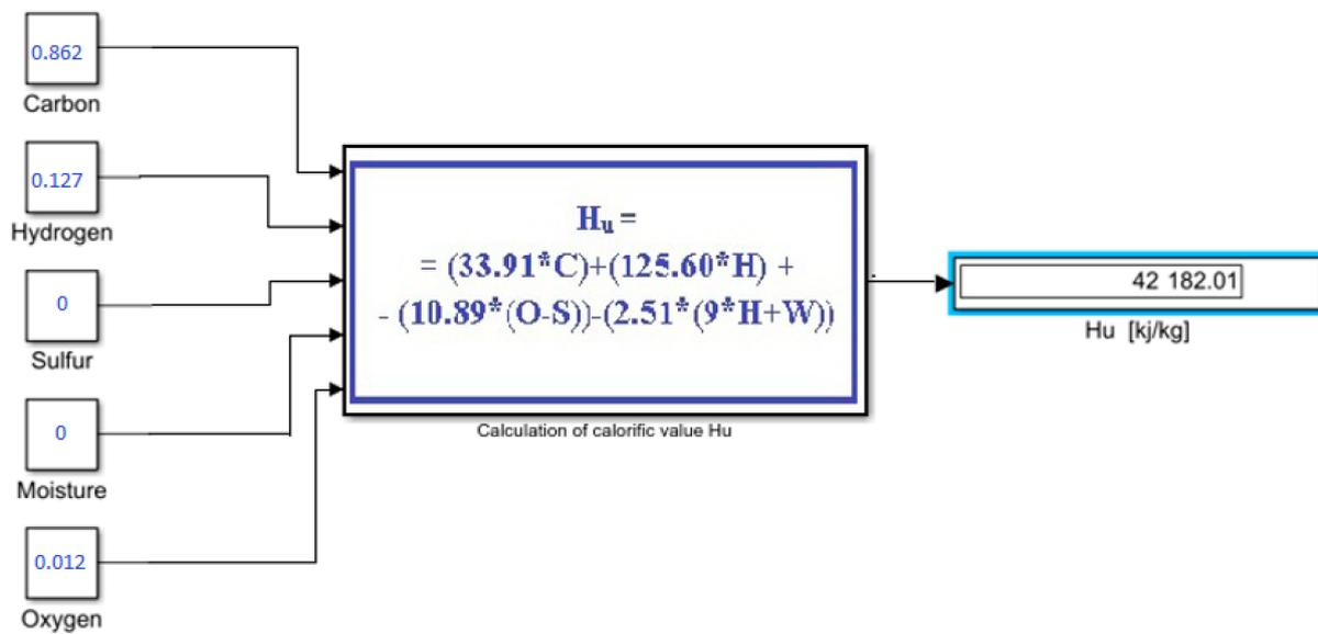
Figure 1. Diagram of the measuring system for determining the calorific value of the fuel.
