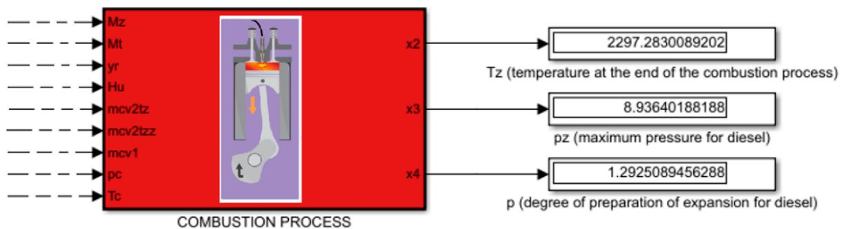
Figure 7. Diagram of the measuring system of the combustion process.
