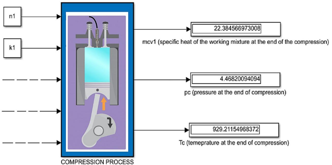
Figure 5. Diagram of the measuring system of the compression process.
