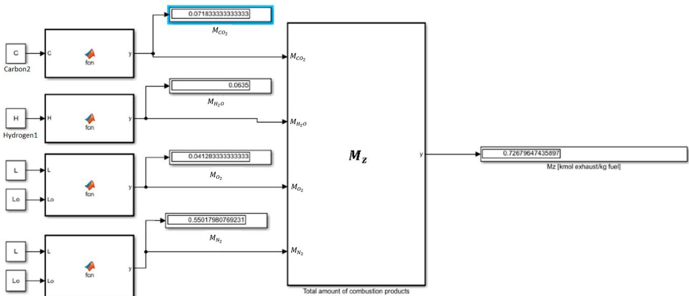
Figure 3. Diagram of the measuring system for determining total amount of combustion products.
